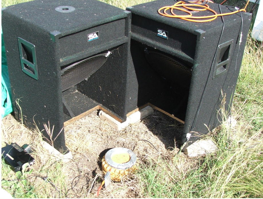
Figure 3.8: Photograph of subwoofers used for high-intensity insonification. Unburied mine is shown for reference.
