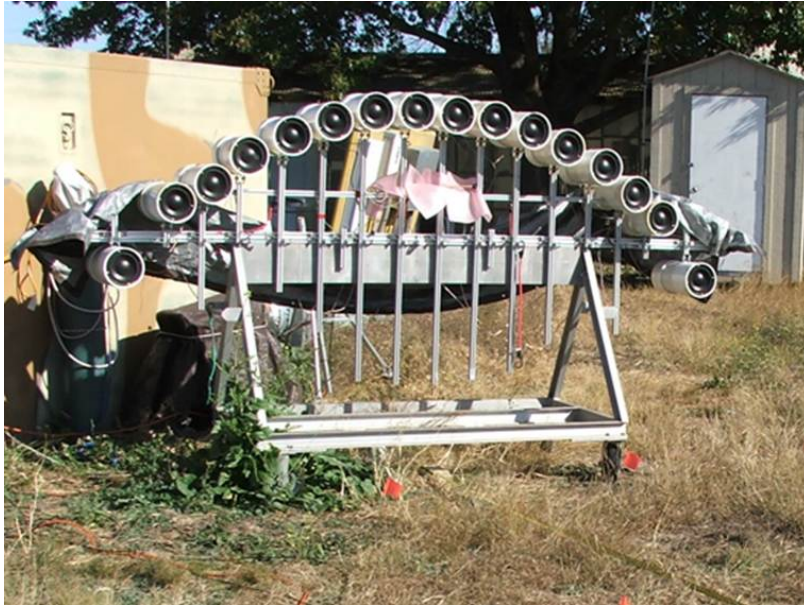
Figure 3.1: Sixteen-speaker array used for ground insonification. The radius of the array is 6 feet, and each speaker is separated horizontally from its neighbors by 8 inches.
