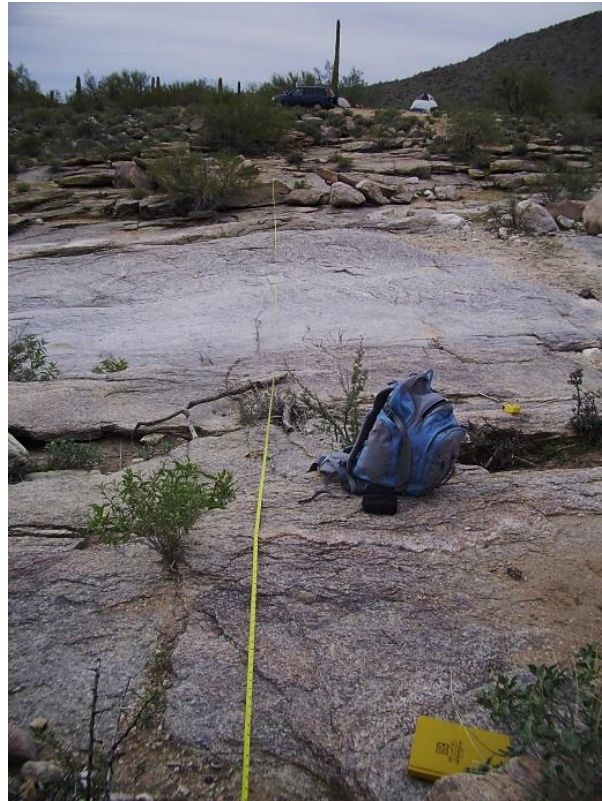
Figure 2.6: Photograph of the eastern transect line looking south. Measurements of shear zone thickness, shear zone orientations, and the spacing between shear zones were made for each shear zone intersecting the measuring tape.
