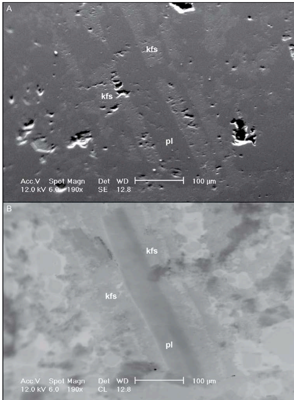
Figure 3.39: SE and CL images of a typical plagioclase feldspar phenocryst with potassium feldspar overgrowth rim. The interior plagioclase core may vary greatly in length, ranging from 20-120 µm. The overgrowth of potassium-rich feldspar suggests that the plagioclase formed first in the petrogenic sequence, and then conditions changed favoring potassium feldspar growth. Sample ORT266-02
