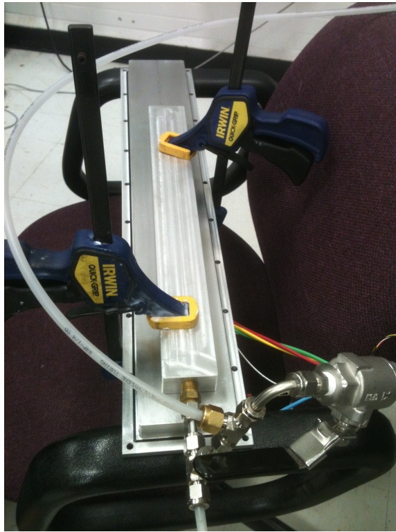
Figure 3.6: Kulite Pressure Transducer Calibration
