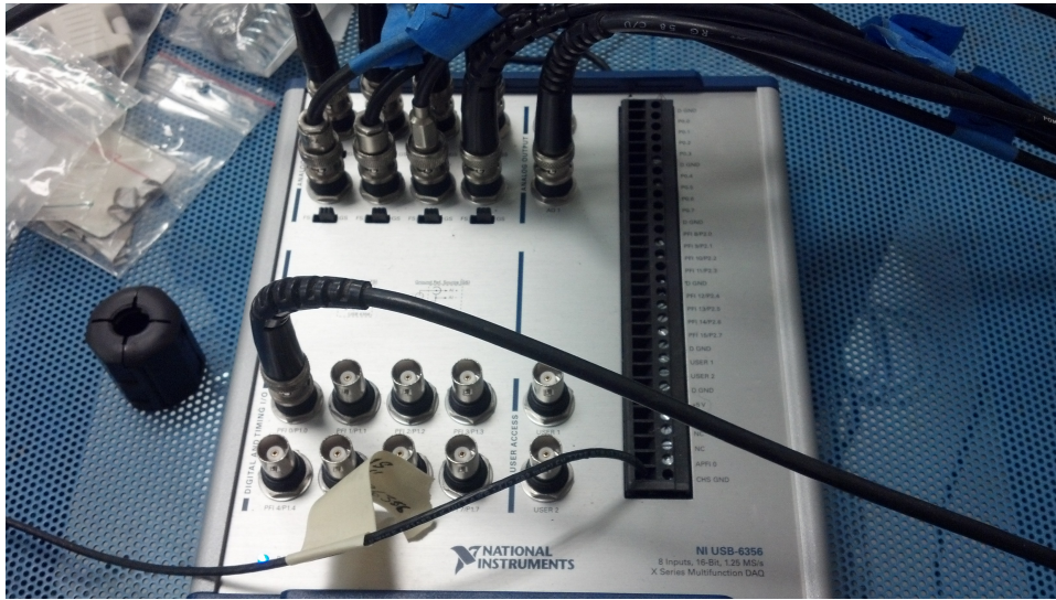
Figure 3.4: NI USB-6356 X-series Multifunction DAQ Device
