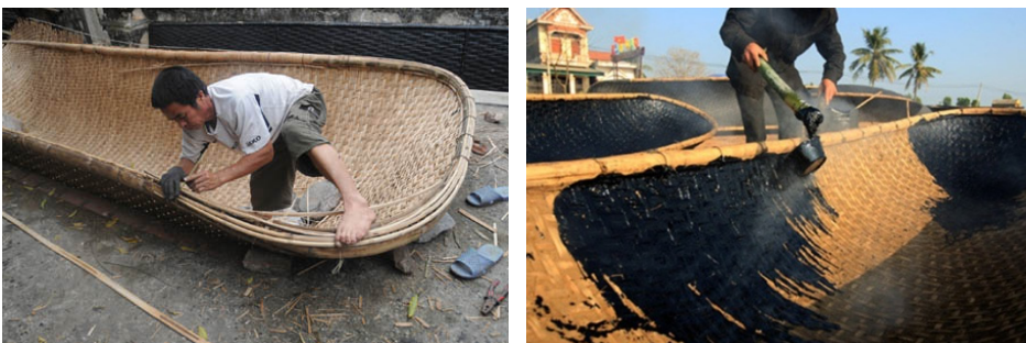
Fig V.1.b.7: Bamboo boat construction: hull weaving and water proofing
