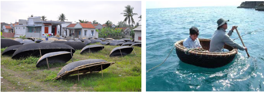
Fig V.1.b.6: Bamboo boat types: leaf and basket boat
