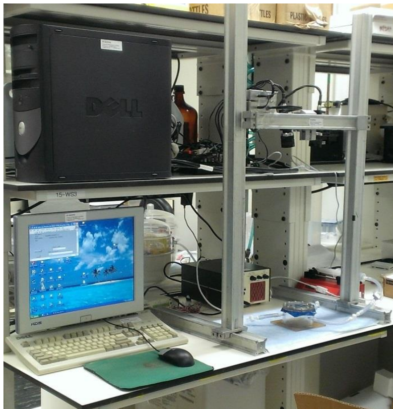
Figure 4-1: Biaxial Bulge Test set-up.
