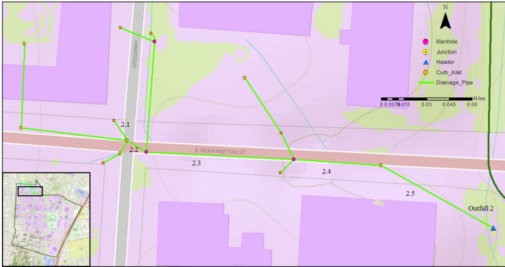
Figure 4.13: The stormwater system that discharges to Waller Creek from Dean Keaton Street
