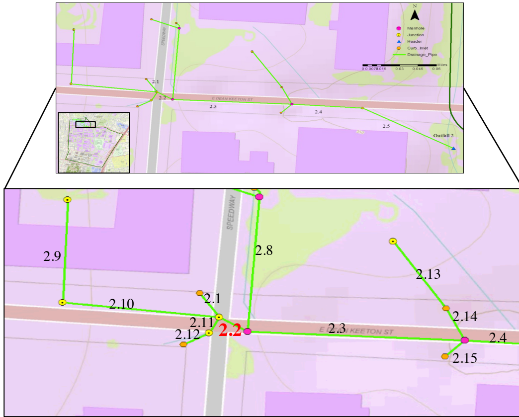
Figure 4.16: Pipeline with unique label 2.2 has a ratio of flow to the total capacity higher than 100% for a 100-yr scenario.
