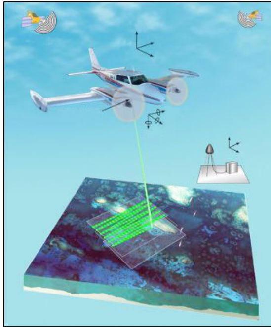
Figure 2.6: Airborne LiDAR system with bathymetric sensor (USGS, 2007)
