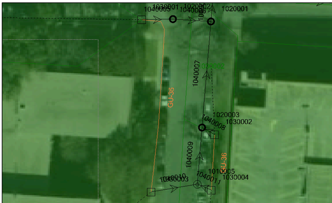
Figure 3.14: Gutter drawn in StormCAD with imagery of the area analyzed as background
