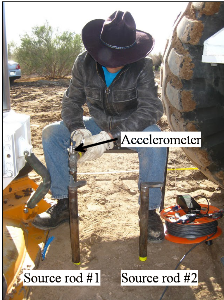
Figure 33. Photograph of crosshole test in progress. The source hammer is outfitted with an accelerometer and is being used to strike the top of source rod #1.
