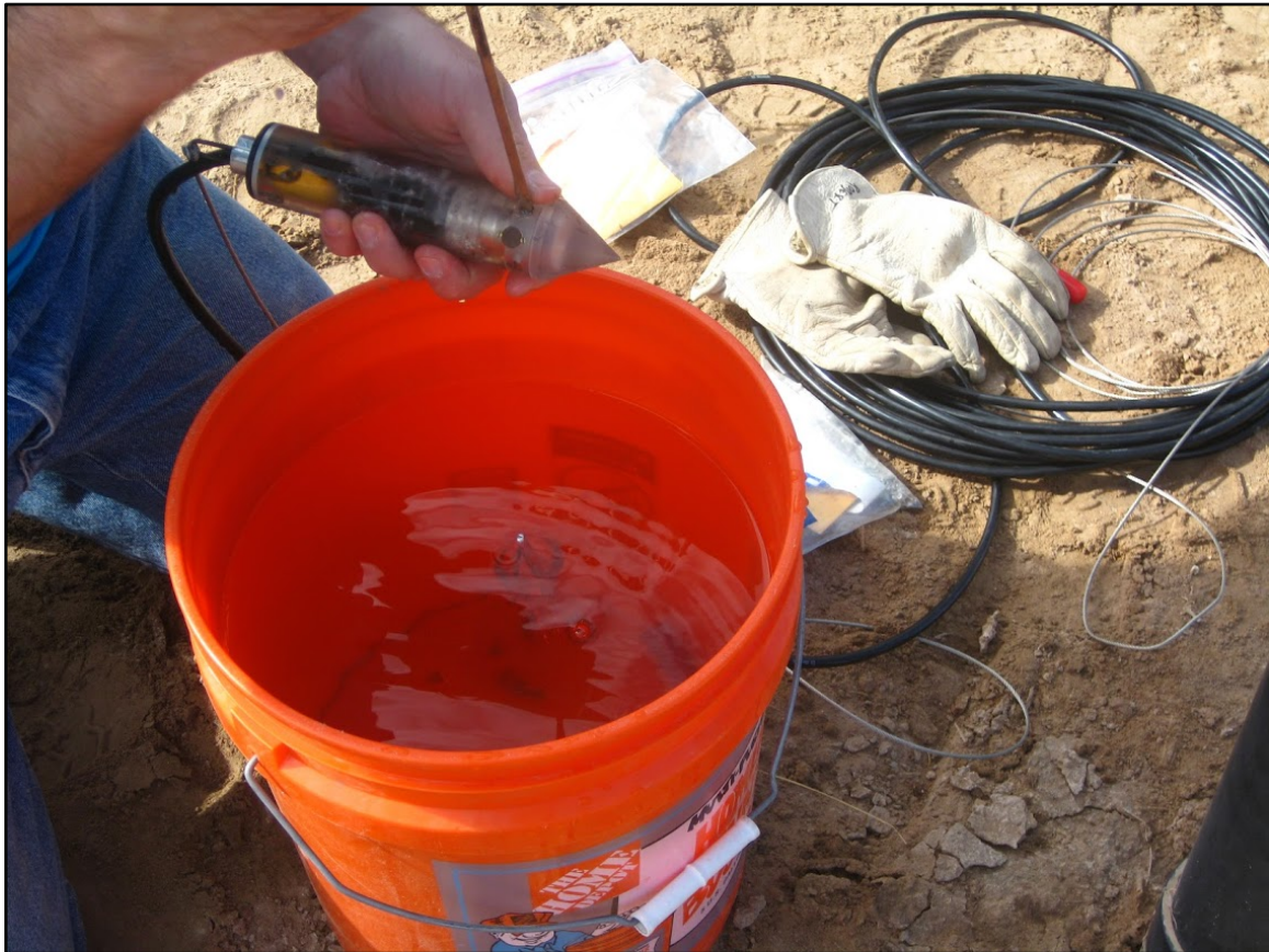
Figure 30. Preparing to submerge the pore pressure sensor in the 5-gallon water bucket. While difficult to see, filters and tools are at the bottom of the bucket, saturated and ready for sensor preparation.
