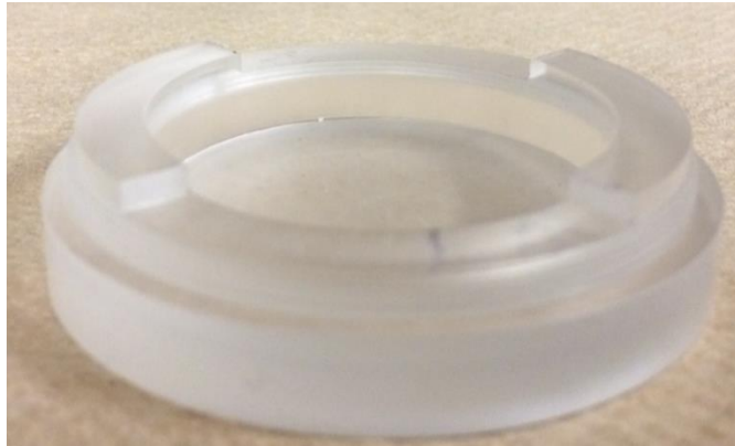
Figure 4.10: View of Notches in Bottom Portion of New Permeameter Cup
