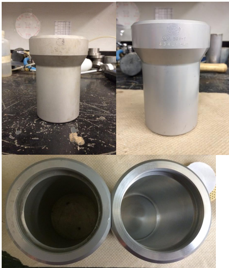
Figure 4.4: IEC Models CAT 384 (top left) and interior (bottom left) and 834s (top right) and interior (bottom right)
