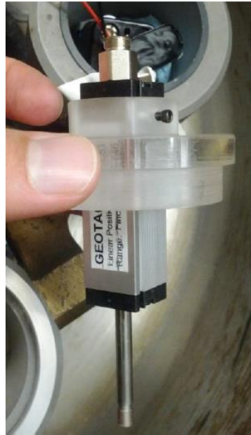
Figure 4.5: Linear Position Sensor (LPS) used in DAS (Walker 2012)
