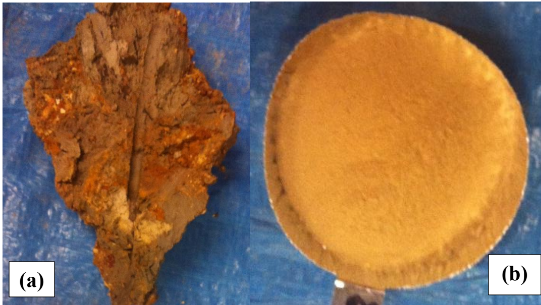
Figure 3.3: Cook Mountain Formation (a) view prior to processing and (b) view after post-processing (right)
