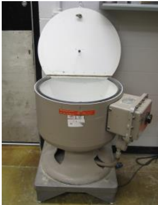
Figure 4.2: Damon IEC XRD Centrifuge (Plaisted 2009)
