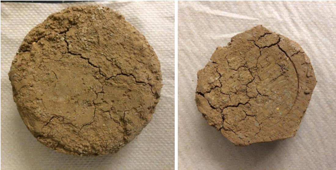
Figure 6.5: Cracks in Specimens Compacted Dry after Moisture Conditioning
