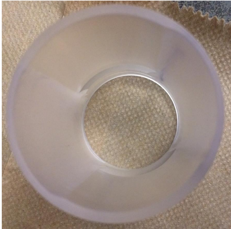
Figure 4.9: Top View of Top Portion of Permeameter Cup for Double Infiltration Centrifuge Set-up
