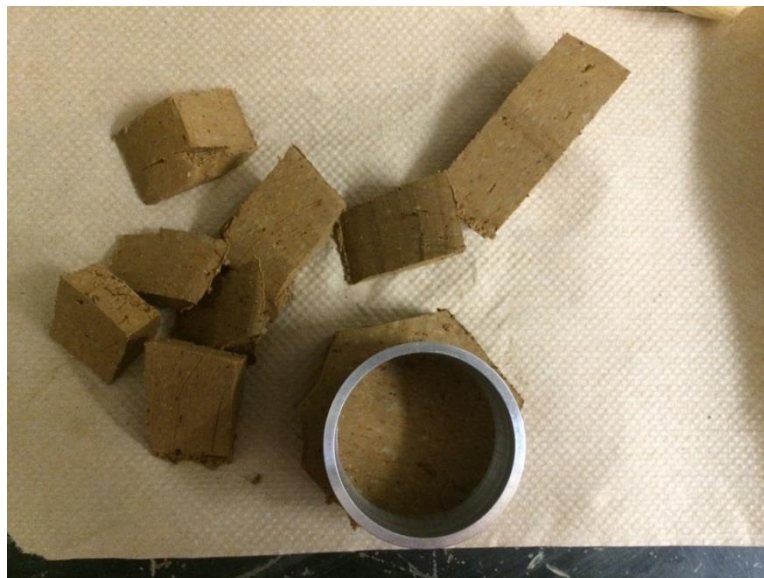
Figure 4.16: Cutting of Excess Soil during Insertion of Cutting Ring
