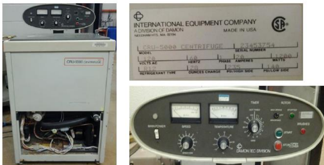
Figure 4.1: Damon IEC CRU-500 Centrifuge and Control Board (Walker 2012)
