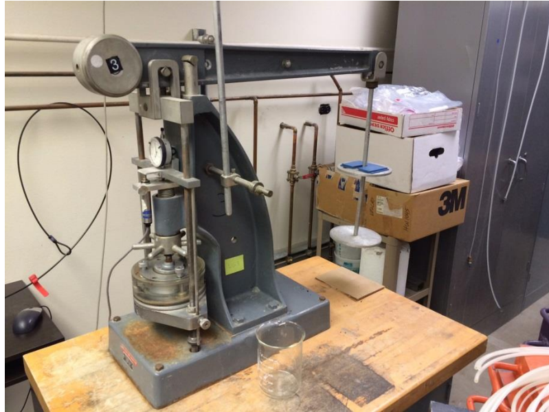
Figure 4.12: Consolidation Frame used for ASTM D4546 Testing
