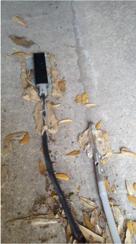
Figure 8. Sampler Tube Intake and Area Velocity Probe at Pon Court Basin Inlet.
