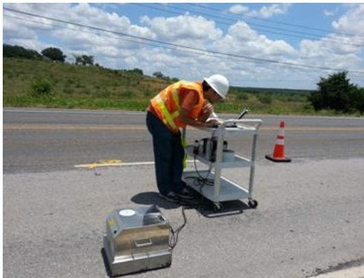
Figure 3.25: Circular Track Meter (CTM) Figure 3.26: CTM testing location
