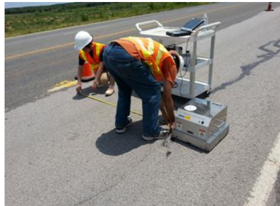
Figure 3.25: Circular Track Meter (CTM) Figure 3.26: CTM testing location
