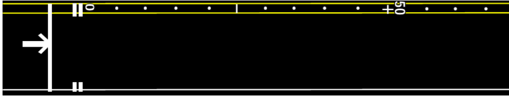
Figure 3.4: Schematic of section and subsection markings (beginning of section shown)
