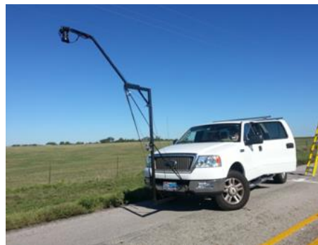
Figure 3.39: Vehicle ready for taking crack map pictures
