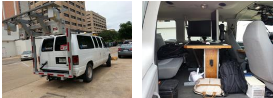
Figure 3.28: Dynatest van –back and inside
