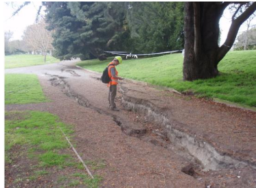
(b) Measurement of Crack with GPS
