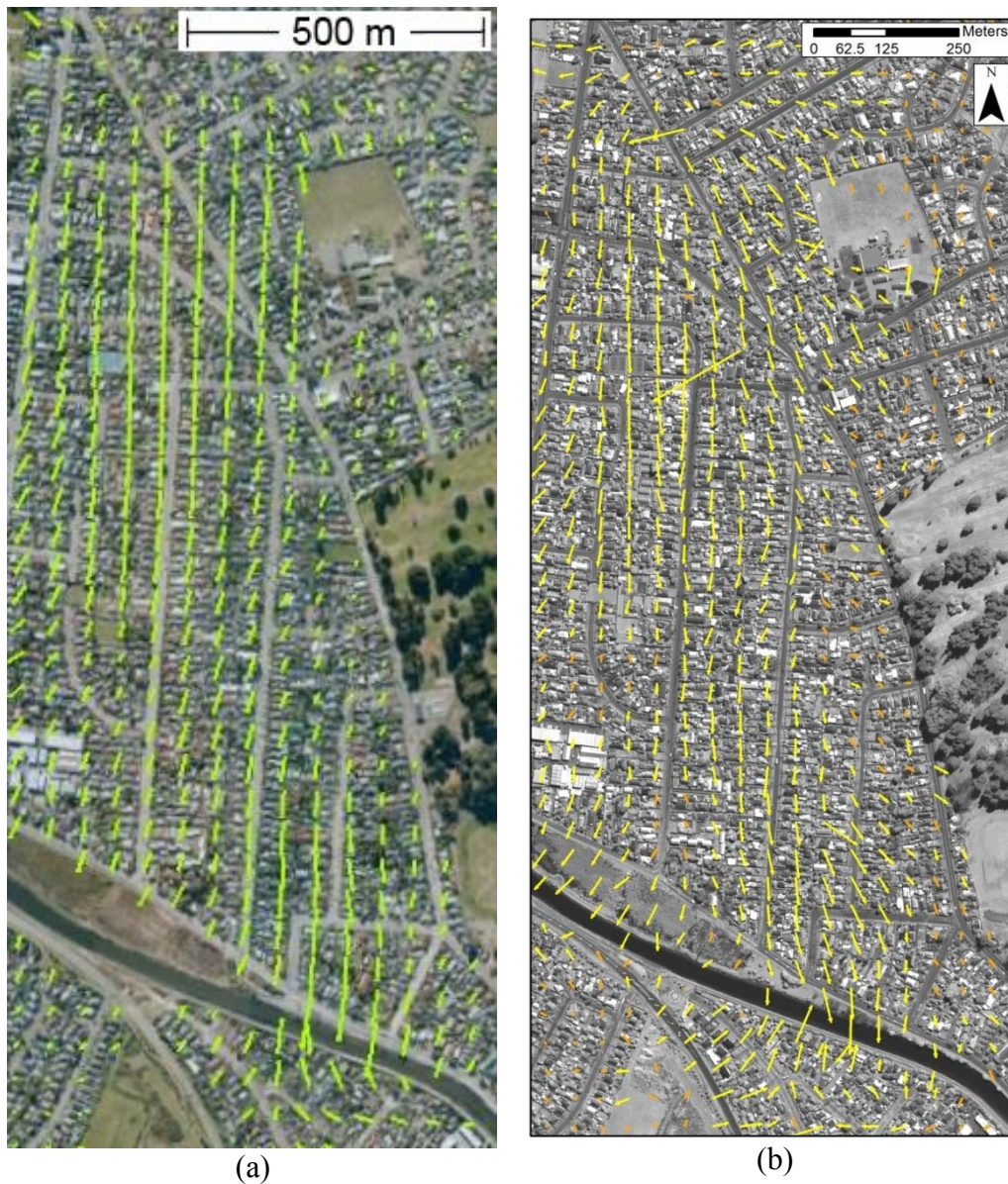
Figure 3.27. (a) LiDAR displacement measurements and (b) displacements from optical image correlation in New Brighton (Canterbury Geotechnical Database 2012a).
