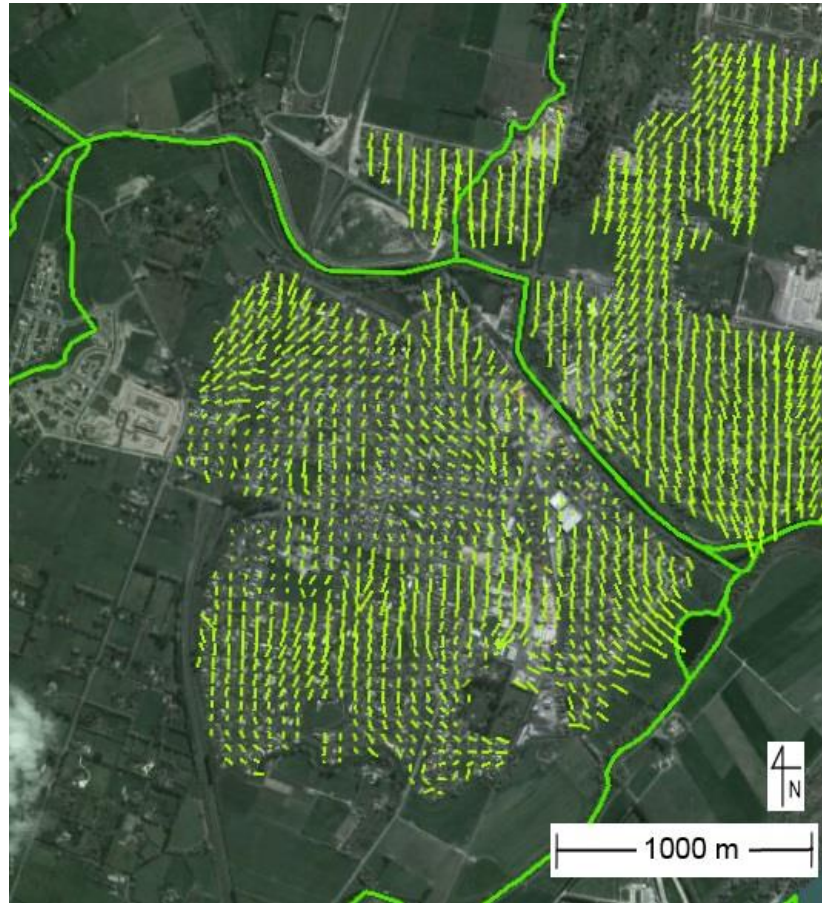
Figure 4.13. Displacements from LiDAR correlation rendered as arrows scaled 56:1 (Beavan et al. 2012).
