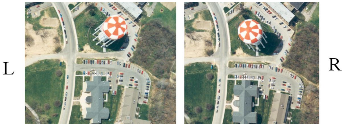
Figure 2.4. Relief displacement of top of water when viewed from left and right of tower. (Bethel 2014)
