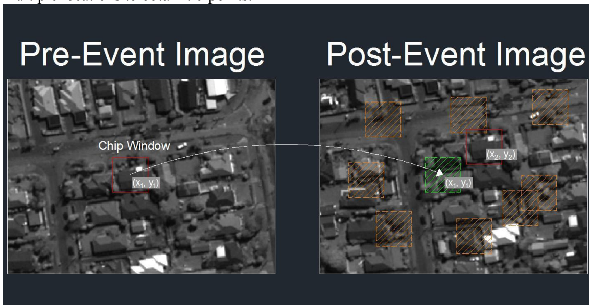
Figure 2.6. Optical Image Correlation Process.
