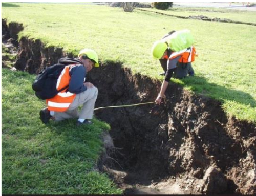
(a) Measurement of Crack using Tape
