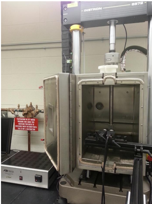
Figure 3.6: A 3-D two-camera DIC setup and loading frame (Instron 8872 UTM)
