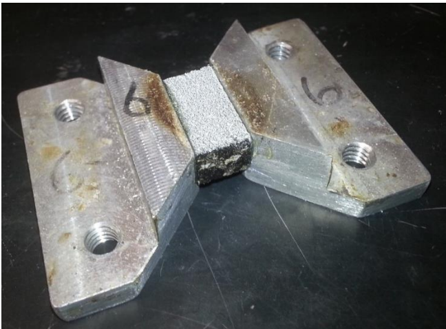
Figure 3.4: Specimen glued on the butterfly setup
