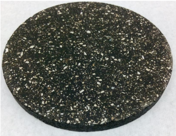
Figure 3.1: 10 mm thick slices from FAM cylinder
