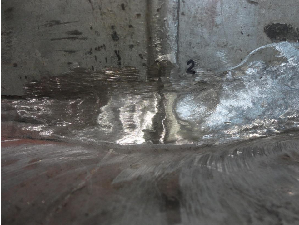
Figure A.2: Bend after the groove was filled
