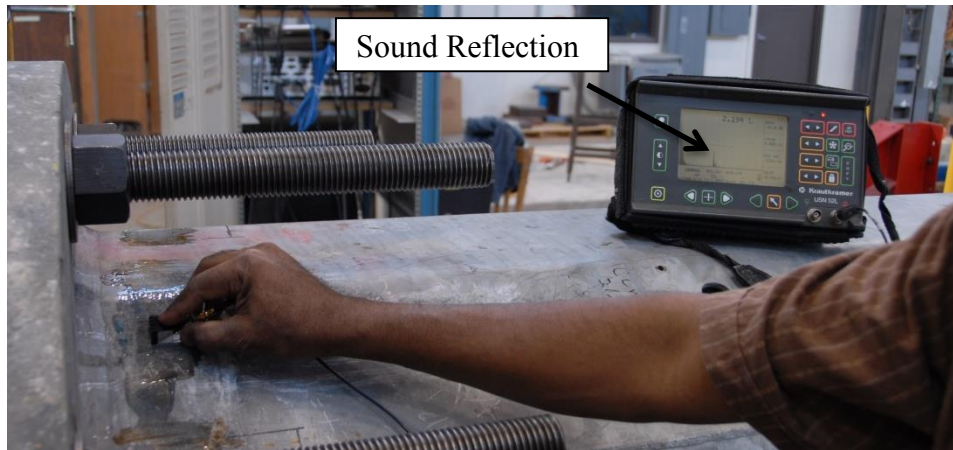
Figure 3.10: Technician performing UT on a HMIP while being tested at FSEL
