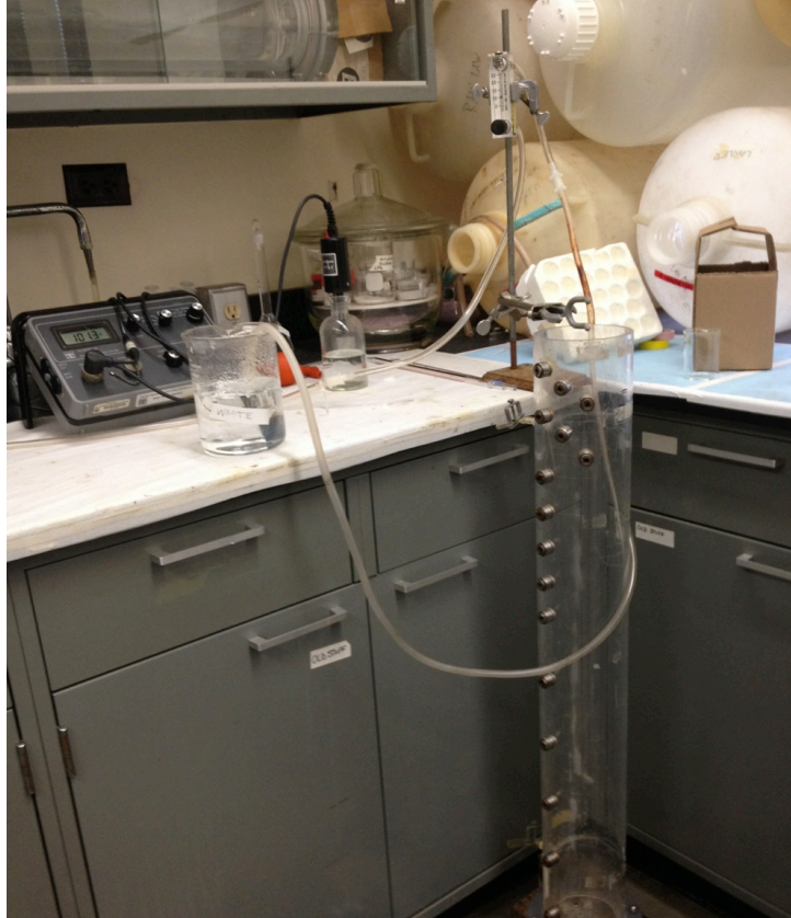
Figure 5.2: Setup for the bubble aeration tests
