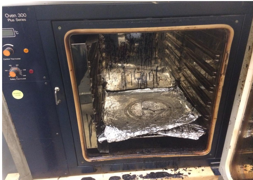
Figure 3.5 Adjustable temperature oven used for laboratory curing
