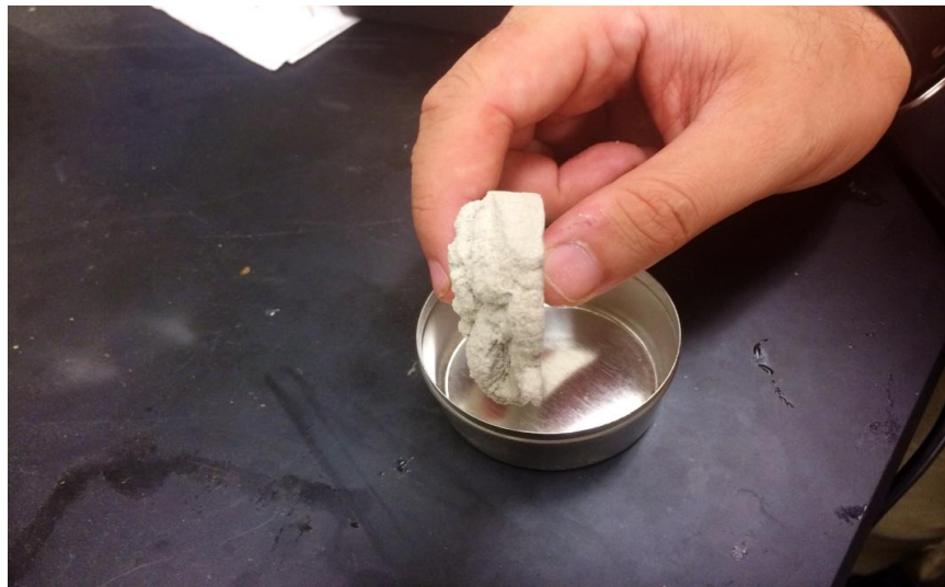
Figure 3.7 Water-Based Polymer Penetration on Reference fine sand
