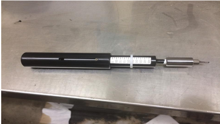
Figure 3.6 Pocket penetrometer with additional modified diameter tip
