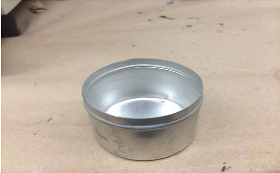
Figure 3.3 2.1 inch diameter by 1.4 inch high circular cans used for preparing specimens
