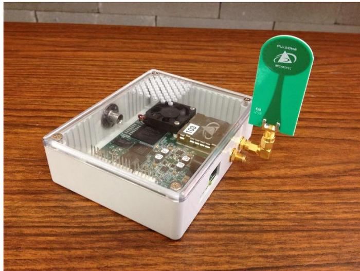
Figure 4.1: Time Domain P410 UWB transceiver
