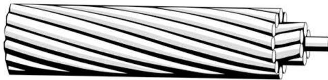
Figure 3. 4: Spiraling of a Conductor [2]
