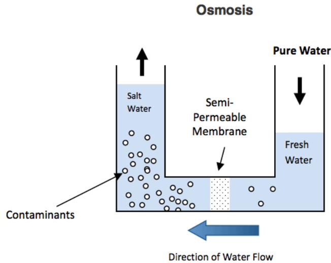
Figure 3.6: Schematic of the RO technology [17].
