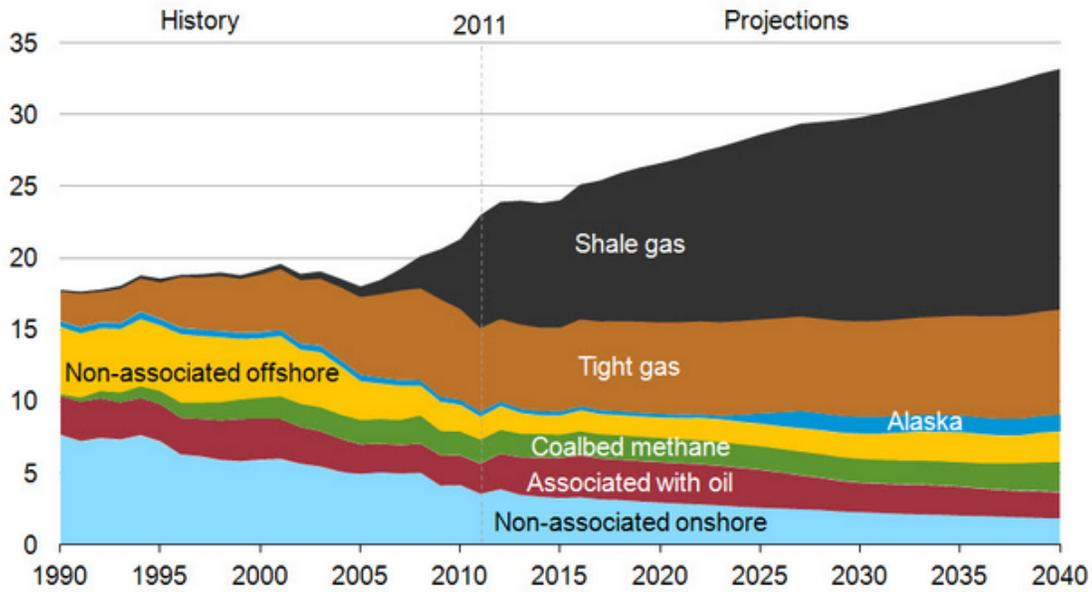
Figure 1.1: This graph shows historical and projected dry natural gas production by type in the U.S. in trillion cubic feet (TCF) [5].
