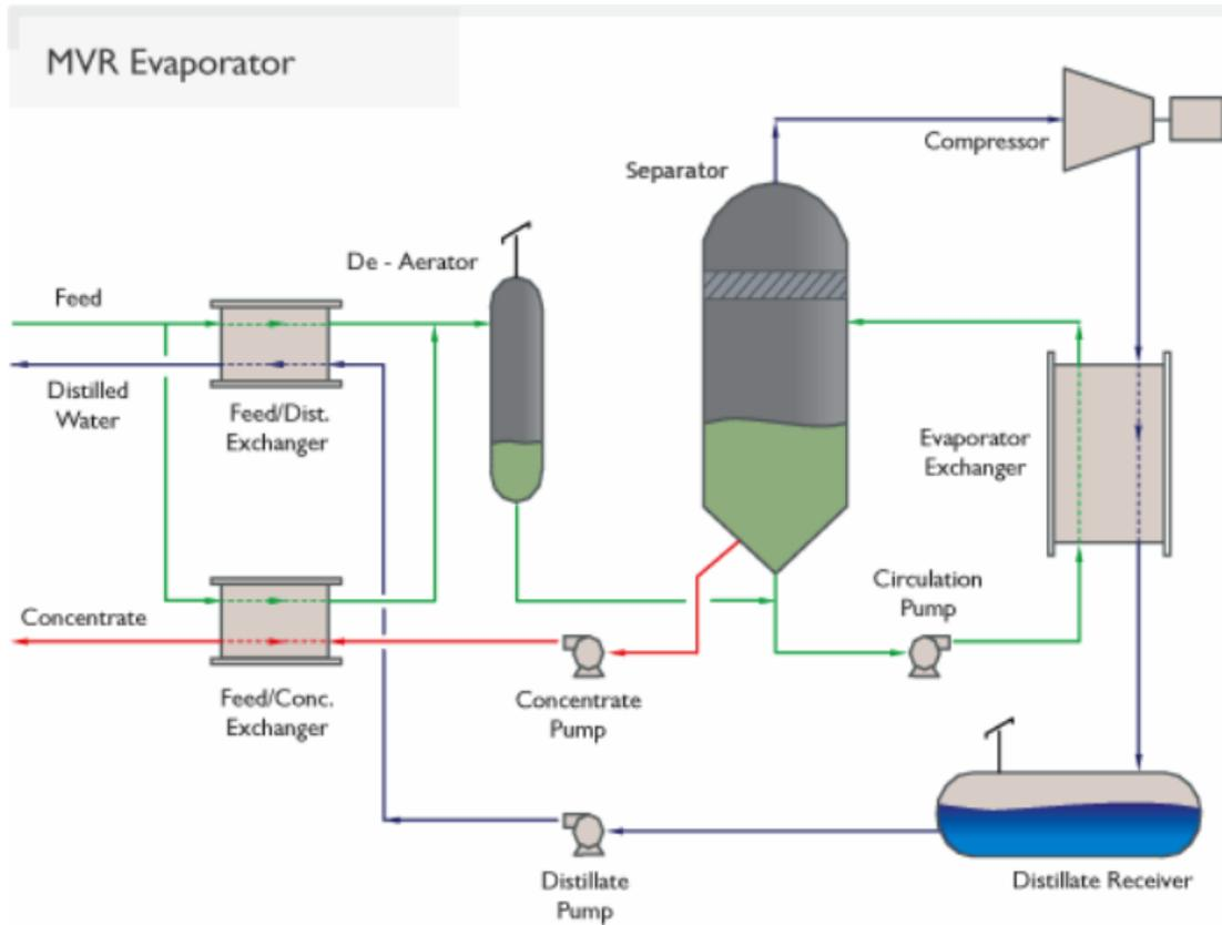
Figure 3.5: Schematic of the MVR distillation system [16].
