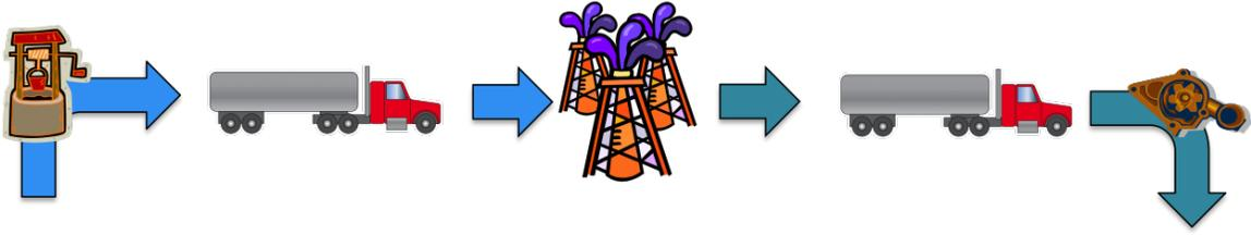
Figure 5.1: This figure shows the current water management strategy for hydraulic fracturing operations in the Permian Basin where the majority of the water is pumped from local groundwater, trucked or piped to the well site, used for fracking, and then trucked or piped to a disposal well. The schematic shows water being trucked to and from the well site instead of piped as this would be the worst case scenario from an energy intensity standpoint.
