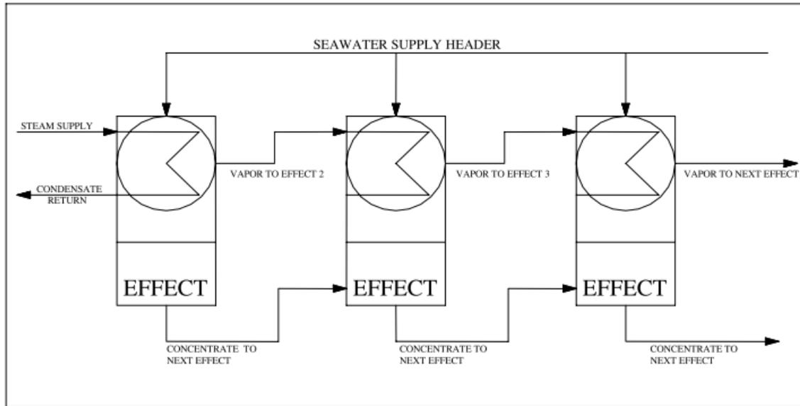
Figure 3.4: Schematic of the MED distillation system [15].
