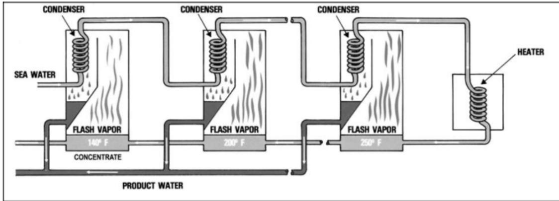
Figure 3.3: Schematic of the MSF distillation system [15].
