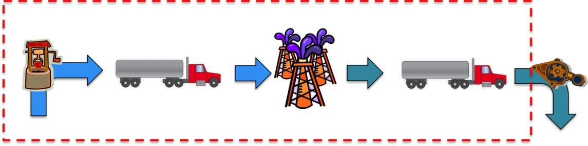
Figure 5.2: This figure shows the system boundaries for the current paradigm in this analysis. Included in the system boundaries are the energy for 1) pumping groundwater, 2) trucking the water to the well site, and 3) trucking the wastewater from the well site to a disposal well. Not included in the system boundaries are 1) the energy for hydraulic fracturing as this value is assumed to be the same in the current paradigm and proposed strategy and 2) the energy for DWI.
