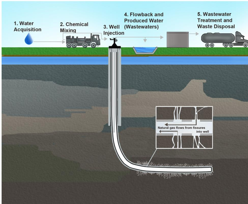
Figure 2.2: This figure depicts the hydraulic fracturing process from water acquisition to wastewater removal. While the picture shows the process including wastewater treatment and waste disposal, in Texas, the vast majority of the wastewater is trucked or piped to nearby disposal wells and does not undergo any treatment. Wastewater treatment is more prevalent in shale regions located in the northeastern U.S. [7] Note: Figure not drawn to scale.
