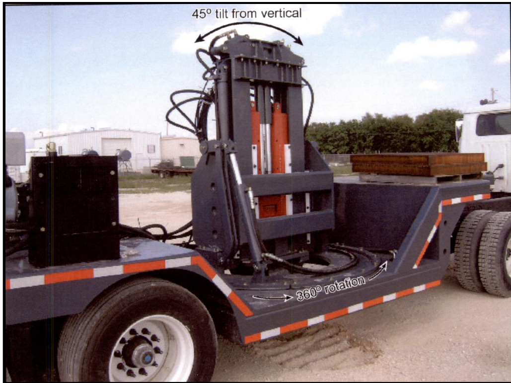
Figure 2.3: VSX accelerated-weight impact source provided by Vecta Technology and United Services Alliance. A vertical impact or an inclined force vector can be delivered to the Earth by this source. Note the reaction mass can be tilted to either side at an angle up to 45 degrees to produce shear waves of opposite polarities.
