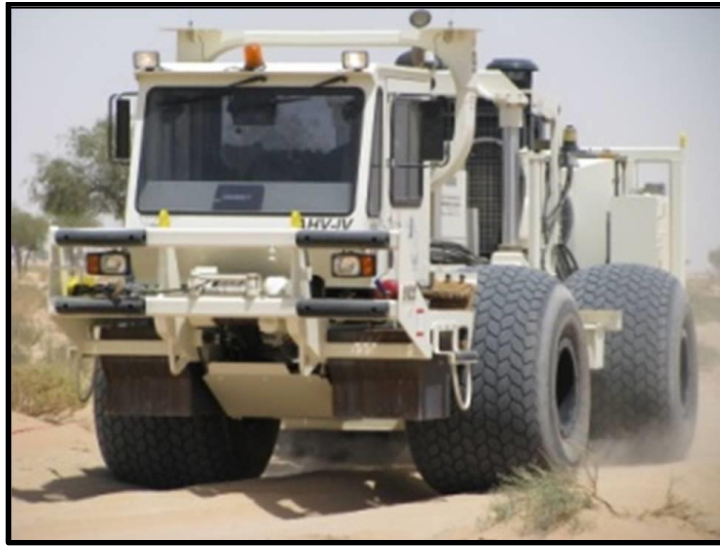
Figure 2.6: 60,000-lb vertical vibrator manufactured by Inova Geophysical Inc. In this study, this source generated a linear 8-second sweep from 8 to 96 Hz.
