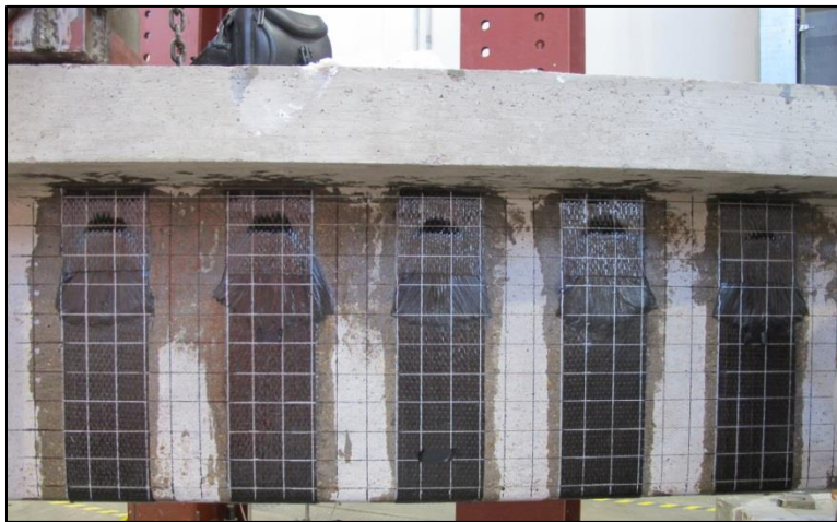
Figure 3-83: Grid lines drawn on the test span
