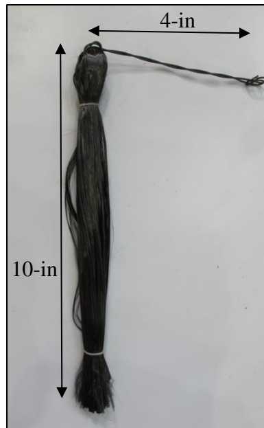
Figure 3-40: Typical CFRP anchor with 4-in. long insertion tool
