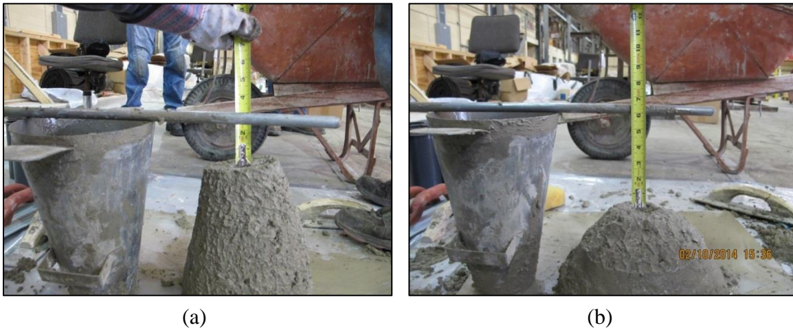
Figure 3-29: Adding water to maintain a 6-in. slump
