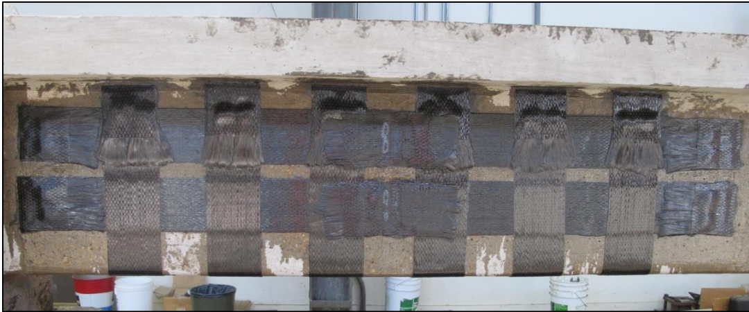
Figure 3-59: Bi-directional application layout for double layers configuration
