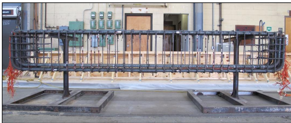
Figure 3-16: Transverse reinforcement for deep specimen with a/d of 1.5
