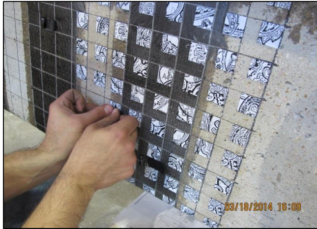
Figure 3-84: Placing paper targets in their location using spray adhesive
