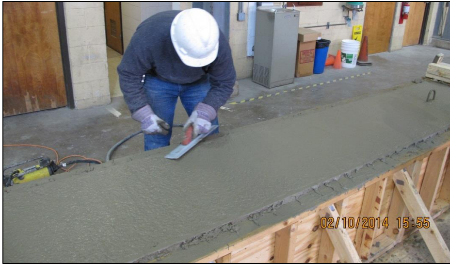
Figure 3-26: Finishing the specimen's top surface
