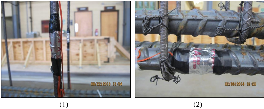
Figure 3-71: Protected strain gauge: (1) in transverse reinforcement, (2) in longitudinal reinforcement
