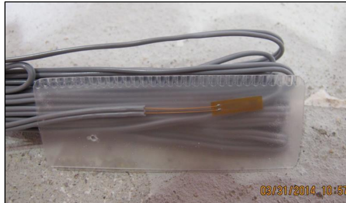
Figure 3-75: Typical strain gauge for composite material
