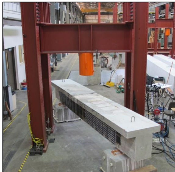
Figure 3-64: As-built test setup with 25-degrees rotation
