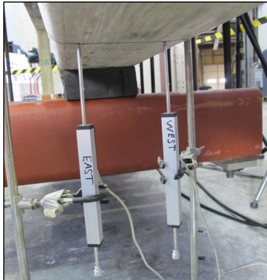
Figure 3-81: LVDT's to measure mid-span displacement
