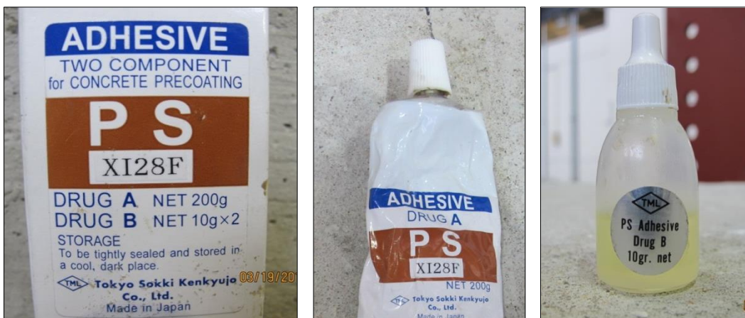
Figure 3-76: The two components adhesive used to provide smooth surface
