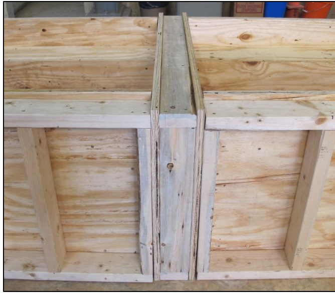
Figure 3-10: Form divider allowing for casting two specimens at the same time
