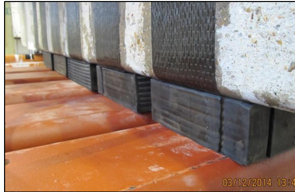
Figure 3-68: 3-in bearing pads to protect the web of the specimen
