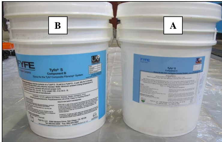
Figure 3-44: The two components of the epoxy
