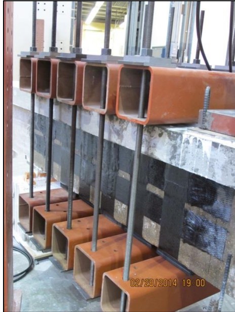
Figure 3-67: External clamps for specimens of a/d = 3
