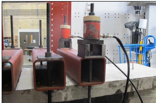
Figure 3-69: Two hydraulic rams pre-stressing not tested region
