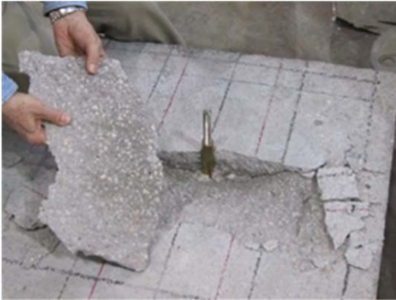
a) concrete cone breakout
