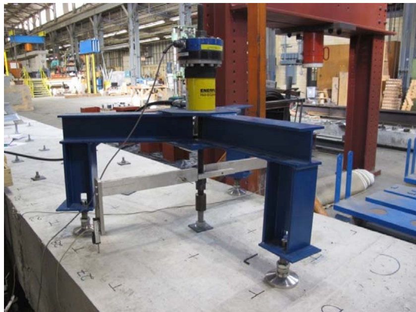
Figure 3-18: Unconfined Test Setup with Larger Steel Tripod
