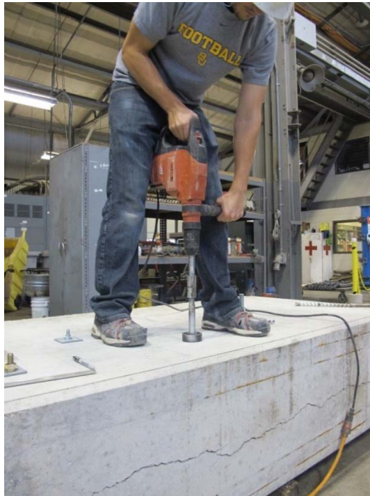
Figure 3-15: Undercutting the Drilled Hole
