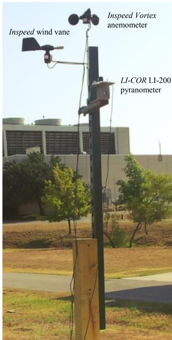
Figure 3.1: Weather monitoring instruments installed at The Pickle Research Campus, The University of Texas at Austin
