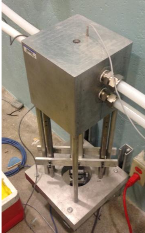
Figure 2.5: The mounted, permanent diverter.
