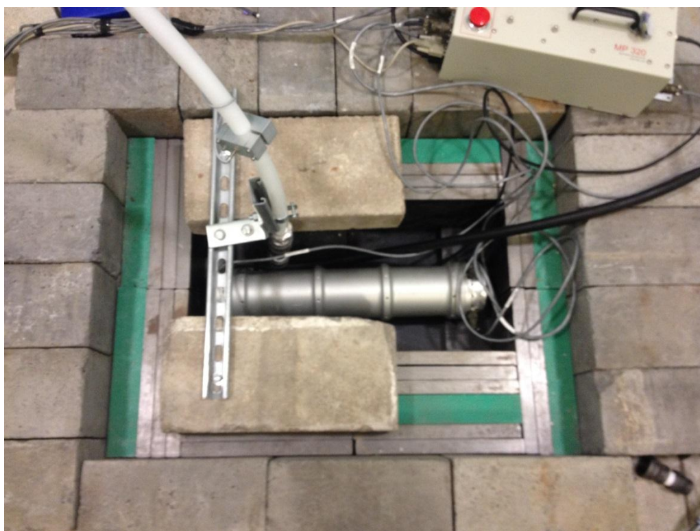
Figure 3.1: Neutron generator from above; note surrounding stainless steel plates (silver), borated polyethylene (green), and leaded concrete.
