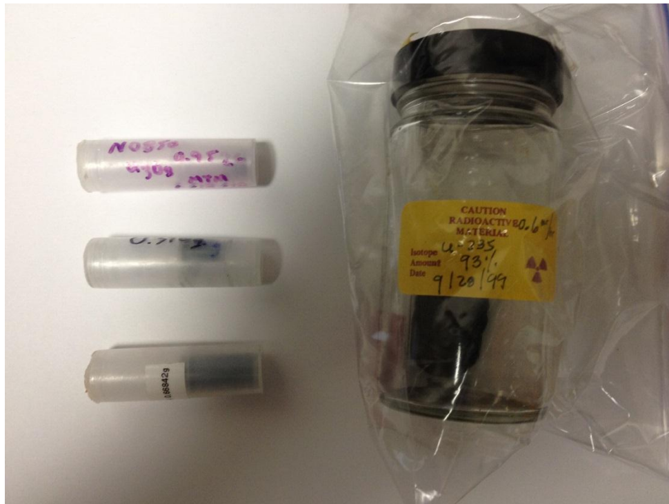
Figure 4.3: Uranium samples used to determine fission products. Top left, natural uranium ore ( U_3O_8 ) - 0.952g. Middle left, enriched (63%) uranium ore ( U_3O_8 ) - 0.376g. Bottom left, shredded HEU (93%) foil- 0.668g. Right, 4x HEU (93%) foils- 21.122g.
