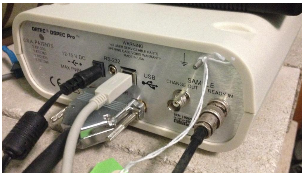
Figure 2.15: DSPEC Pro being gated using a standard RG-56 coaxial cable from the prompt gamma reduction prototype circuit.
