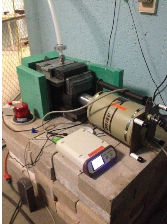
Figure 2.12: The detector system, a portable Ortec HPGe SMART detector coupled to a custom-made DSPEC Pro.
