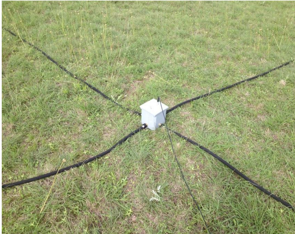
Figure 1.2: Microporous wind filter with microphone in sealed box.
