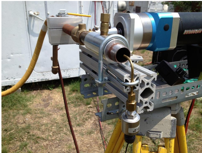
Figure 2.6: Pitot tube setup at outlet with short nipple in aluminum collar.
