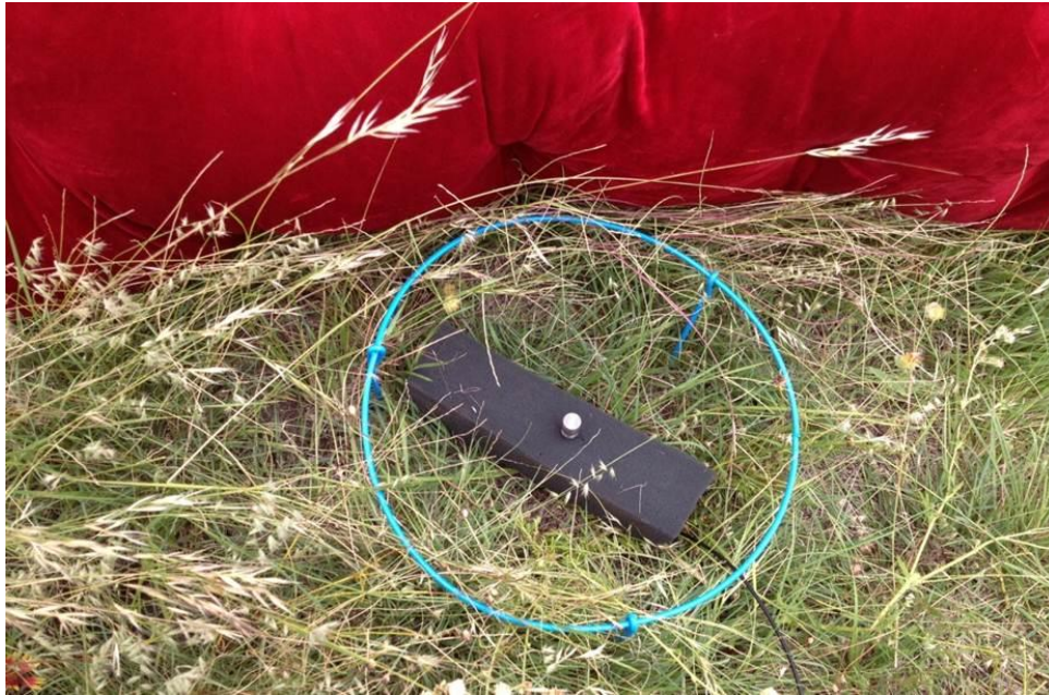
Figure 1.4: Microphone in foam support under metal frame (blue) to support wind cushion (red).
