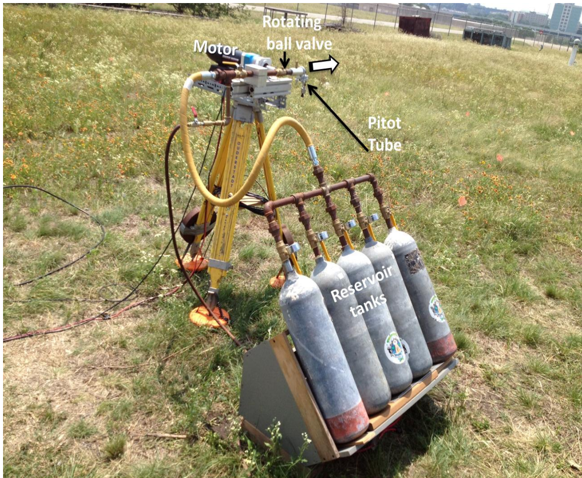
Figure 2.5: Photograph of system with horizontal jet nozzle configuration.
