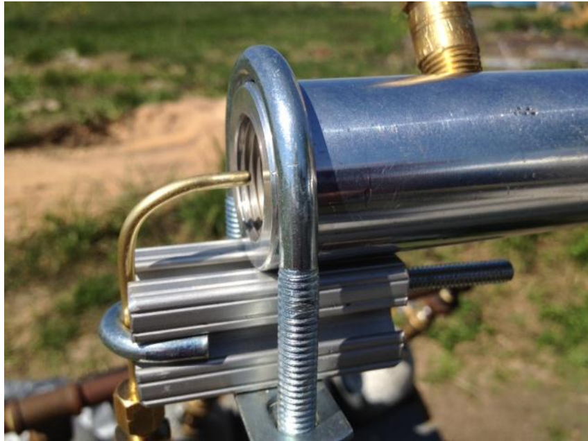
Figure 2.7: Pitot tube setup at outlet of aluminum collar.
