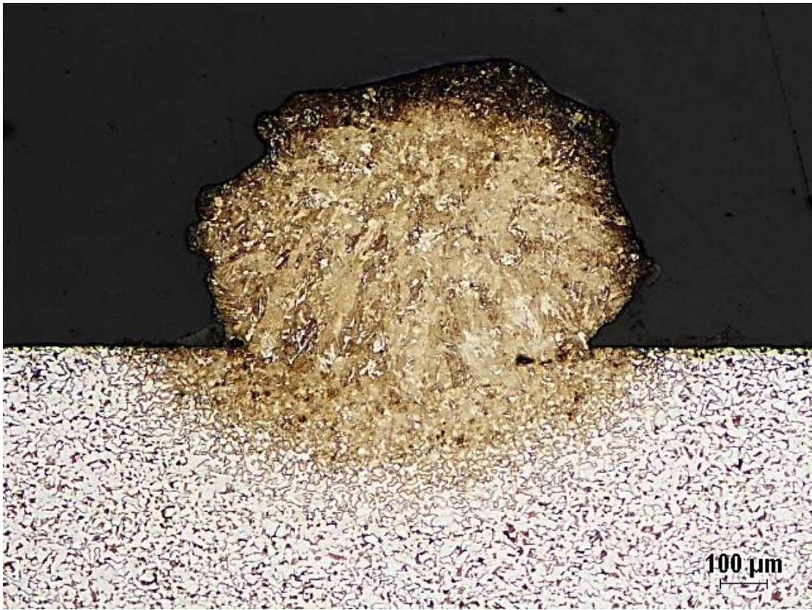
Figure 42: 10× micrograph of the crosssection of the single pass deposition from test series one
