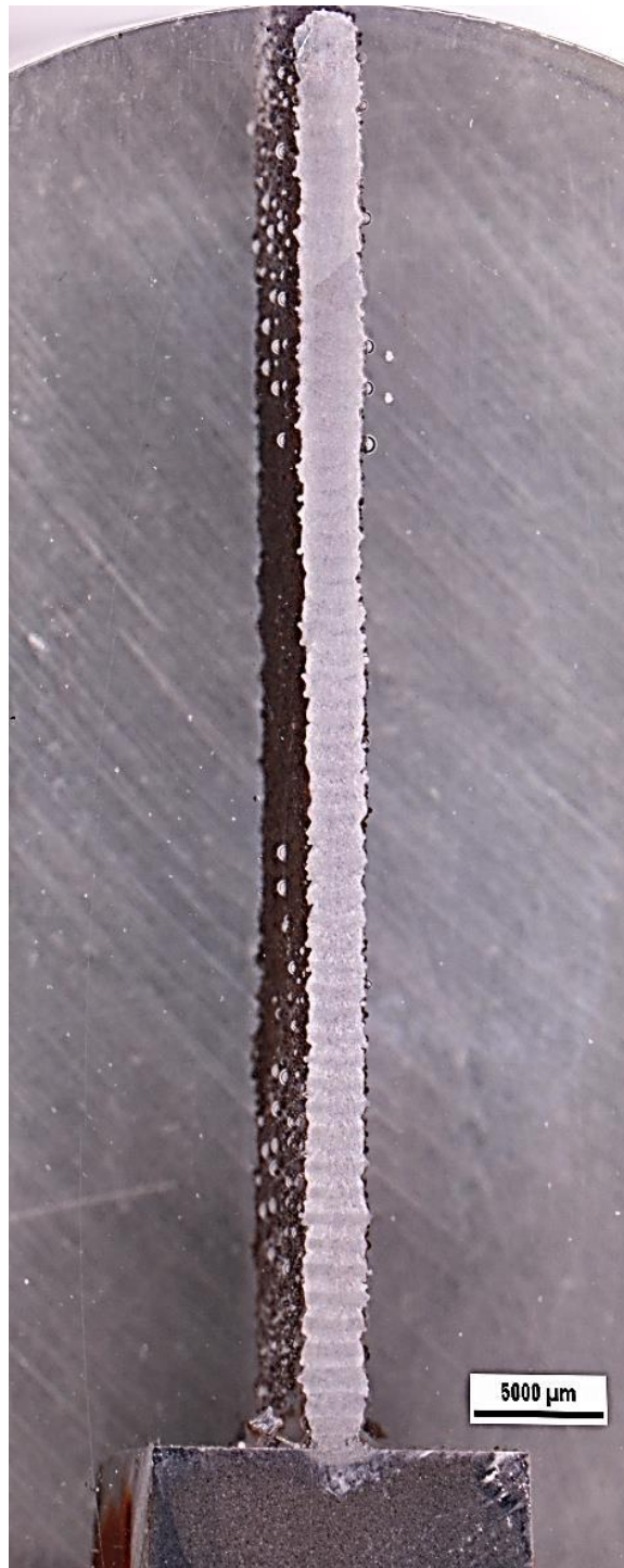
Figure 48: Stereo-microscope cross section image of the one inch wall deposition from test series one
