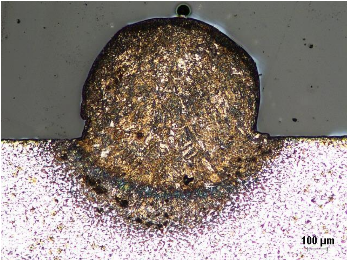
Figure 47: 5× micrograph of the crosssection of the two pass deposition from test series three
