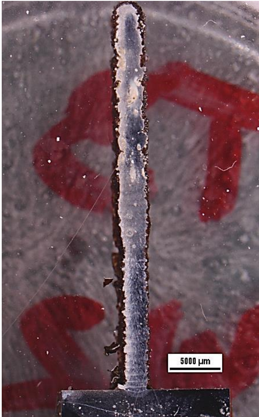
Figure 50: Stereo-microscope cross section image of the one inch wall deposition from test series three
