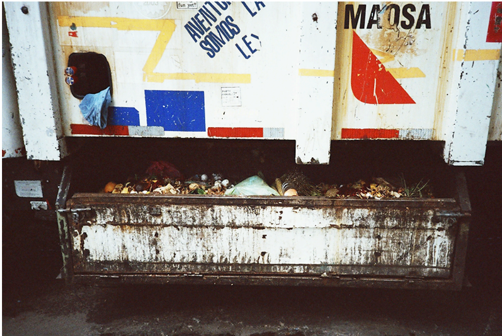
Figure #9: Example of trash trucks that have been informally outfitted with separate compartments for organic trash
