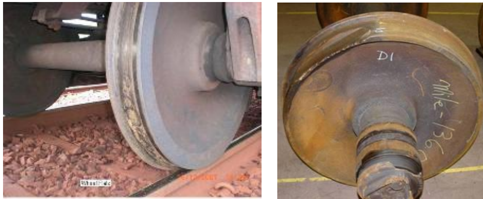
Figure 3-2: Wheel Surface Defects and Flat Spot [www.tsb.gc.ca]
