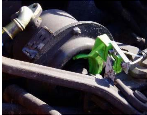
Figure 3-14: Proximity sensor for brake piston stroke measurement [FRA Research Results, 2009]
