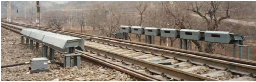
Figure 3-7: Trackside Acoustic Detection System TADS® [Transportation Technology Center, Inc.]
