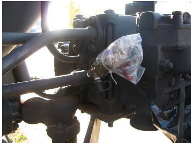
Figure 3-15: Brake pressure transducer on instrumented research truck [FRA, 2010]
