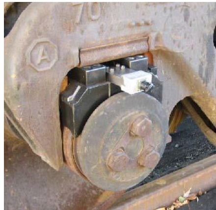
Figure 3-17: Vertical load adapter with strain gages to measure vertical wheel forces [FRA – Instrumented Tank Car, 2010]
