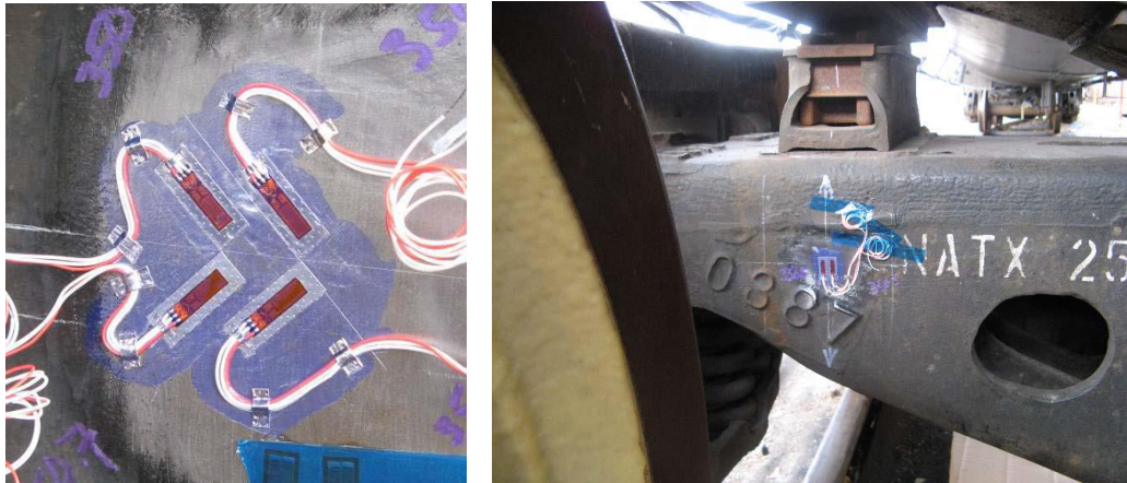
Figure 3-16: Strain gages mounted on the couler and bolster for test purposes [FRA – Instrumented Tank Car, 2010]
