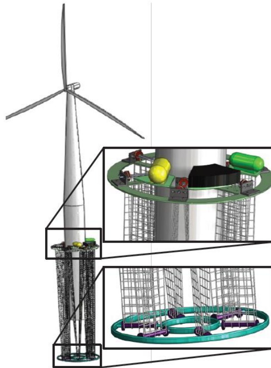
Figure 18. Symbiotic Mooring Scheme. For easiness to see, only 6 loops of belt instead of 20 are drawn in the figure. (Baelden 2013)
