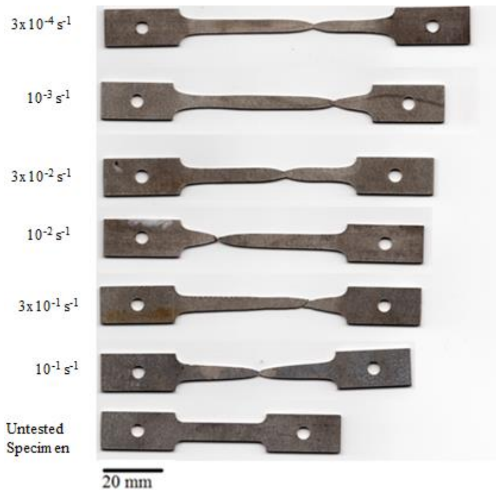
Figure 4.2: Specimens with the TD parallel to LTD, tested at a temperature of 300°C. The tested specimens demonstrate a diffuse neck.
