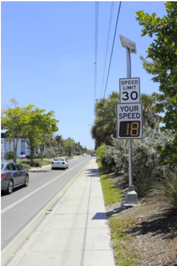
Illus. 1. Dynamic Speed Display Sign: a feedback loop used to curtail speeding. Photo: Serenethos/Shutterstock.com (editorial use only license).
