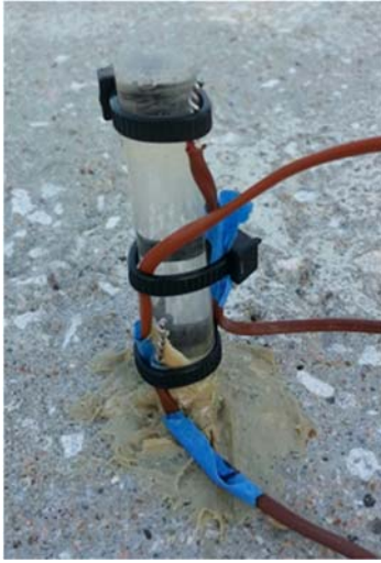
Figure 79: Thermocouples at Mid-Span of each Repair Section
