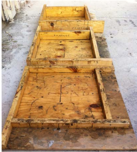
Figure 51: The 3 Temperature Gradient Slabs Formwork
