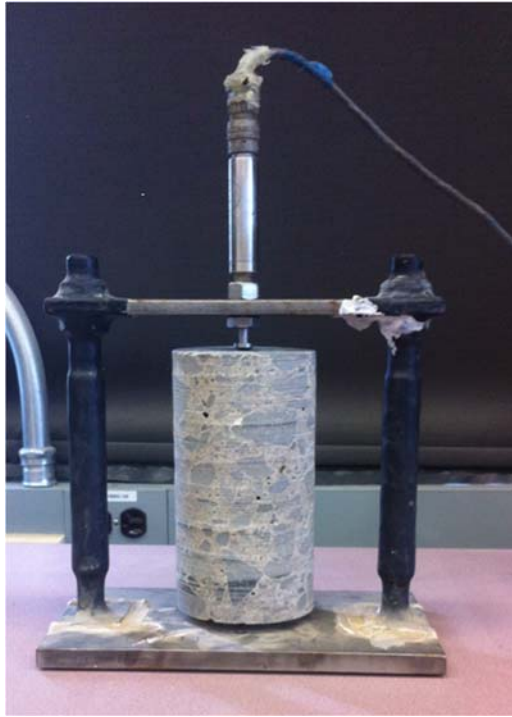
Figure 18: Coefficient of Thermal Expansion Setup
