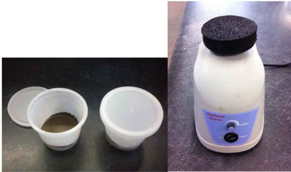
Figure 28: A) Grace AdiaCal TC Calorimetry Sample Holder (Bentivegna, 2012) B) Ultrasonic Mixer used for Paste Samples
