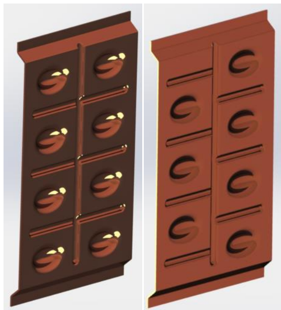
Figure 4.21: The redesign of fin half with a symmetric version (left) and an asymmetric version (right)
