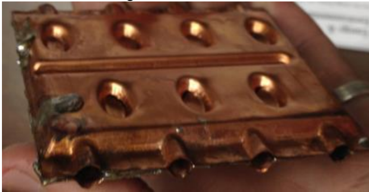
Figure 4.7: Soldered fin halves
