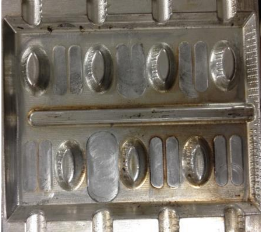
Figure 4.6: The male mold with slot features removed and dimple features tapered
