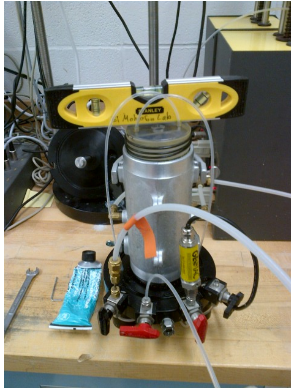
Figure 3-7: Specimen in Mold on Triaxial Base
