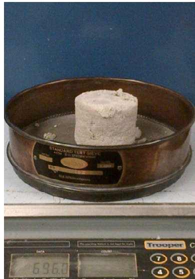
Figure 3-21: Weighing Specimen in Sieve
