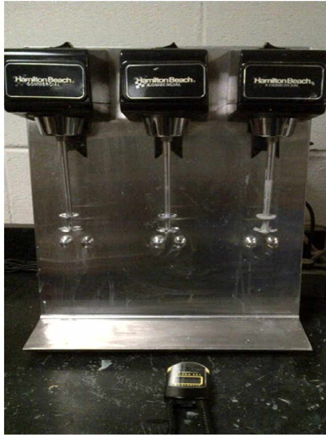
Figure 3-20: Hamilton Beach High Shear Mixer with timer
