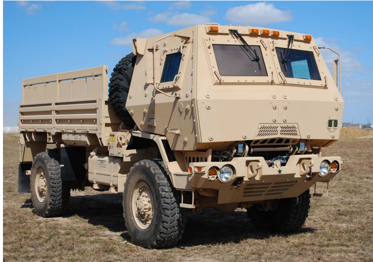
Figure 2.7: FMTV Light Vehicle, B-Kit (Appliqué Armor Panels Installed) Configuration [29]
