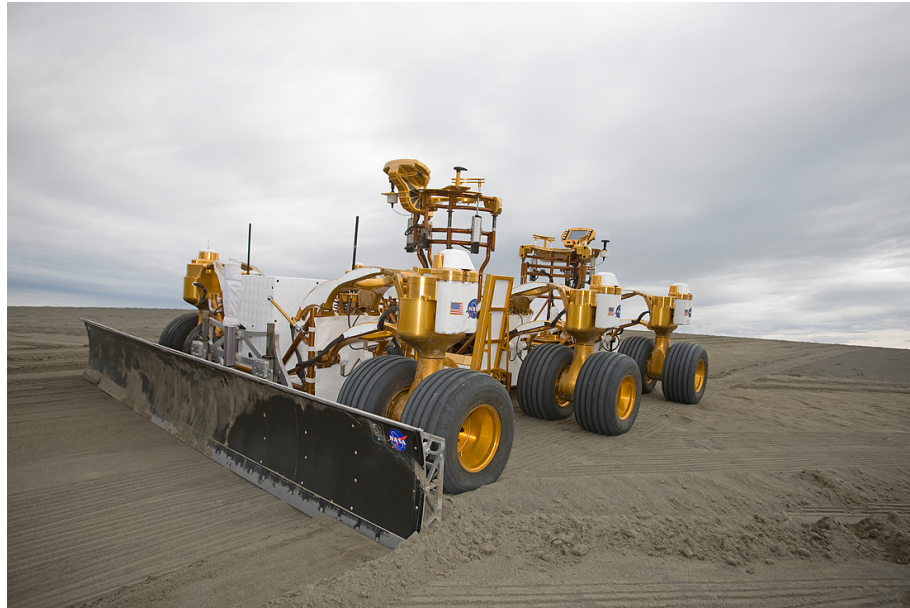
Figure 4.32: Chariot Platform with Bulldozing Attachment (Grading Blade)
