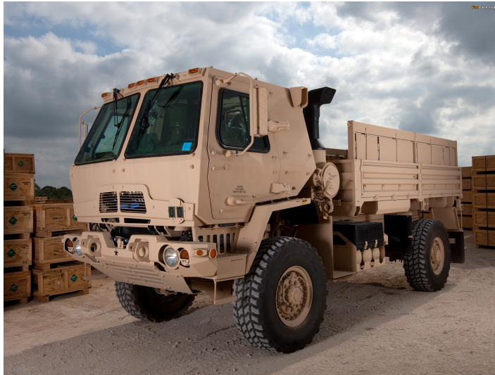
Figure 2.6: FMTV Light Vehicle, A-Kit (Base Armor) Configuration [29]
