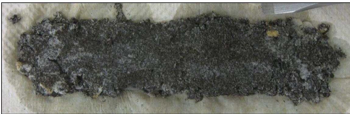
Figure 4.33: Mixture of 50% 40/70 ceramic and 50% 40/70 sand after exposure to stress. The screwdriver is included for scale.
