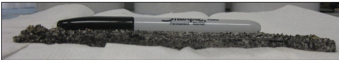
Figure 4.14: Cross-sectional view of mixture of 50% 20/40 sand and 50% 20/40 ceramic after exposure to stress. The marker is included for scale.
