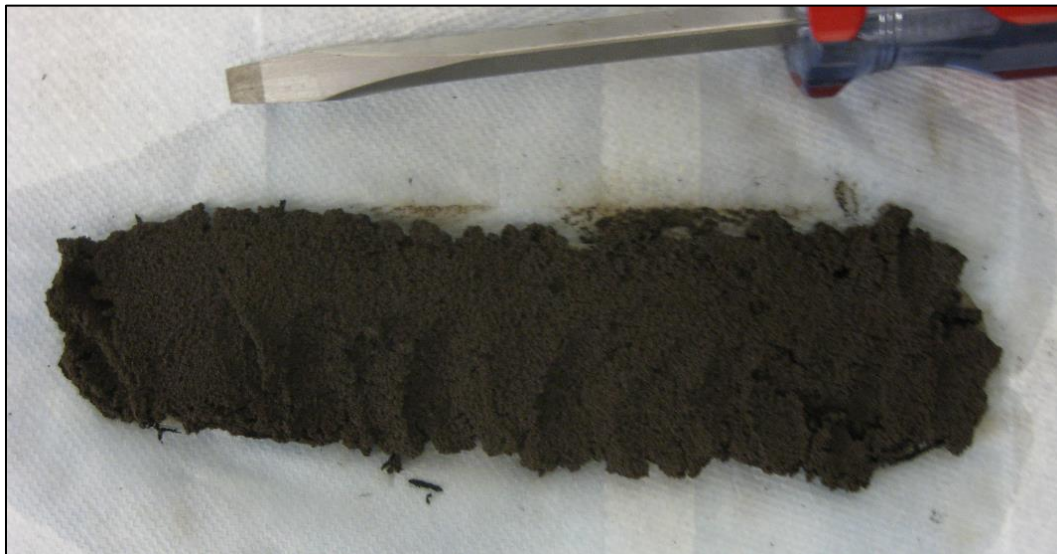
Figure 4.8: 40/70 ceramic pack after exposure to stress. The screwdriver is included for scale.
