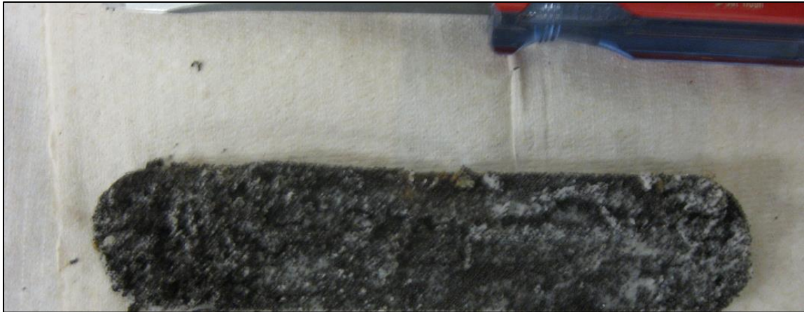
Figure 4.27: Mixture of 50% 20/40 ceramic and 50% 40/70 sand after exposure to stress. The screwdriver is included for scale.
