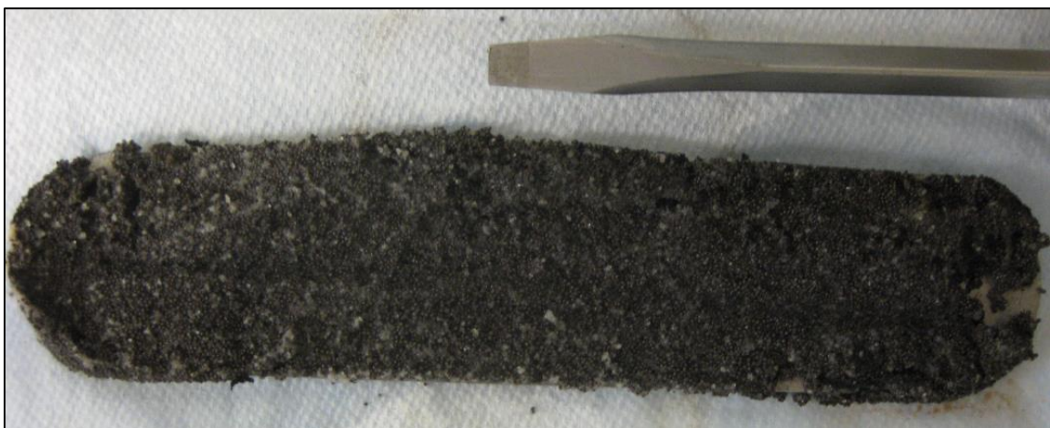
Figure 4.15: Mixture of 25% 20/40 sand and 75% 20/40 ceramic after exposure to stress. The screwdriver is included for scale.
