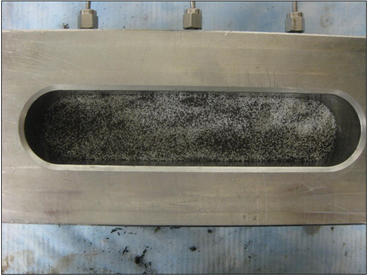
Figure 3.8: Fifty fifty mixture of 20/40 sand and 40/70 ceramic before testing.
