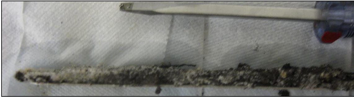
Figure 4.22: Cross-sectional view of mixture of 50% 20/40 sand and 50% 40/70 ceramic after exposure to stress. The screwdriver is included for scale.
