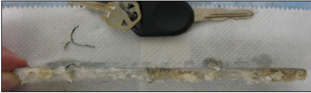
Figure 4.3: Cross-sectional view of 20/40 sand pack after exposure to stress. The key is included for scale.
