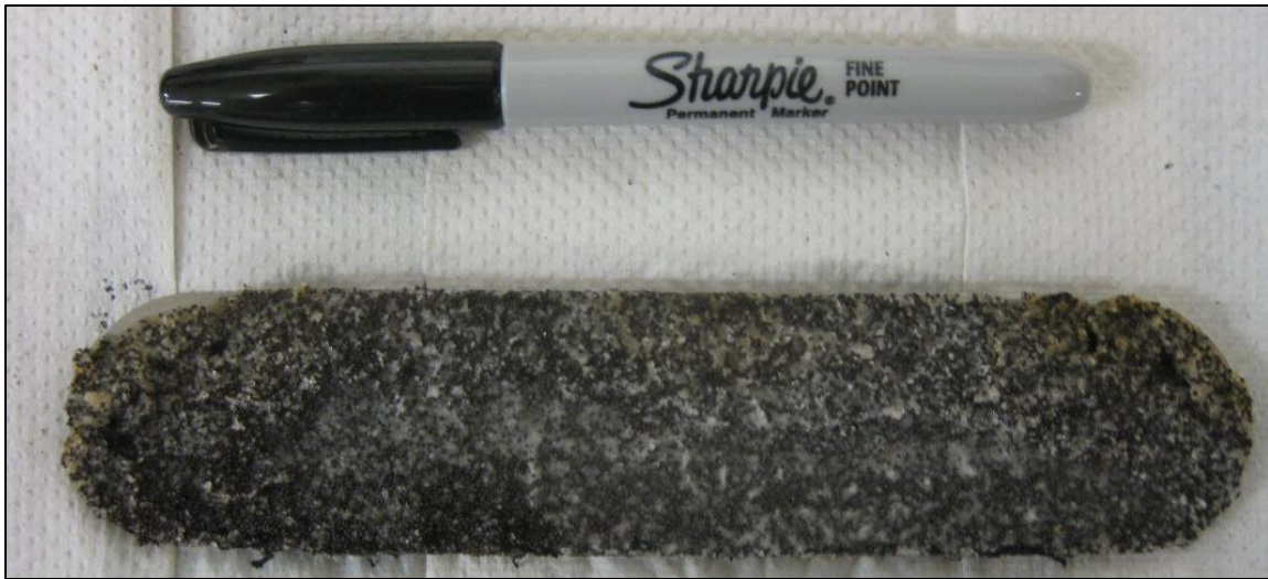
Figure 4.13: Mixture of 50% 20/40 sand and 50% 20/40 ceramic after exposure to stress. The marker is included for scale.
