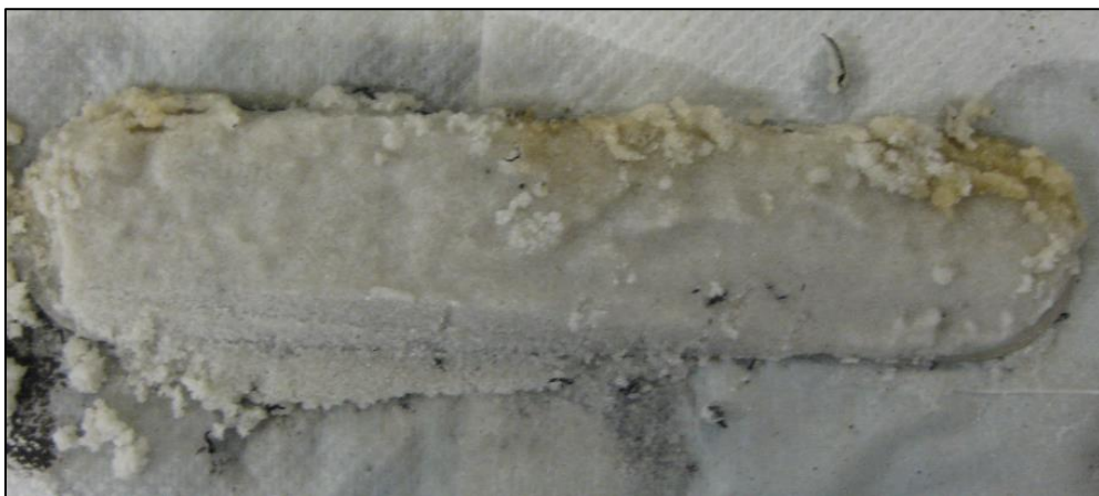
Figure 4.2: 20/40 sand pack after exposure to stress.
