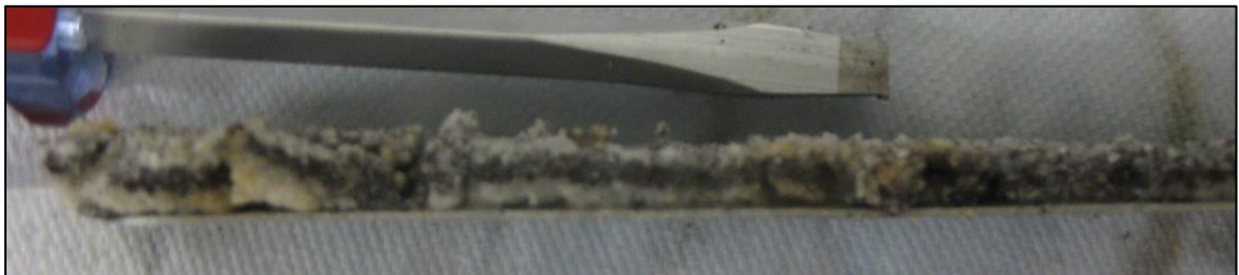
Figure 4.24: Cross-sectional view of mixture of 75% 20/40 sand and 25% 40/70 ceramic after exposure to stress. The screwdriver is included for scale.
