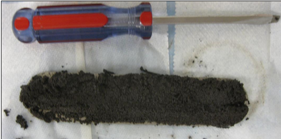
Figure 4.6: 20/40 ceramic pack after exposure to stress. The screwdriver is included for scale.
