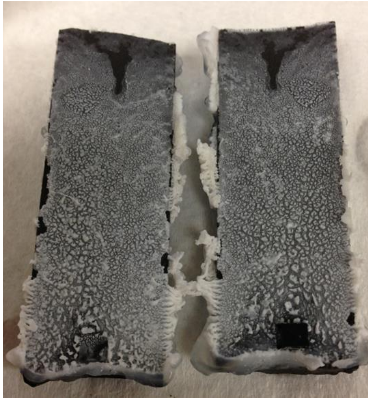
Figure 13: Interior of a cement fracture filled with 3 wt% Carbopol 934 polymer dispersion and allowed to sit for 4 days.
