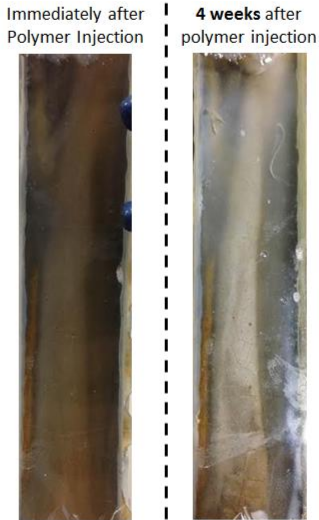
Figure 79: Photographs of Core 6FP-24 during and after polymer injection (3 wt% Carbopol 934 and 0 wt% NaCl). Core was pre-flushed with HCl acid.
