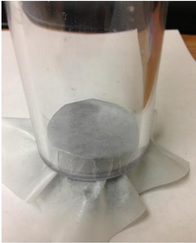
Figure 99: Wax paper and rubber stopped used to seal bottom of polycarbonate tube.
