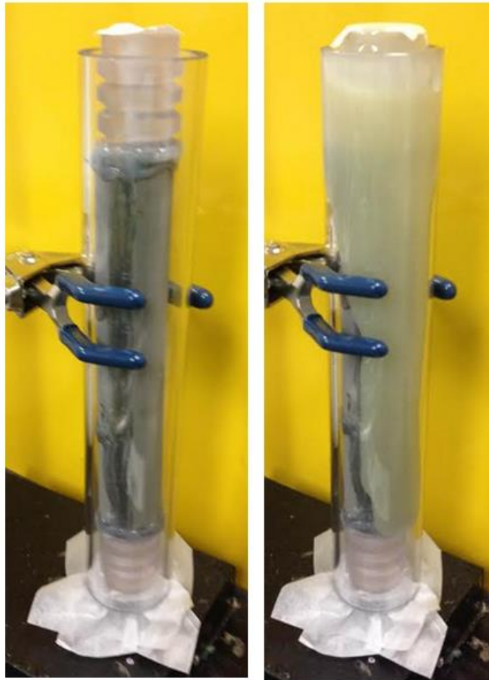
Figure 100: Cement fractured core placed into polycarbonate tube (left) and 24 hour epoxy poured into the space between the core and tube (right).
