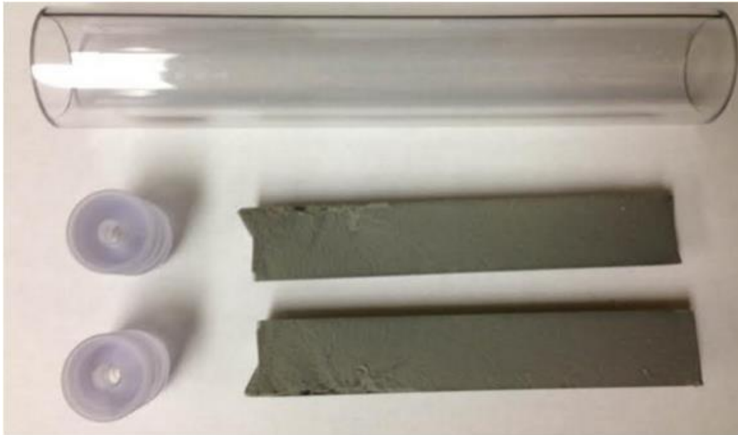
Figure 96: Materials required for epoxy core holder. Polycarbonate tube, fractured cement core, and core endcaps.
