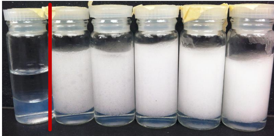
Figure 3.6 The effluent for the critical shear rate experiment performed in 1,000 micron beads. The critical shear rate was between 188 s -1 and 375 s -1 . The red line indicates the critical shear rate window. Nanoparticle dispersion (3 wt% NaCl, 2 wt% Nyacol DP 9711) and mineral oil co-injected at 1:1 phase ratio.
