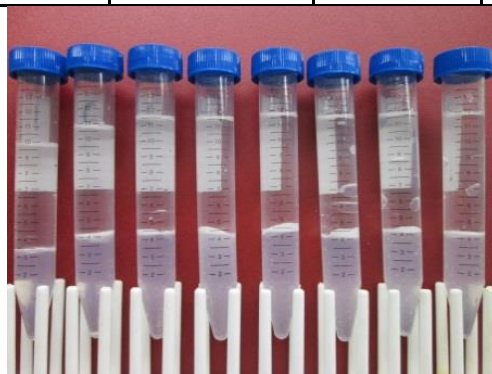
Figure 4.13 Experimental conditions and effluent from Beadpack Experiment 11. Only the constituent phases from the broken emulsion were produced for the entire duration of the experiment.
