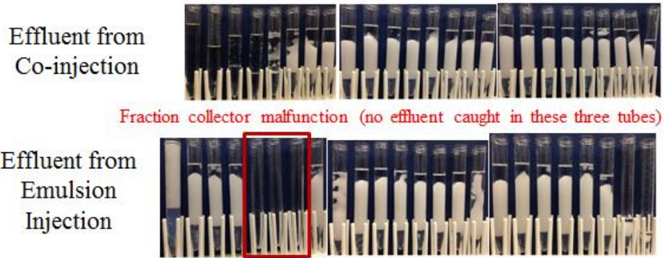
Figure 5.30 The effluent from the co-injection and the emulsion injection in Core O. Each tube contains 12 mL or 0.29 PV.
