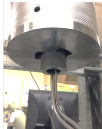
Core Holder with bottom three prong end piece
