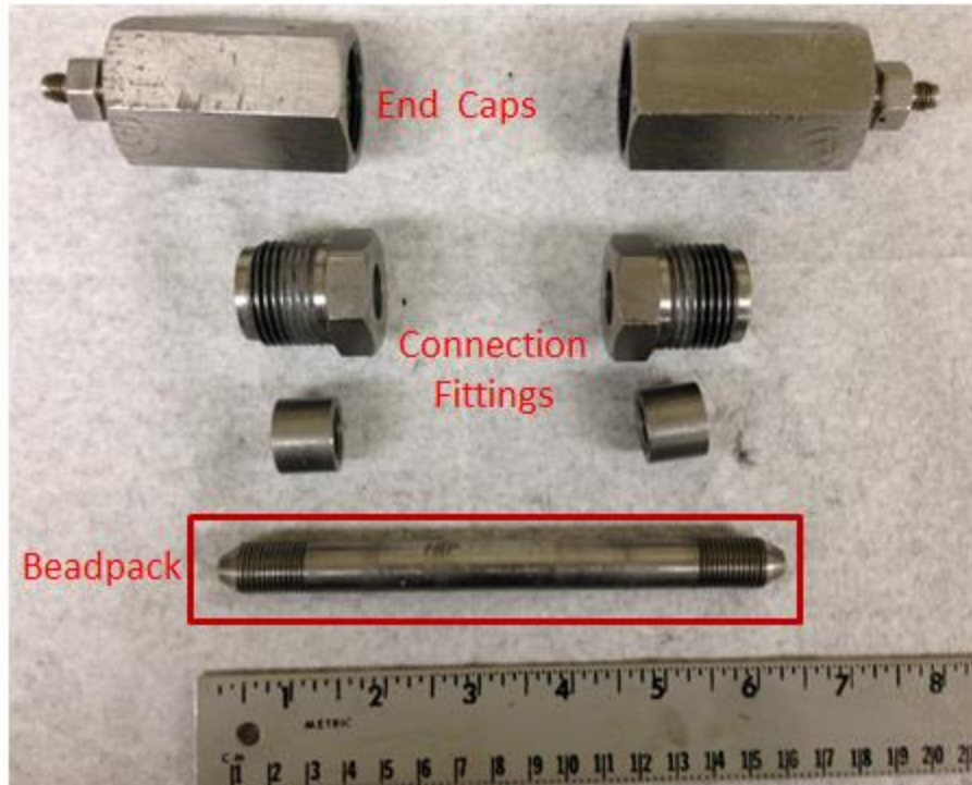
Figure A.6 The beadpack components including the connection fittings and end caps.
