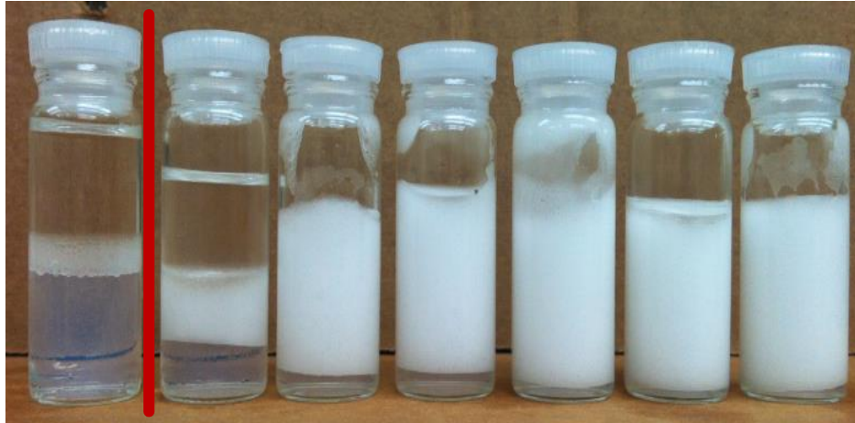
Figure 3.4 The effluent for the critical shear rate experiment performed in 275 micron beads. The critical shear rate was between 341 s -1 and 511 s -1 . The red line indicates the critical shear rate window. Nanoparticle dispersion (3 wt% NaCl, 2 wt% Nyacol DP 9711) and mineral oil co-injected at 1:1 phase ratio.
