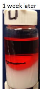
Figure 5.46 The octane emulsion and octane vial that was left undisturbed for a week.
