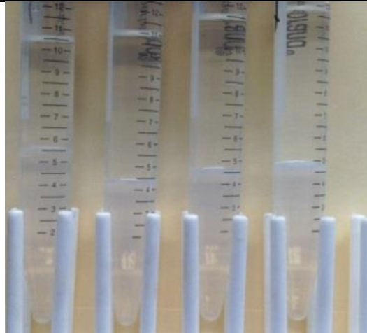
Figure 4.7 Experimental conditions and effluent from Experiment 5. Only the constituent phases from the broken emulsion were produced for the entire duration of the experiment.
