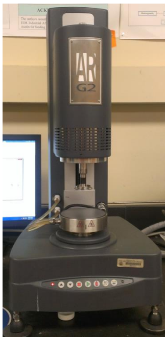
Figure A.1 Photo of AR-G2 magnetic bearing rheometer used to measure fluid viscosities.
