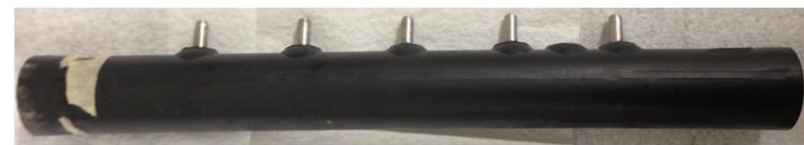
Figure A.11 Example of the Boise and Berea sandstone cores used in this thesis (top). The cores were placed into the rubber sleeve pictured (bottom). The rubber sleeve with pressure taps was housed in the core holder.
