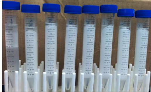
Figure 4.12 Experimental conditions and effluent from Beadpack Experiment 10. Only the constituent phases from the broken emulsion were produced for the first 9 pore volumes but stable emulsion along with small volumes of oil and aqueous phases from coalesced emulsion was produced for the remainder of the experiment
