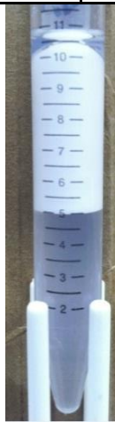
Figure 4.6 Experimental conditions and effluent from Beadpack Experiment 4. Stable emulsion was produced in the effluent. Nevertheless a small amount of oil phase and aqueous phase were also produced (see top of sample tube) indicating a moderate degree of coalescence also occurred. Approximately 2 to 3 mL of aqueous phase contained in the effluent was from dead volume in the effluent line (see text).
