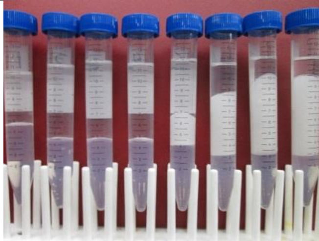
Figure 4.8 Experimental conditions and effluent from Beadpack Experiment 6. Only the constituent phases from the broken emulsion were produced for the first 45 pore volumes. Stable emulsion was produced after 45 pore volumes of injection though coalesced phases also continued to be produced along with the emulsion.
