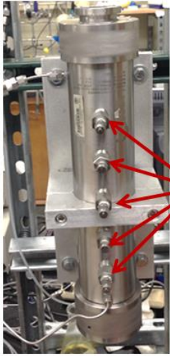
Hassler core holder without top and bottom fittings
