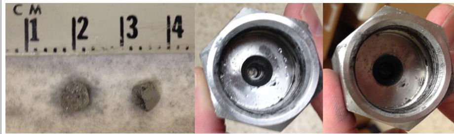
Figure A.7 The mesh pieces (left), end cap without mesh (middle), end cap with mesh (right).
