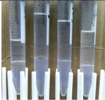
Figure 4.4 Experimental conditions and effluent from Beadpack Experiment 2. Only the constituent phases from the broken emulsion were produced for the entire duration of the experiment.
