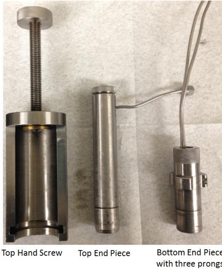
Figure A.9 The core holder fittings including the top hand screw (left), top end piece (middle), and the bottom end piece (right).
