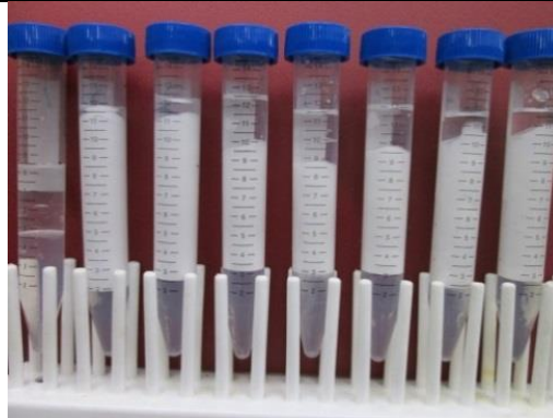
Figure 4.9 Experimental conditions and effluent from Beadpack Experiment 7. Only the constituent phases from the broken emulsion were produced for the first 8 pore volumes (leftmost sample) but stable emulsion was produced along with the coalesced phases (small fraction of oil and large fraction of aqueous phase in each sample tube) for the remainder of the experiment.
