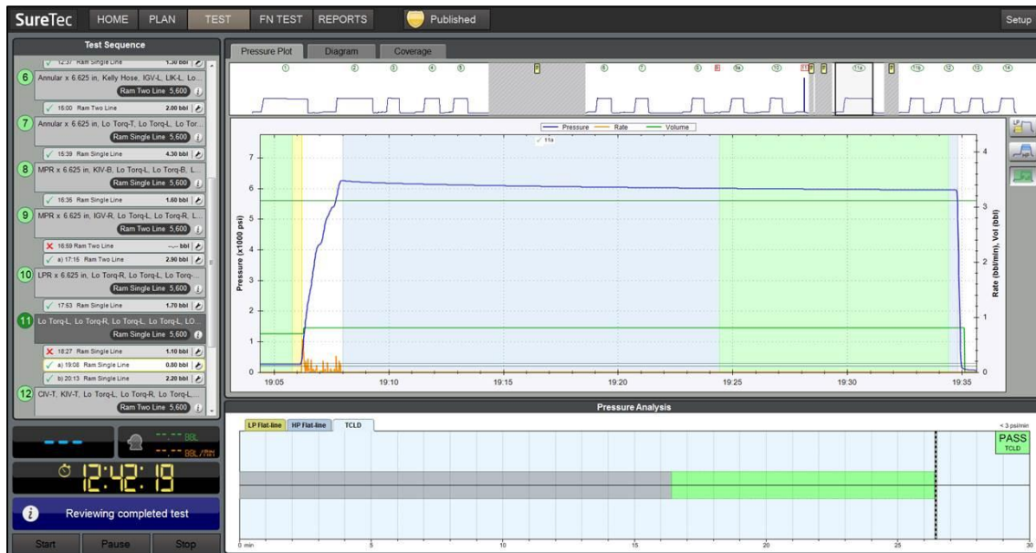
Figure 4.3: BOP component testing user interface. Displayed is the test in which an incorrect valve alignment according to the procedure was mistakenly tested. While passing the TLCDD test, it was noticed that the volume pumped was relatively lower than volumes in previous tests (left column). With the aid of the user display and digital real-time data, this mistake was identified and corrected, and the subsequent test with the correct alignment passed. (Courtesy of IPT Global)
