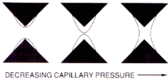
Figure 2-6 Schematic showing snap-off in a pore throat. (Rossen, 1995).
