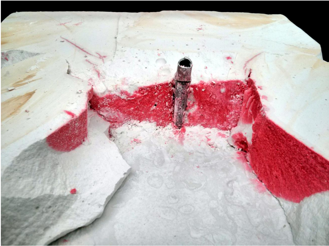
Figure 4.29: Side view photo of the block sample in test 6 shows hydraulic fracture intersecting collapsed orthogonal cavities, reorienting along them, and deflecting off of them.
