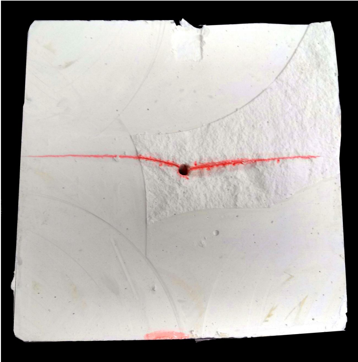
Figure 4.2: Top view photo of the middle section of the block sample in test 1 shows planar hydraulic fracture in red dye
