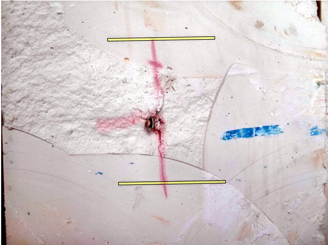
Figure 4.11: Top view photo of the middle section of the block sample in test 3 shows hydraulic fracture (in red dye) planar crossing of embedded inclusions (in yellow shade)
