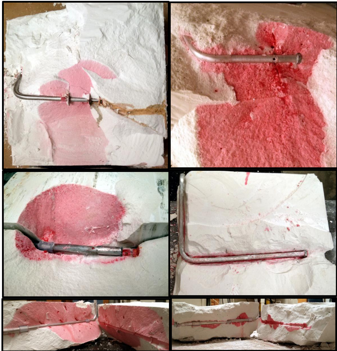
Figure 3.16: Examples of various horizontal wellbore designs attempted in multiple tests that had unsuccessful outcomes due to the observed tendency of such testing set up to generate longitudinal hydraulic fractures instead of the requisite transverse fractures.
