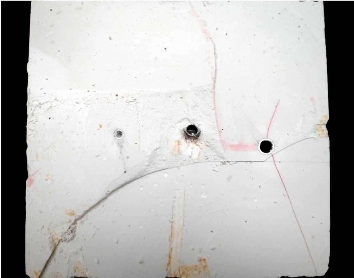
Figure 4.47: Bottom view photo of the middle section of the block sample in test 10 shows three perforation clusters (black holes) with a small hydraulic fracture propagating from the middle cluster (invisible in this photo) and another hydraulic fracture (in red dye) propagating from the third cluster on the far right with outwards curvature (note that injection flow was from left to right and the first cluster on the far left was plugged due to experimental difficulties)
