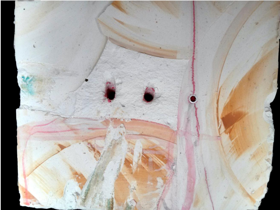
Figure 4.43: Top view photo of the middle section of the block sample in test 9 shows three perforation clusters (black holes) with a hydraulic fracture (in red dye) propagating from the first perforation cluster on the right with minor outwards curvature (note that injection flow direction was from right to left)
