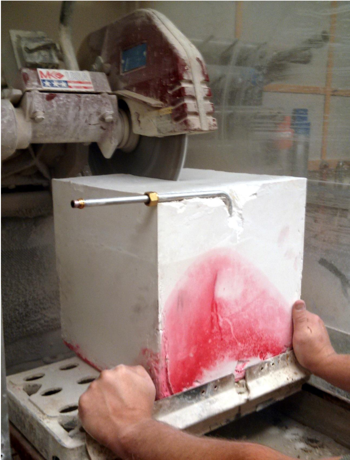
Figure 3.11: The core saw with lapidary diamond blade used to cut-open the hydraulic-fracture tested samples
