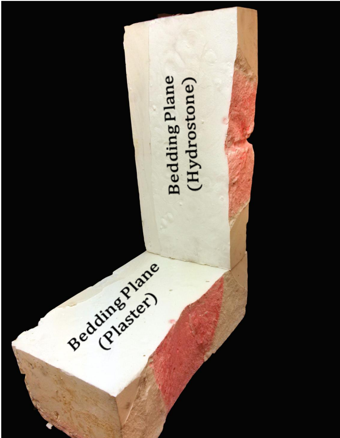
Figure 4.14: Side view photo of the block sample in test 3 shows hydraulic fracture (in red dye) planar crossing of a bedding plane without fluid leakage along the bedding-plane interface
