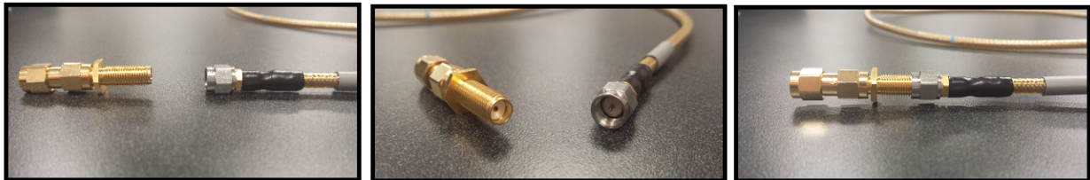
Figure 3.5 shows how the previous assembly in figure 3.3 connects to the coax cable.
