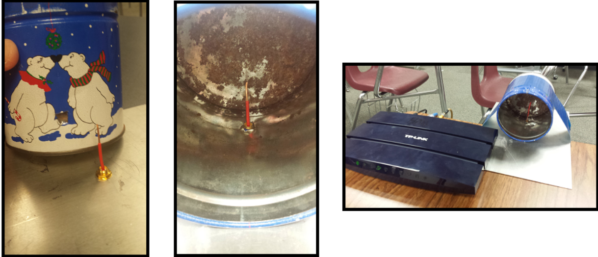
Figure 3.11: assemble can with router setup
