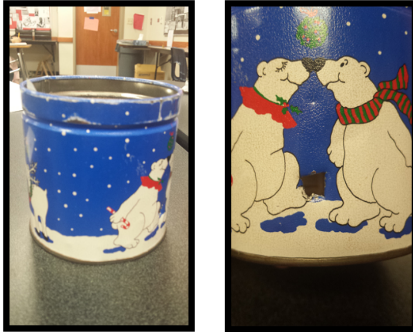
Figure 3.8: Pictured above is the can used for the antenna.
