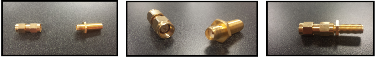
Figure 3.4: picture 1 shows RPSMA on left and female-to-female SMA connector on right in each picture
