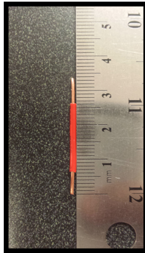
Figure 3.9: Monopole antenna used for the cantenna
