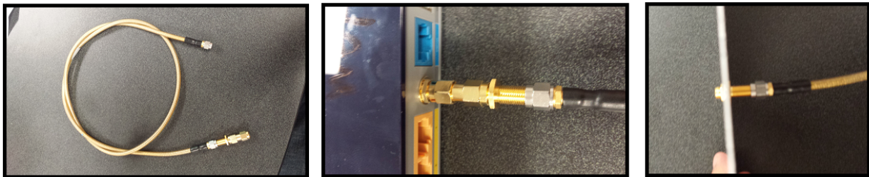
Figure 3.6: coax cable on left, RPSMA end connected to modem in middle, coax cable connected to mounting plate on right.
