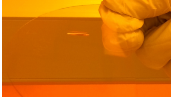
Figure 14: Flow and resistance of water drop on anisotropic imprinted pattern.
