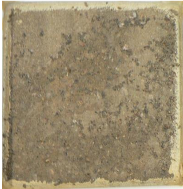
Figure 17. CAC-3 samples after 50 cycles according to ASTM C 672.
