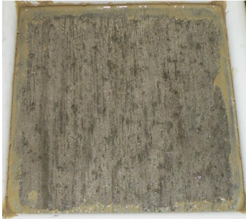
Figure 84. Salt scaling (ASTM C 672) specimen of material CAC-3 after 5 cycles.
