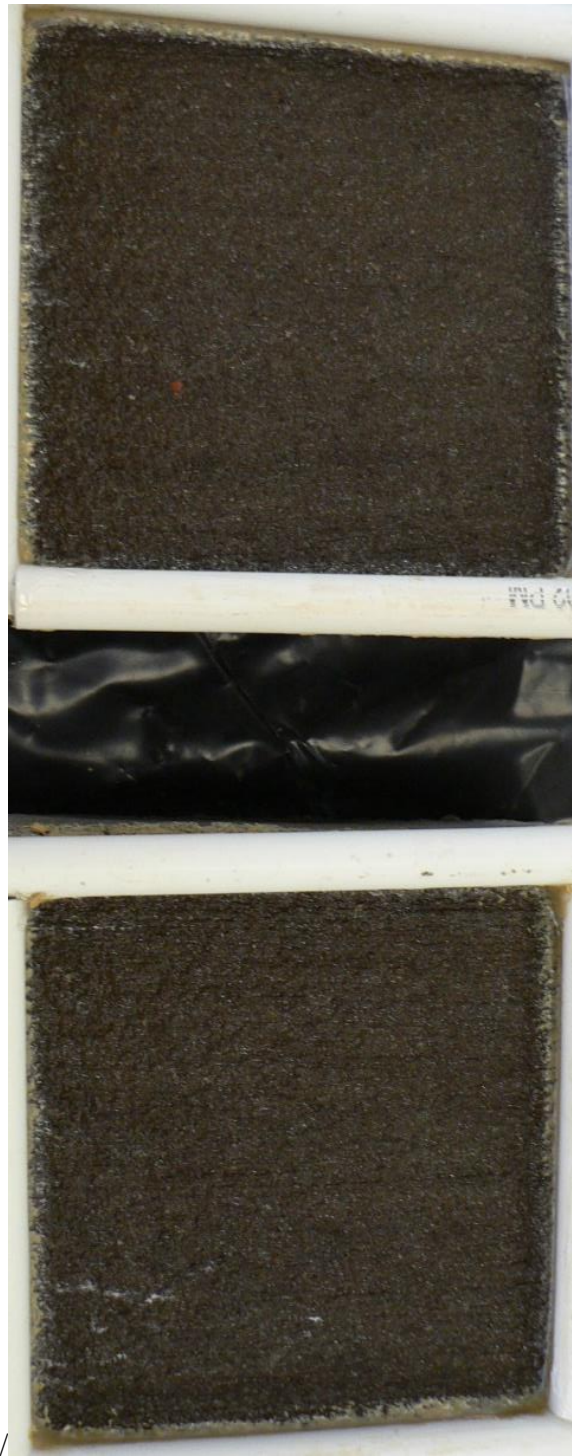
Figure 81. Salt scaling (ASTM C 672) specimen of material CAC-1 after 5 cycles.
