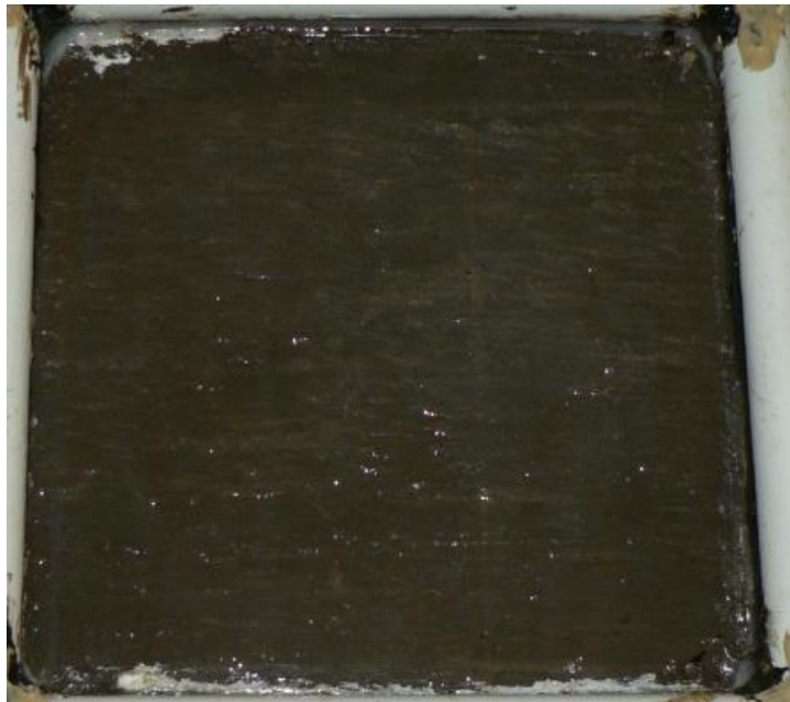
Figure 86. Salt scaling (ASTM C 672) specimen of material P-2 after 10 cycles.
