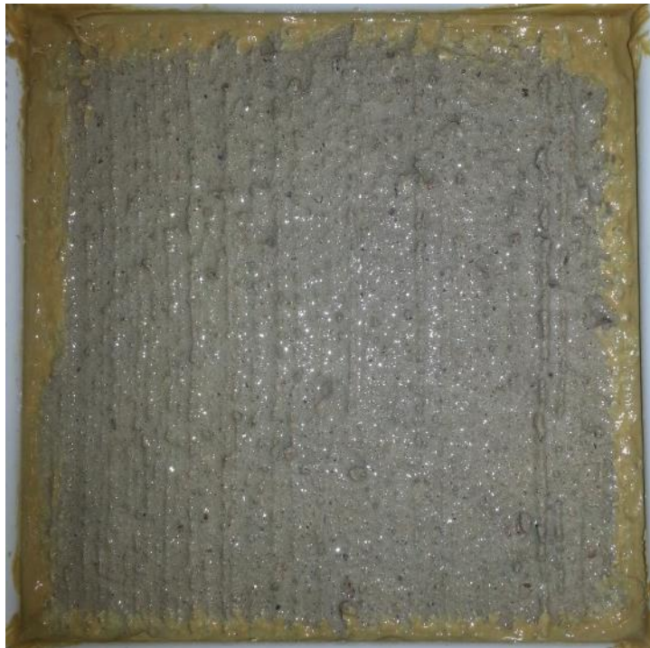
Figure 91. Salt scaling (ASTM C 672) specimen of material CSA-2 after 10 cycles.
