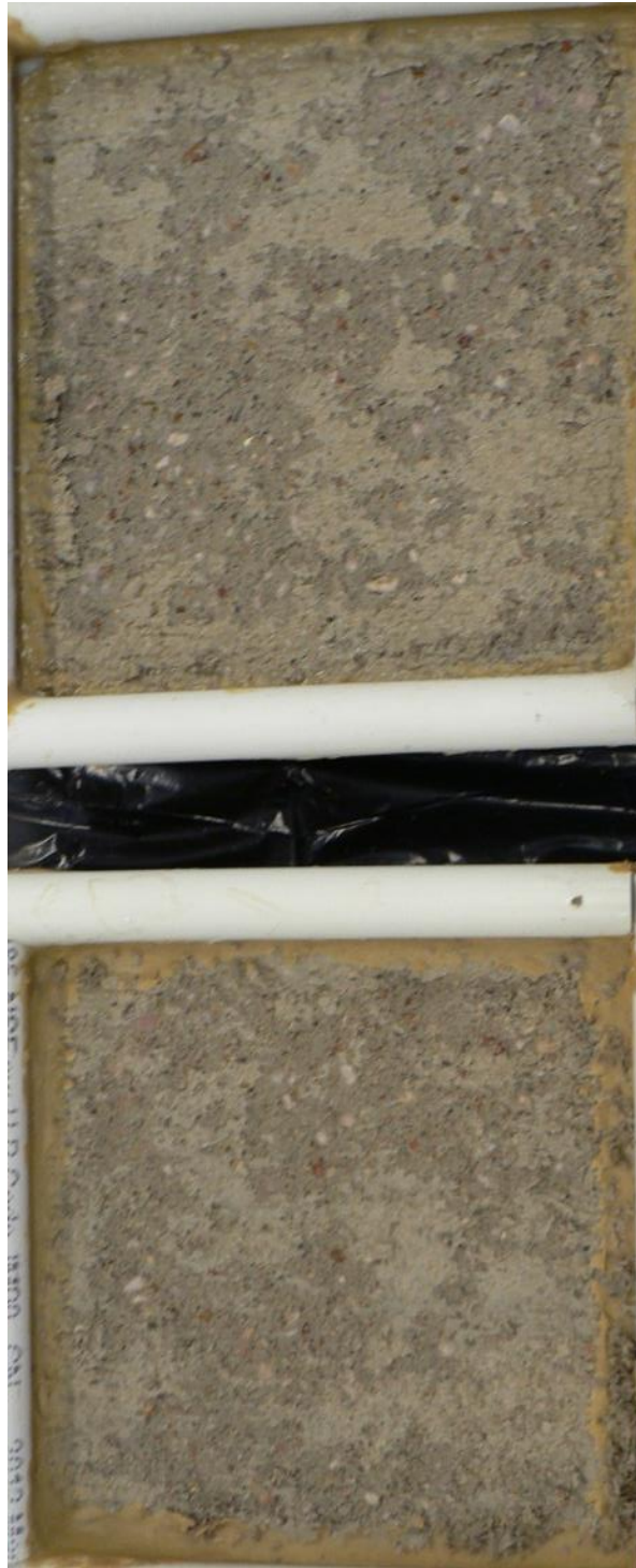
Figure 90. Salt scaling (ASTM C 672) specimen of material CSA-Latex after 10 cycles.
