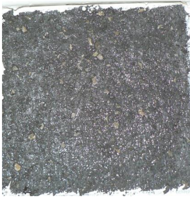
Figure 10. P-3 samples after 50 cycles according to ASTM C 672.
