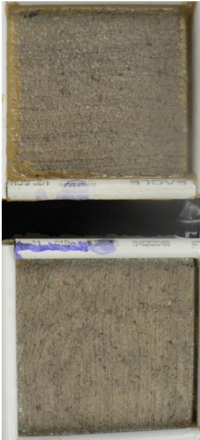
Figure 69. Salt scaling (ASTM C 672) specimen for material CSA-1 after 0 cycles.
