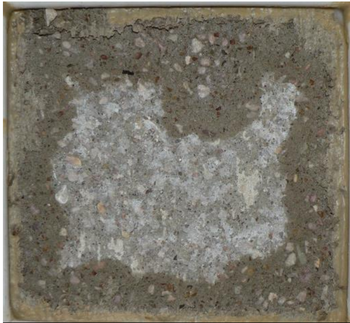
Figure 113. Salt scaling (ASTM C 672) specimen of material CSA-Latex after 25 cycles.
