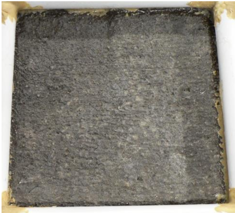
Figure 73. Salt scaling (ASTM C 672) specimen for material CAC-Latex after 0 cycles.
