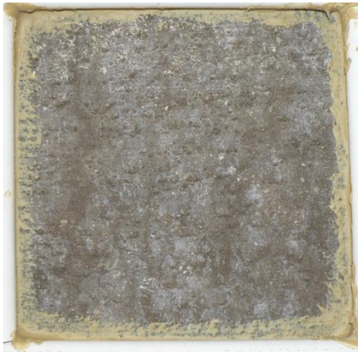
Figure 76. Salt scaling (ASTM C 672) specimen for material CAC-2 after 0 cycles.
