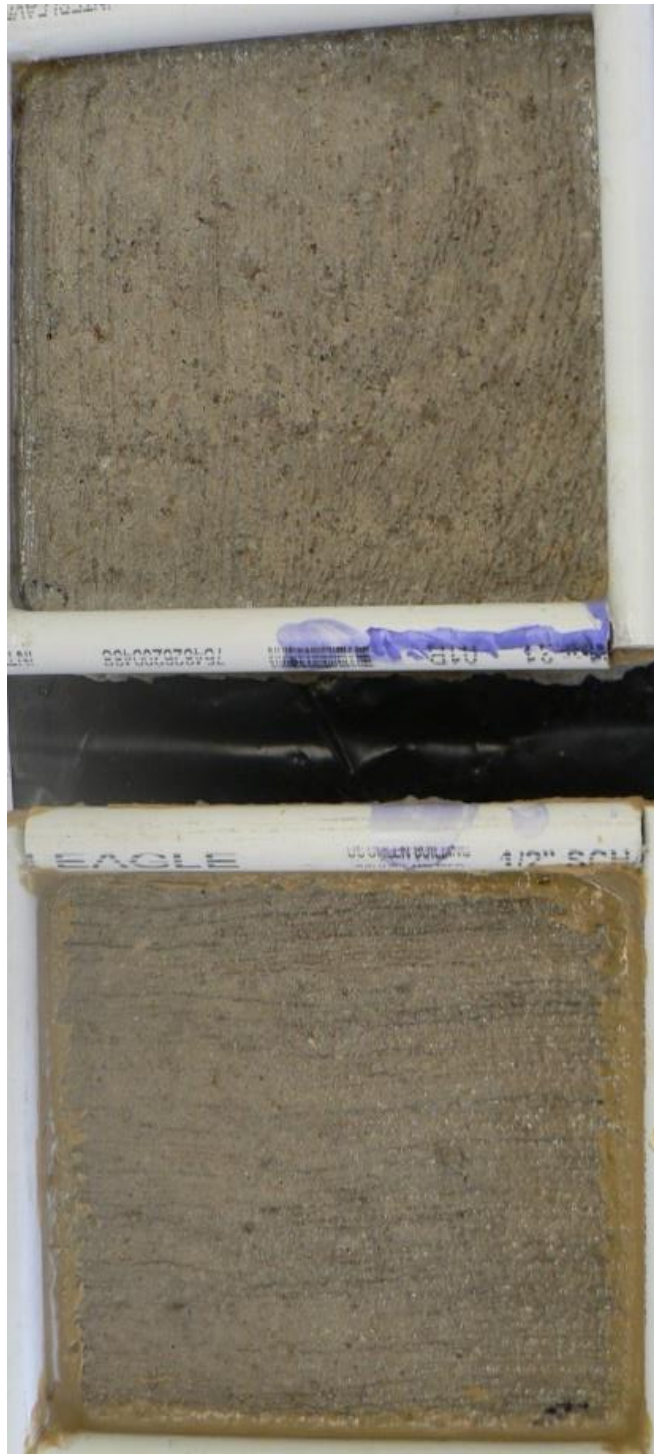
Figure 79. Salt scaling (ASTM C 672) specimen of material CSA-1 after 5 cycles.
