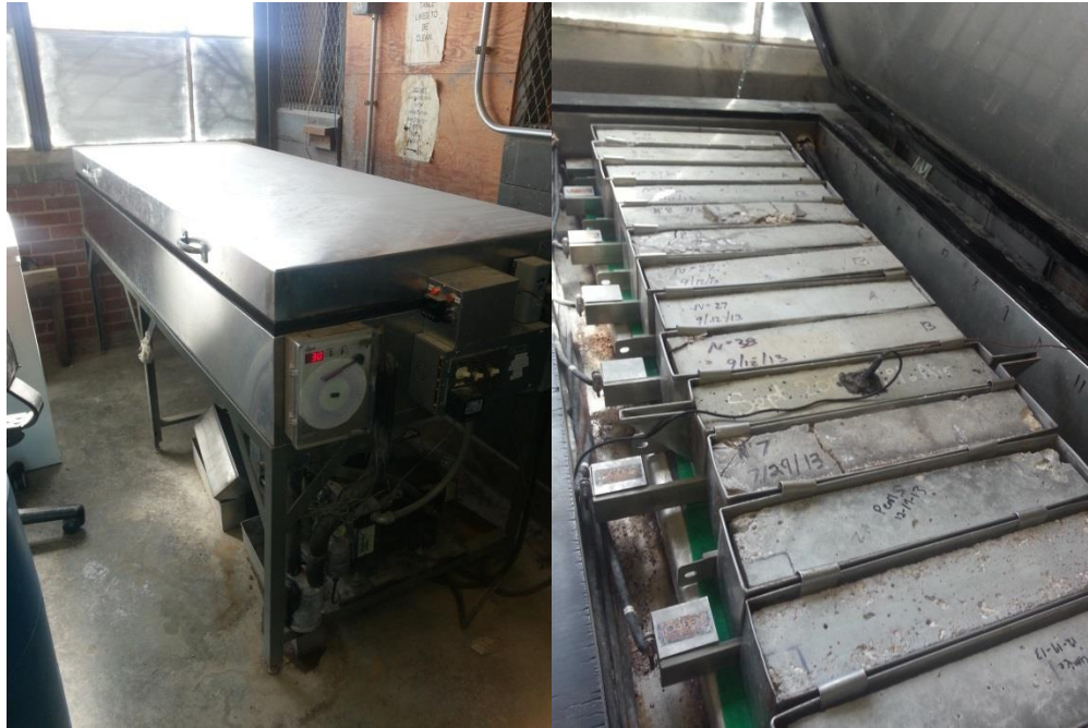
Figure 22. Specimens for ASTM C 666 in the freezing-and-thawing chamber.
