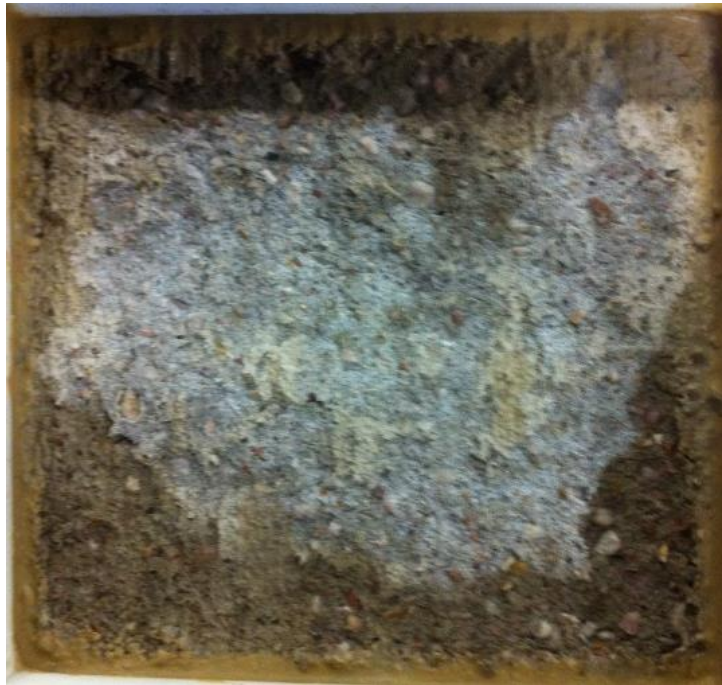
Figure 102. Salt scaling (ASTM C 672) specimen of material CSA-Latex after 15 cycles.
