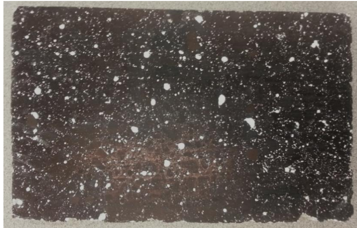
Figure 5. Example of final concrete specimen ready for use in RapidAir system.
