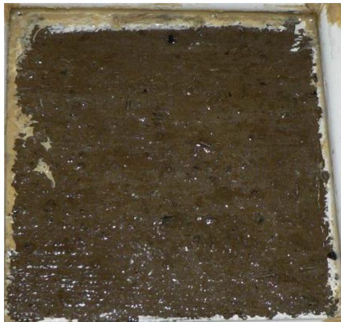
Figure 11. P-AAFA samples after 50 cycles according to ASTM C 672.
