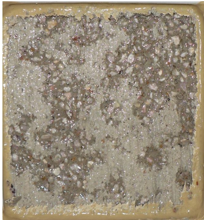
Figure 19. CSA-1 samples after 25 cycles (50 unavailable) according to ASTM C 672.
