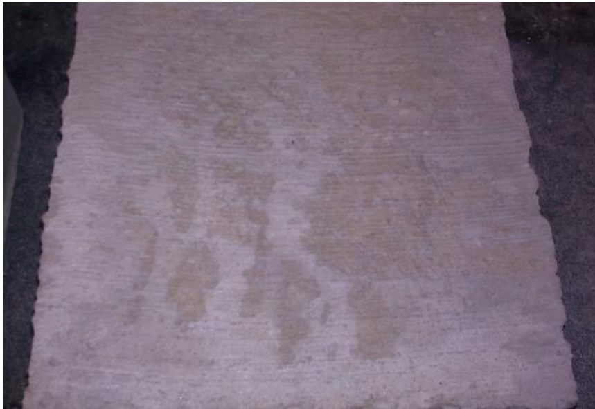
Figure 66. Salt scaling (ASTM C 672) specimen for material P-1 after 0 cycles.
