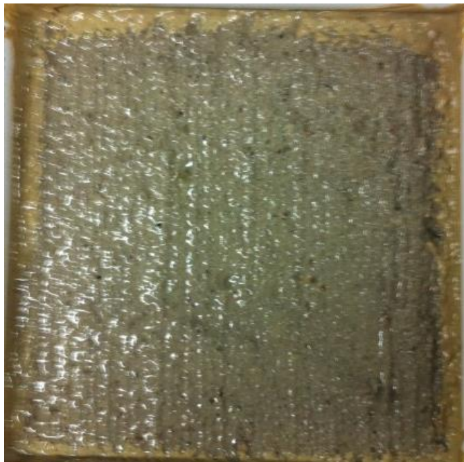
Figure 125. CSA-2 samples after 50 cycles according to ASTM C 672.
