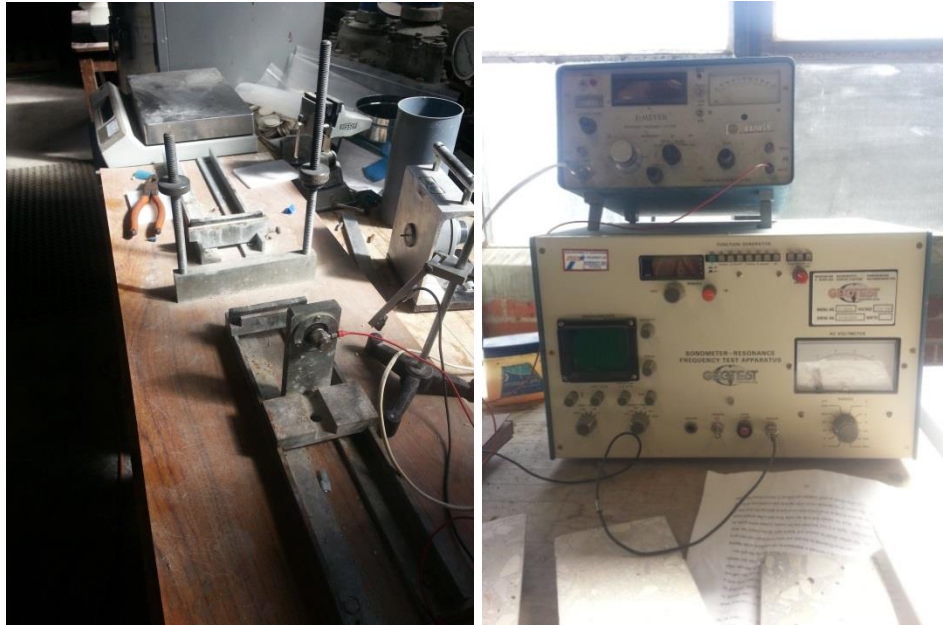
Figure 21. Equipment for testing the fundamental transverse frequency of concrete samples according to ASTM C 666.
