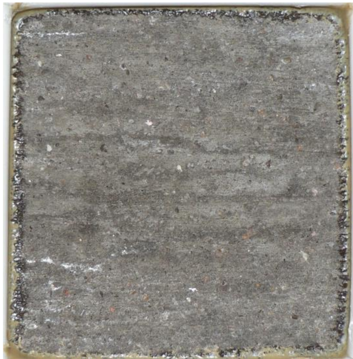
Figure 115. Salt scaling (ASTM C 672) specimen of material CAC-1 after 25 cycles.
