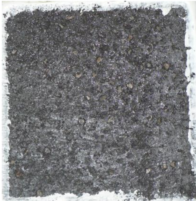
Figure 123. P-3 samples after 50 cycles according to ASTM C 672.
