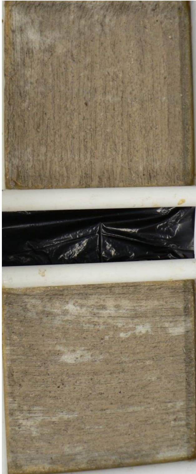
Figure 95. Salt scaling (ASTM C 672) specimen of material CSA-3 after 10 cycles.
