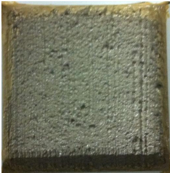
Figure 114. Salt scaling (ASTM C 672) specimen of material CSA-2 after 25 cycles.
