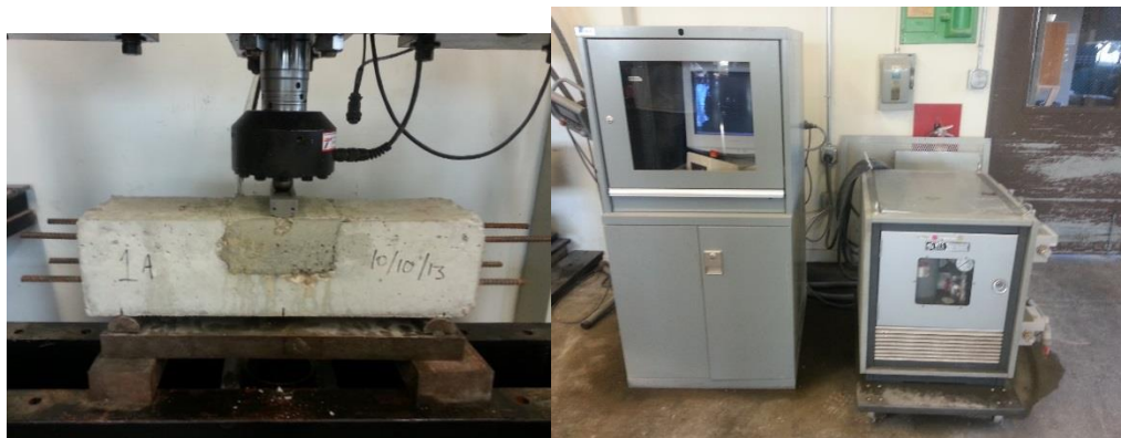
Figure 56. Loading fatigue-corrosion beams under repetitive loads using MTS loading machine.
