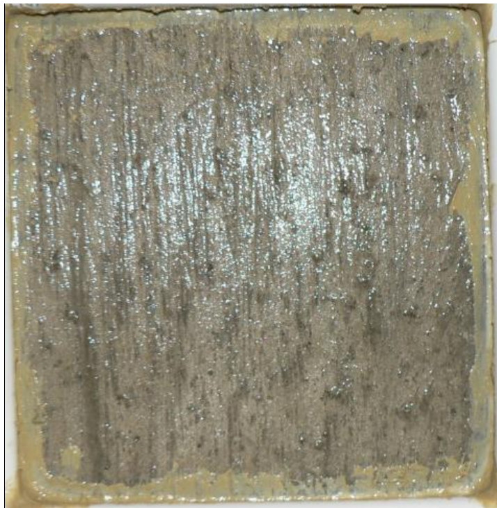
Figure 107. Salt scaling (ASTM C 672) specimen of material CAC-3 after 15 cycles.
