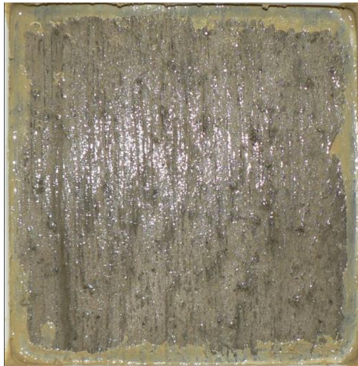
Figure 119. Salt scaling (ASTM C 672) specimen of material CAC-3 after 25 cycles.
