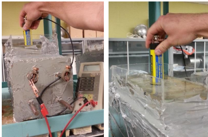
Figure 58. Measuring macrocell voltage of reinforcing steel using voltmeter and reference electrode .
