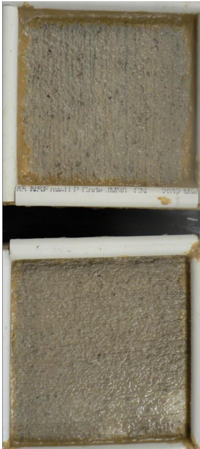
Figure 70. Salt scaling (ASTM C 672) specimen for material CSA-Latex after 0 cycles.
