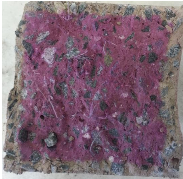
Figure 42. P-AAFA sample displaying carbonation depth at 11 months using Phenolphthalein PH indicator.
