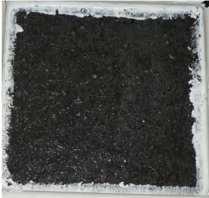
Figure 87. Salt scaling (ASTM C 672) specimen of material P-3 after 10 cycles.
