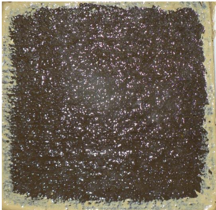
Figure 97. Salt scaling (ASTM C 672) specimen of material CAC-2 after 10 cycles.
