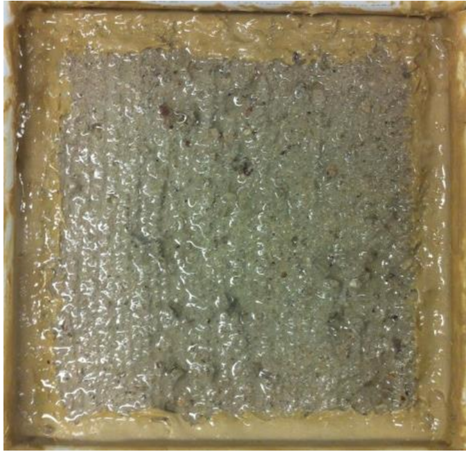
Figure 12. CSA-2 samples after 50 cycles according to ASTM C 672.
