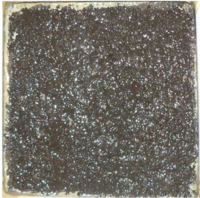
Figure 14. CAC-Latex samples after 50 cycles according to ASTM C 672.
