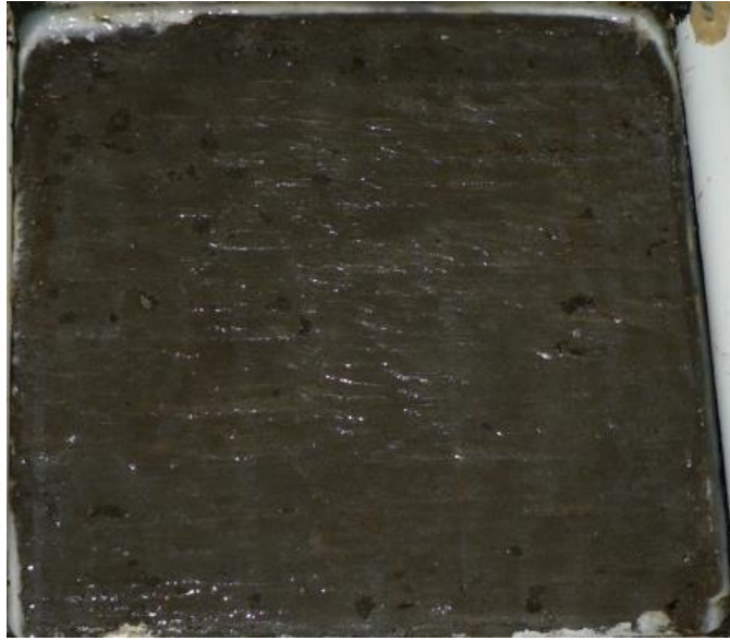
Figure 122. P-2 samples after 50 cycles according to ASTM C 672.
