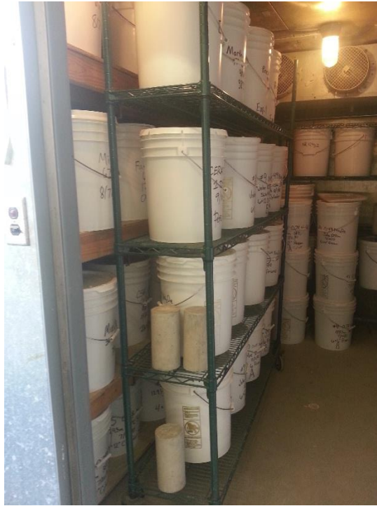
Figure 26. Temperature and humidity controlled room for ASTM C 1293 testing.
