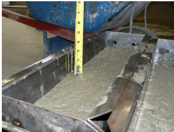
Figure 53. Casting the bottom layer of fatigue-corrosion beams.
