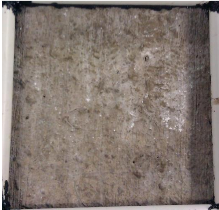
Figure 68. Salt scaling (ASTM C 672) specimen for material P-AAFA after 0 cycles.
