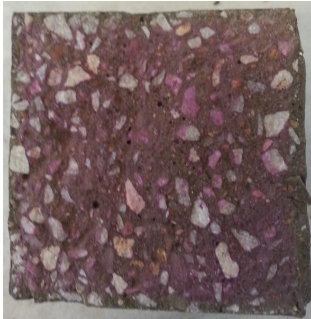
Figure 47. CAC-1 sample displaying carbonation depth at 11 months using Phenolphthalein PH indicator.
