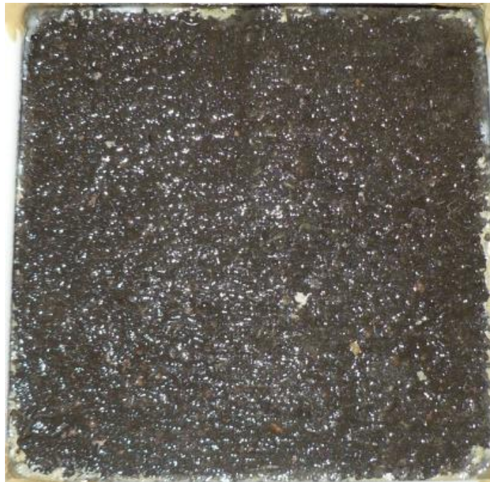
Figure 127. CAC-1 samples after 50 cycles according to ASTM C 672.
