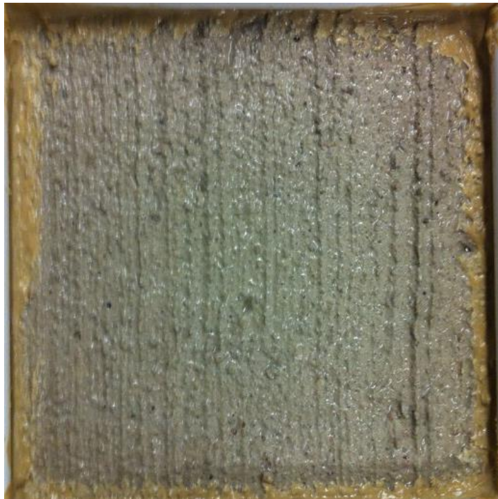
Figure 103. Salt scaling (ASTM C 672) specimen of material CSA-2 after 15 cycles.
