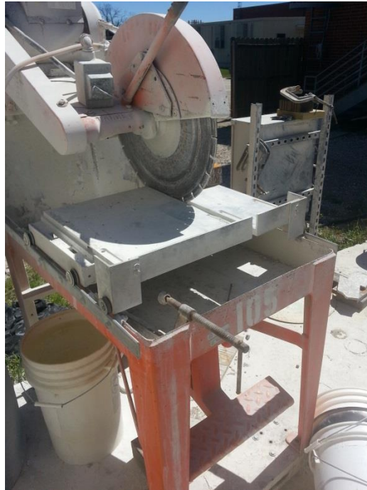
Figure 2. Wet saw used for cutting hardened air specimens.
