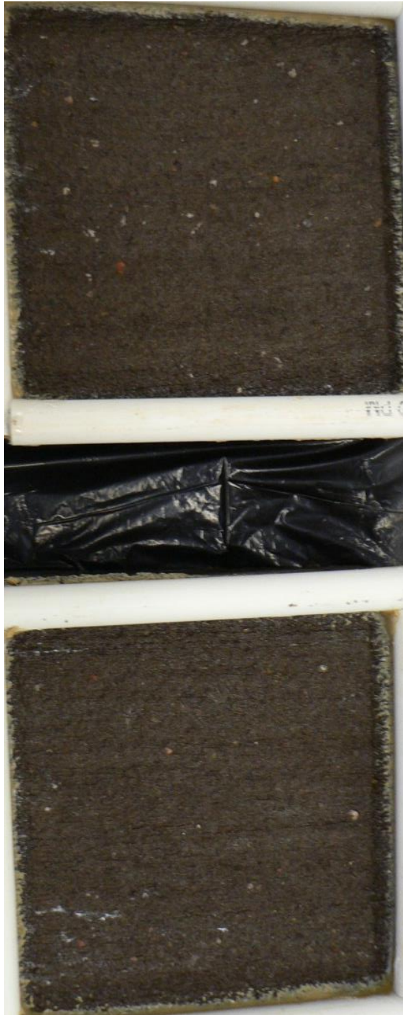
Figure 92. Salt scaling (ASTM C 672) specimen of material CAC-1 after 10 cycles.
