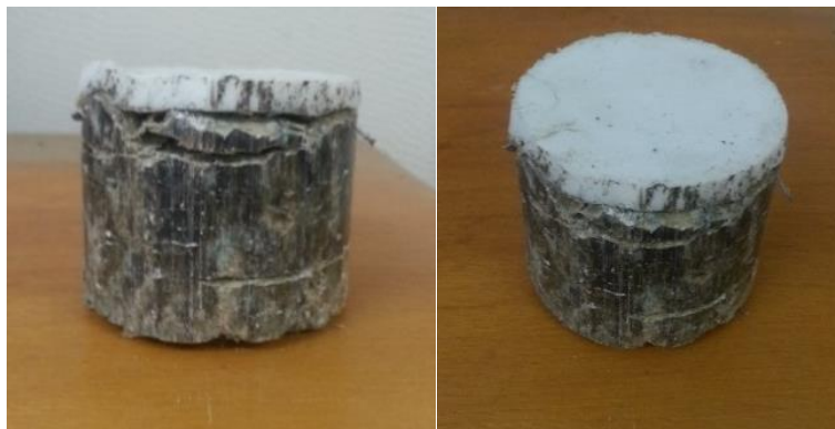
Figure 29. P-AAFA samples after attempting pore solution extraction via pore press.
