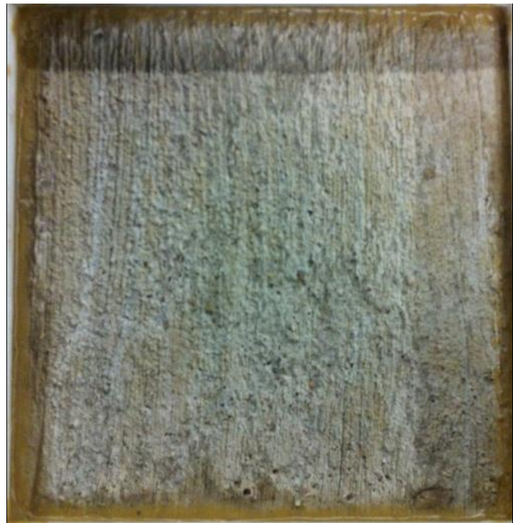
Figure 106. Salt scaling (ASTM C 672) specimen of material CSA-3 after 15 cycles.
