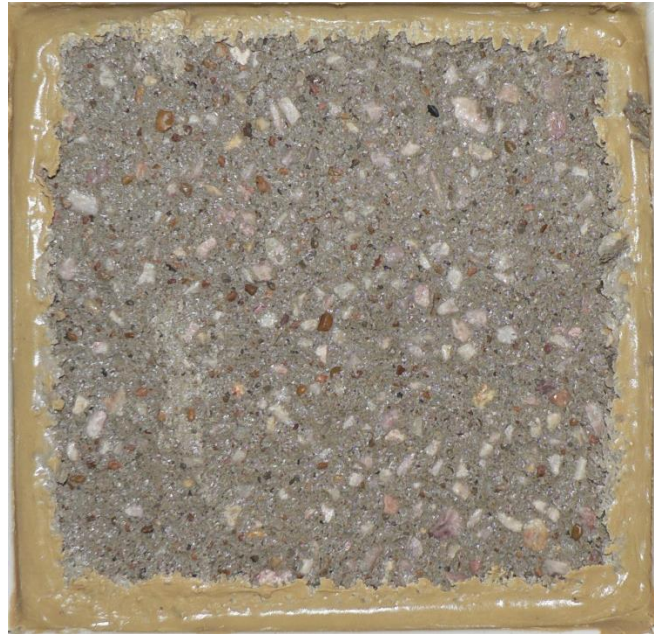
Figure 20. CSA-Latex samples after 25 cycles (50 unavailable) according to ASTM C 672.
