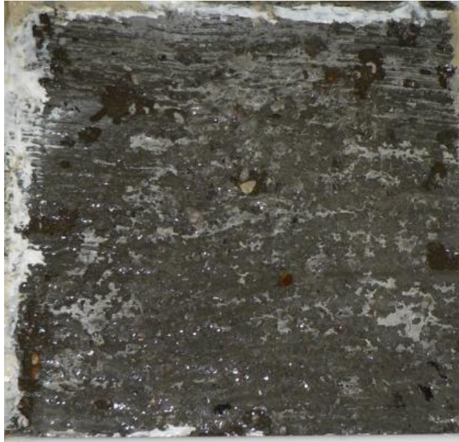
Figure 128. CAC-Latex samples after 50 cycles according to ASTM C 672.
