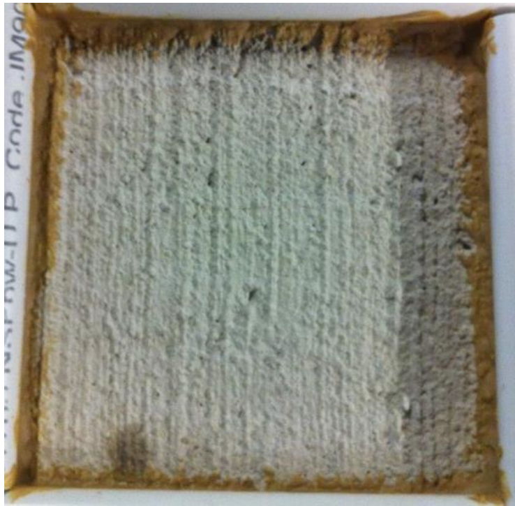
Figure 71. Salt scaling (ASTM C 672) specimen for material CSA-2 after 0 cycles.
