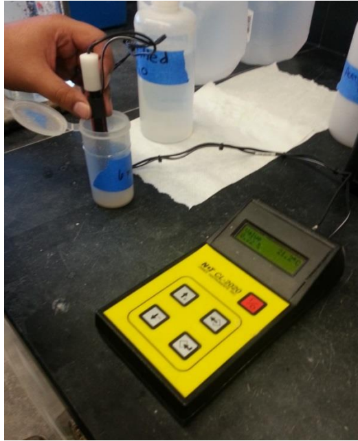
Figure 49. Measuring chloride content using James Instruments, Inc. CL-2020 chlorimeter.
