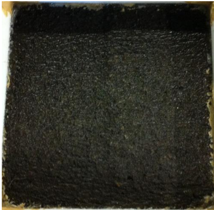
Figure 93. Salt scaling (ASTM C 672) specimen of material CAC-Latex after 10 cycles.
