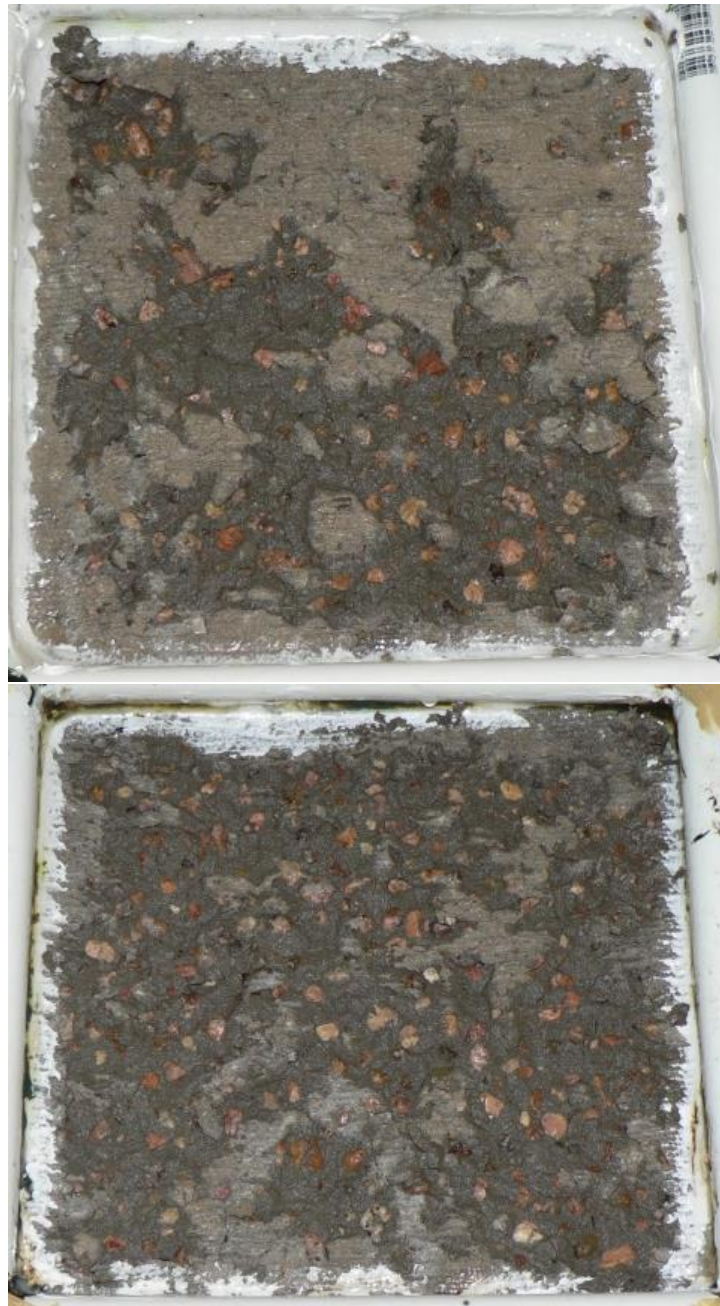
Figure 77. Salt scaling (ASTM C 672) specimen for material P-1 after 5 cycles.
