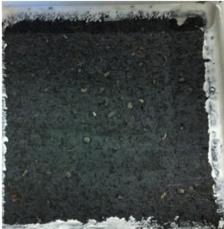
Figure 99. Salt scaling (ASTM C 672) specimen of material P-3 after 15 cycles.
