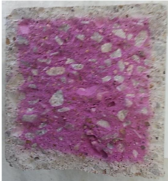
Figure 43. CSA-1 sample displaying carbonation depth at 11 months using Phenolphthalein PH indicator.
