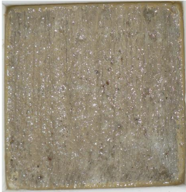
Figure 16. CSA-3 samples after 50 cycles according to ASTM C 672.
