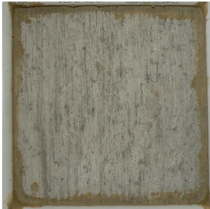
Figure 75. Salt scaling (ASTM C 672) specimen for material CAC-3 after 0 cycles.
