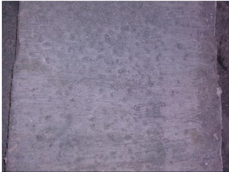
Figure 67. Salt scaling (ASTM C 672) specimen for material P-3 after 0 cycles.
