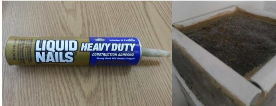
Figure 7. Liquid Nails adhesive and typical specimen used in ASTM C 672 testing.
