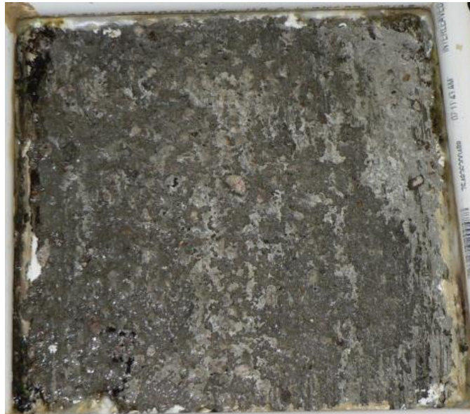
Figure 15. PC Type III samples after 50 cycles according to ASTM C 672.
