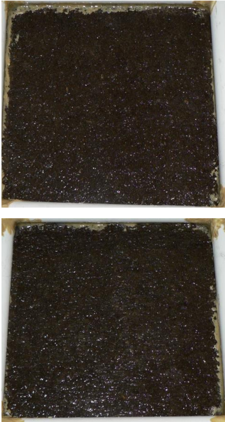
Figure 82. Salt scaling (ASTM C 672) specimen of material CAC-Latex after 5 cycles.
