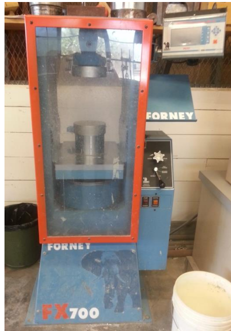
Figure 28. Forney FX700 compressive testing machine.
