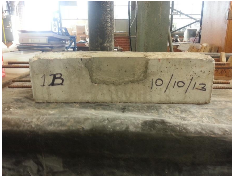
Figure 55. Example of final fatigue-corrosion beam and inset repair material.
