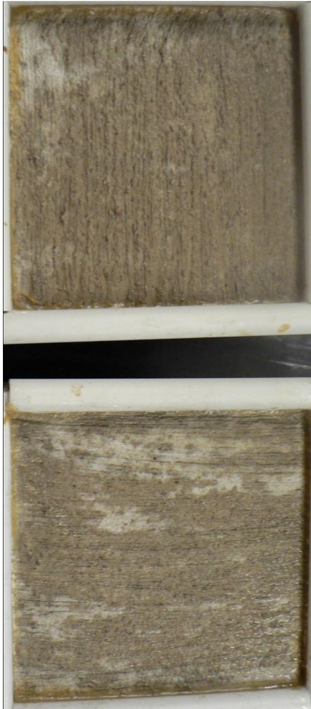
Figure 74. Salt scaling (ASTM C 672) specimen for material CSA-3 after 0 cycles.
