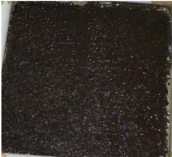
Figure 105. Salt scaling (ASTM C 672) specimen of material CAC-Latex after 15 cycles.
