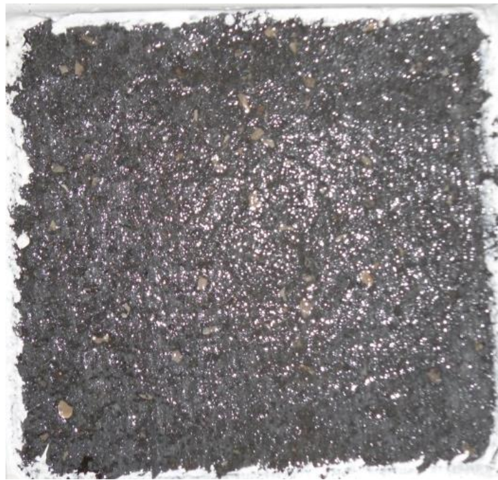
Figure 110. Salt scaling (ASTM C 672) specimen of material P-3 after 25 cycles.
