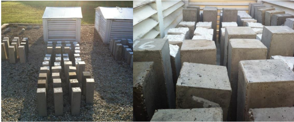
Figure 40. Test location of carbonation prisms.
