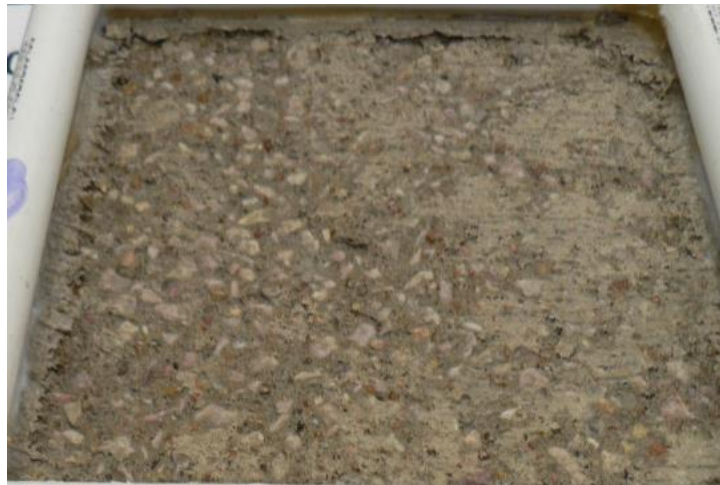
Figure 89. Salt scaling (ASTM C 672) specimen of material CSA-1 after 10 cycles.
