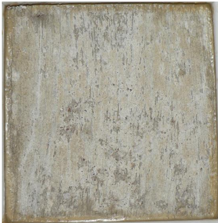
Figure 118. Salt scaling (ASTM C 672) specimen of material CSA-3 after 25 cycles.
