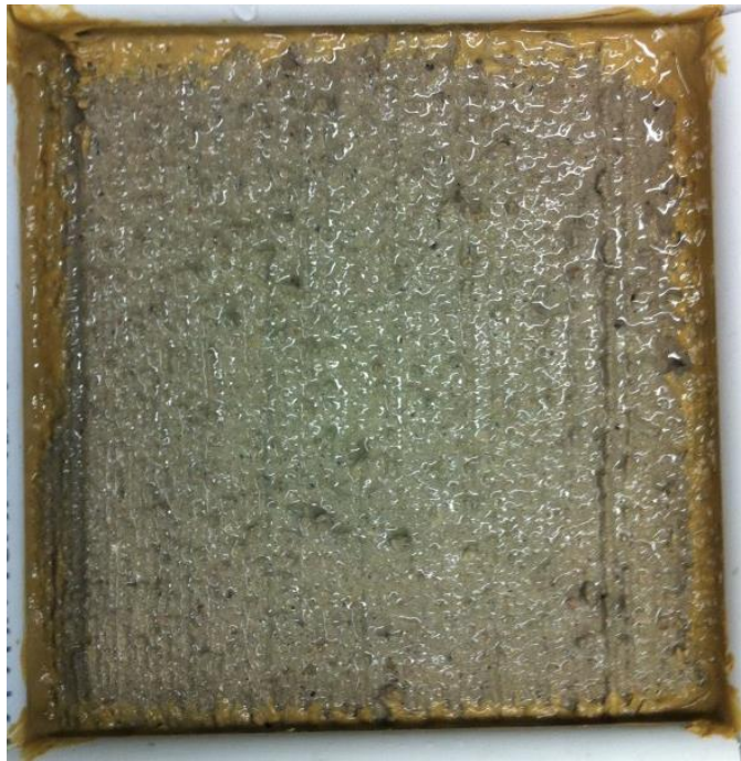
Figure 80. Salt scaling (ASTM C 672) specimen of material CSA-2 after 5 cycles.
