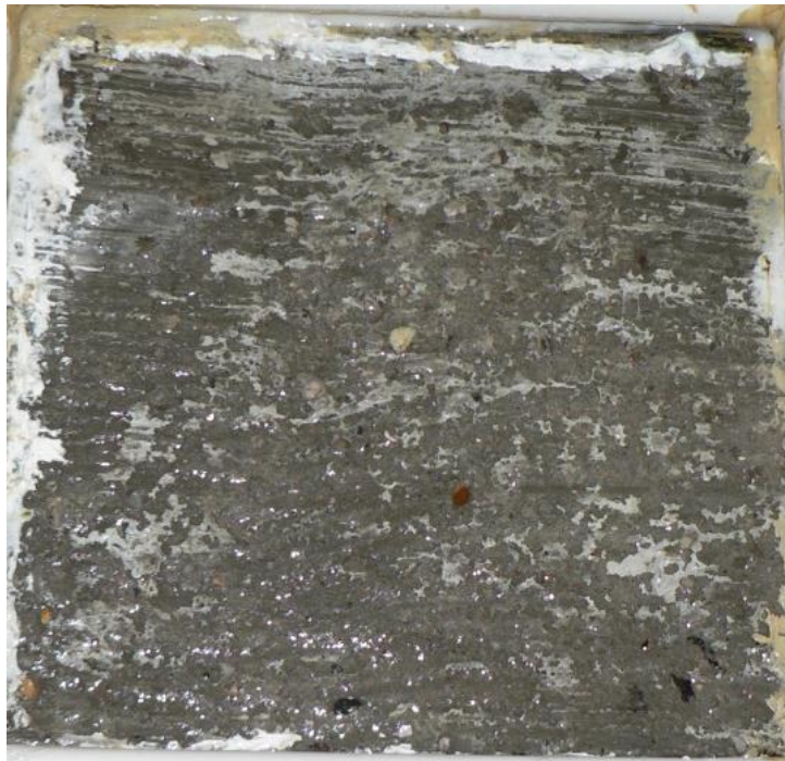
Figure 117. Salt scaling (ASTM C 672) specimen of material PC Type III after 25 cycles.
