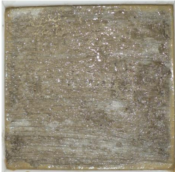
Figure 129. PC Type III samples after 50 cycles according to ASTM C 672.
