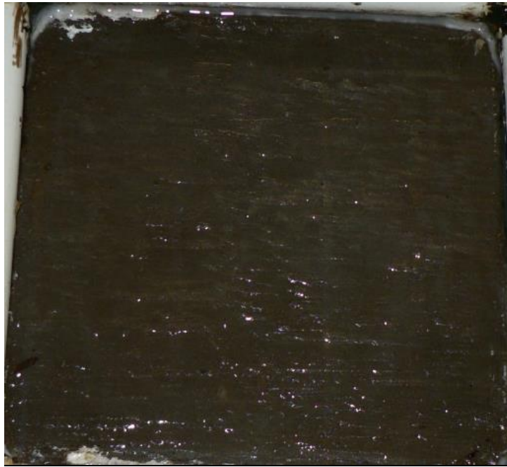
Figure 98. Salt scaling (ASTM C 672) specimen of material P-2 after 15 cycles.
