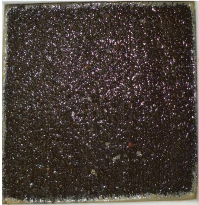
Figure 13. CAC-1 samples after 50 cycles according to ASTM C 672.
