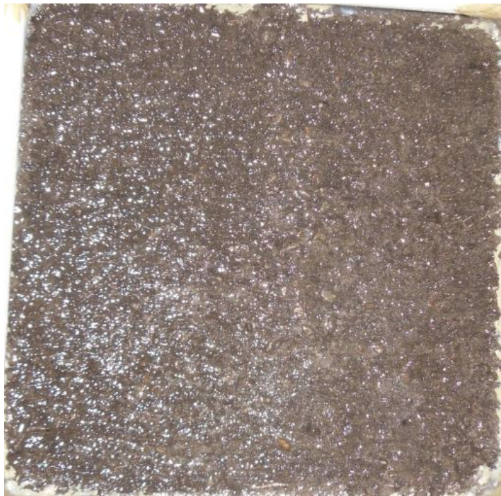
Figure 116. Salt scaling (ASTM C 672) specimen of material CAC-Latex after 25 cycles.
