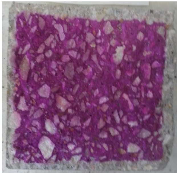
Figure 44. CAC-3 sample displaying carbonation depth at 11 months using Phenolphthalein PH indicator.
