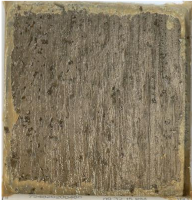
Figure 130. CAC-3 samples after 50 cycles according to ASTM C 672.
