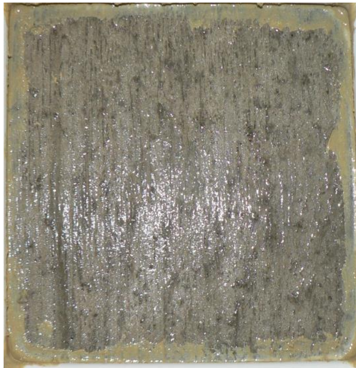
Figure 96. Salt scaling (ASTM C 672) specimen of material CAC-3 after 10 cycles.
