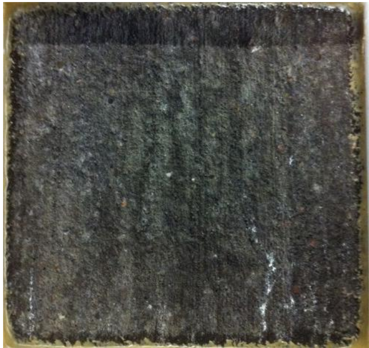
Figure 104. Salt scaling (ASTM C 672) specimen of material CAC-1 after 15 cycles.
