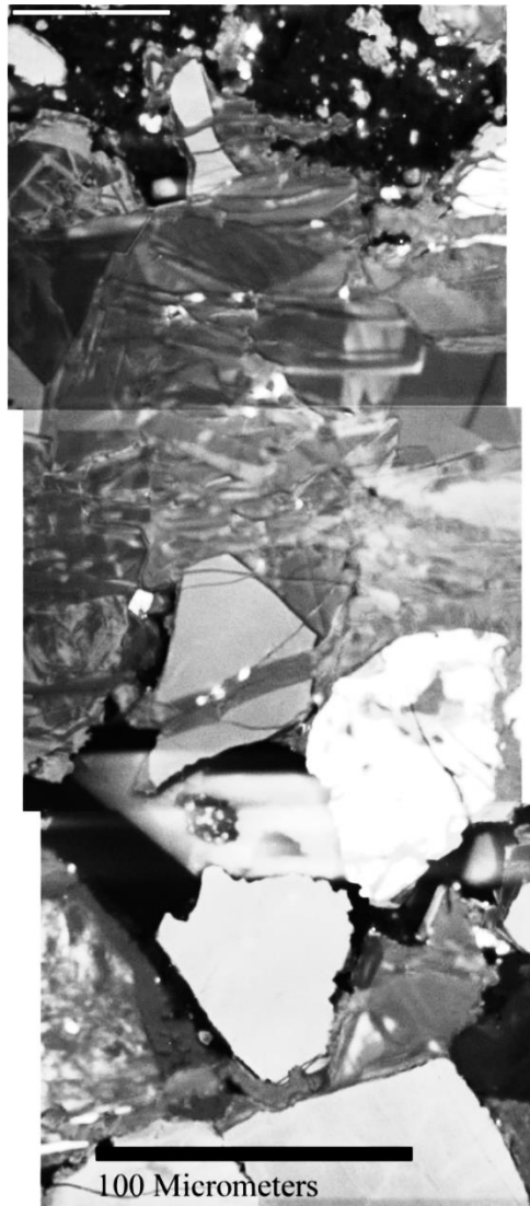
Figure B. 15: Panchromatic SEM-CL image of bridge 5. The blurriness around the white quartz grain at the bottom is an imaging artifact caused by high luminescence.
