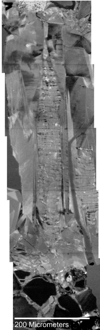
Figure B. 24: Panchromatic SEM-CL image of bridge 1 of fracture 1. A smaller partially crack-seal bridge can be observed to the right of bridge 1. The crack-seal texture covers most of the bridge but euhedral cement is present at the upper side; thin section cutting effect is suspected to be the reason.
