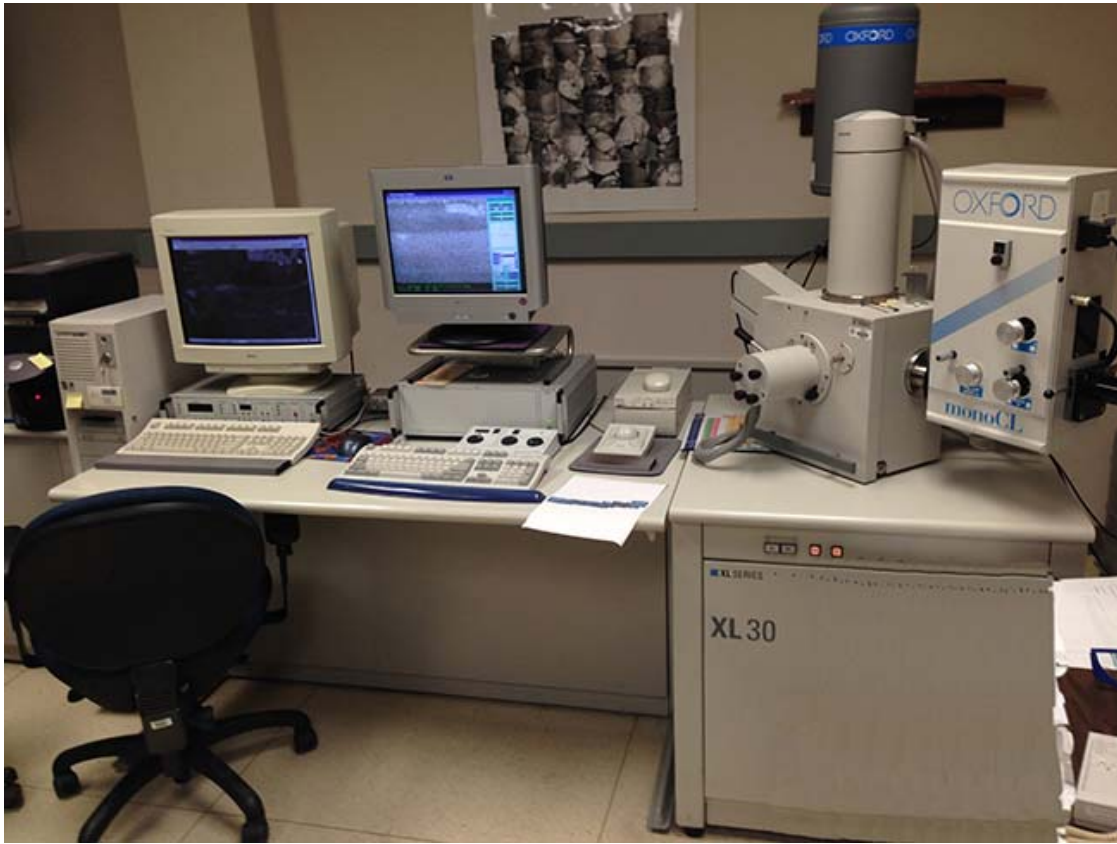
Figure 3.4: The scanning electron microscope system utilized in this study. The Oxford monoCL unit can be seen attached to the SEM chamber.
