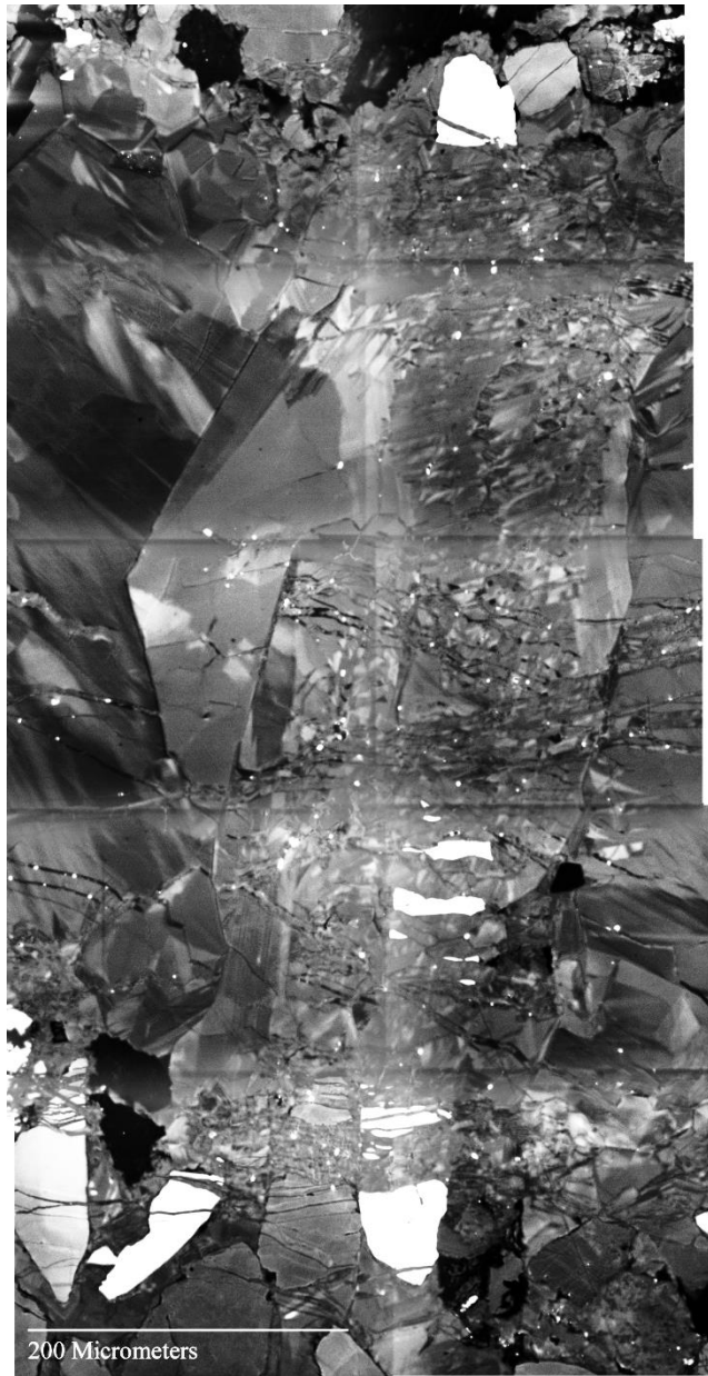
Figure B. 18: Panchromatic SEM-CL image of bridge 6. The fracture splits a white quartz grain with one half of the grain located in the upper fracture wall and the other in the lower fracture wall; some fragments are displaced within the crack-seal bridge. Late crack-seal can be observed cutting euohedral quartz cement on both sides of the bridge.
