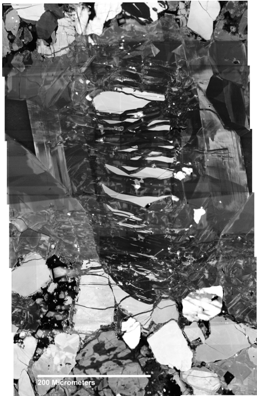
Figure B. 17: Panchromatic SEM-CL image of bridge 2. Two generations of fractures have affected the embedded quartz grain: older intragranular microfractures and younger crack-seal fracture increments that are responsible for the observed fragmentation of the grain.
