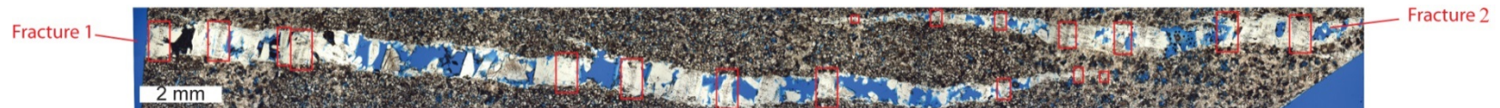
Figure B. 1: Petrographic image of SFOT-1-1,108.3'. Fracture 1 (bottom left) contains remnant tips of previously isolated fractures; fracture visual porosity (blue) is estimated to be 30%. Fracture 2 (top right) is in close proximity to the tip of fracture 1; fracture visual porosity is around 23%. The dominant type of cement is quartz and small amounts of ankerite. Labeled quartz bridges (B#) were imaged using SEM-Cl.
