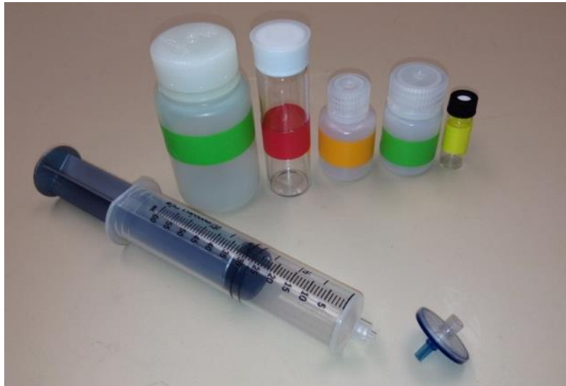
Figure 9: Chemical sampling bottles. Left to right: Raw sample, carbon, cations, anions, and stable isotopes.
