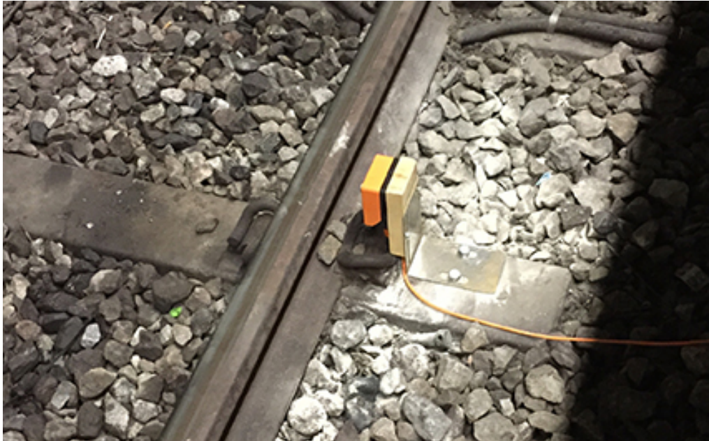
Figure 26. The position of the inductive sensor
