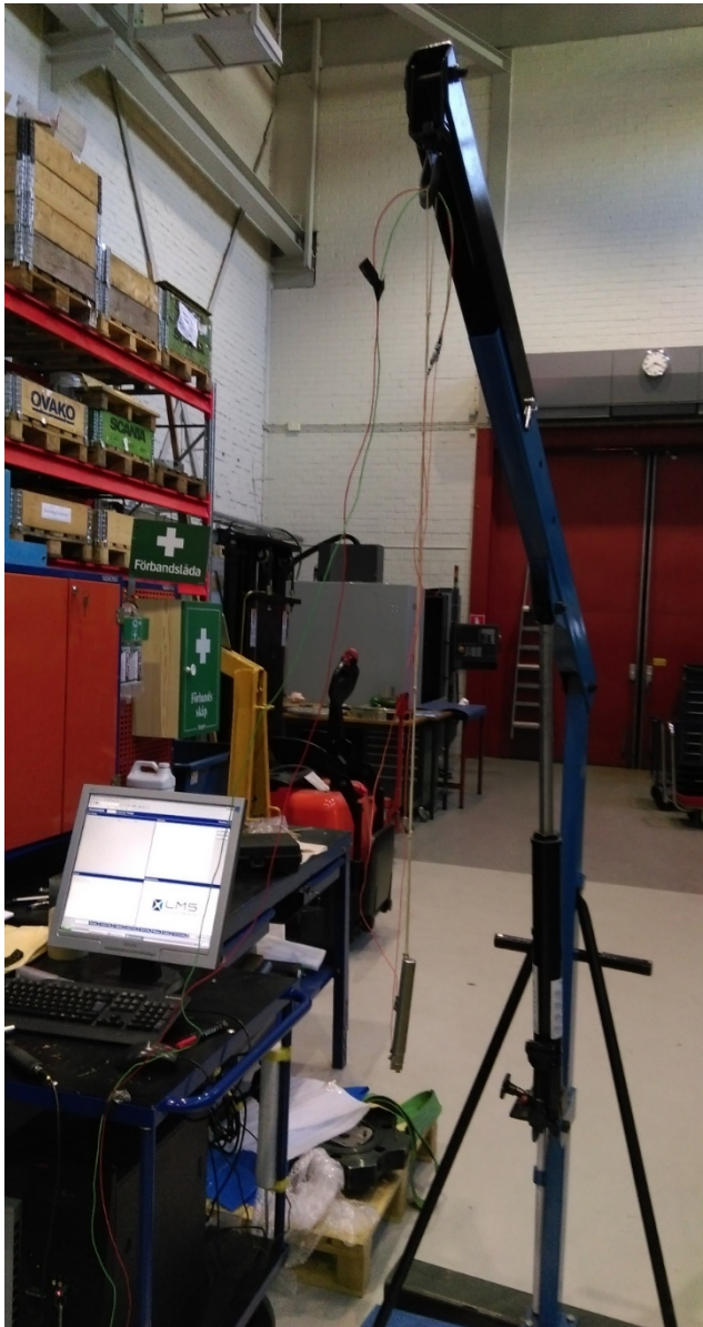
Figure 3.5: The experimental set up of free hanging test. The sensors are attached to the cutting tool with the help of wax and the setup is connected to the LMS test lab unit.
