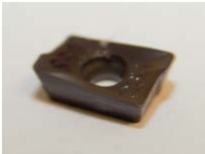
Figure 3.9: Insert used-ISCAR HM90 APKT 1003PDR IC 950.
