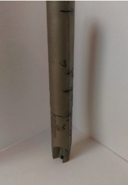
Figure 3.3: Cutting tool made of Bohler-Uddeholm H13.
