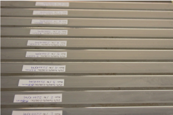
Figure 3.8: Each slot is machined at different RPM and depth of cut ( A_p ).
