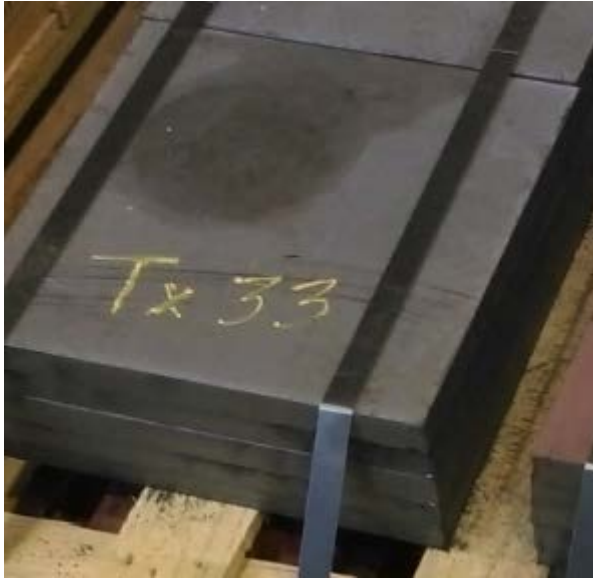
Figure3.1: (left) Toolox 33 plates (Workpiece/Dimension: 20x300x300 mm); (Right) Toolox 44 cutting tool.
