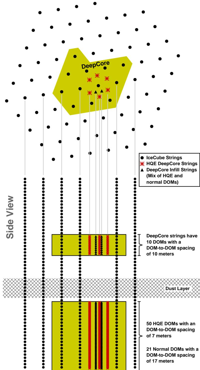
**Figure 19:** Top down and side-view diagram of DeepCore. The side-view shows the difference in DOM distribution for the infill strings and their relation to the dust layer [5].
