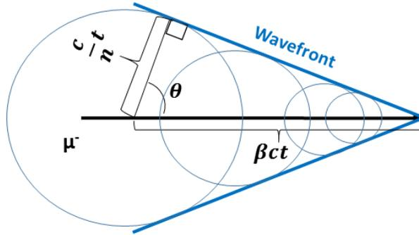
**Figure 5:** Diagram of a Cherenkov light cone produced by a muon traveling at speed  $v = \beta c$  through a transparent medium with index of refraction  $n$ . The blue circles show points of light emission along the particle track. Since the muon travels faster than light in this medium, the light emission forms a shock-front analogous to a sonic boom.
