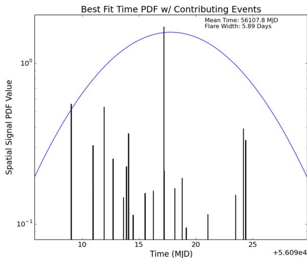
**Figure 49:** Plot above shows the signal spatial p.d.f. values for several of the most signal-like events for the best fit flare. The y-axis denotes the value of the spatial p.d.f. while the x-axis gives the time of arrival for the event in MJD. The blue Gaussian is the time profile for the best fit flare found by the method.
