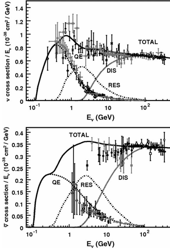
**Figure 1:** Total inclusive cross-section is plotted above as a function of energy along with individual cross-sections for different interaction channels. Above a few tens of GeV, it is clear that deep inelastic scattering begins to dominate [40].
