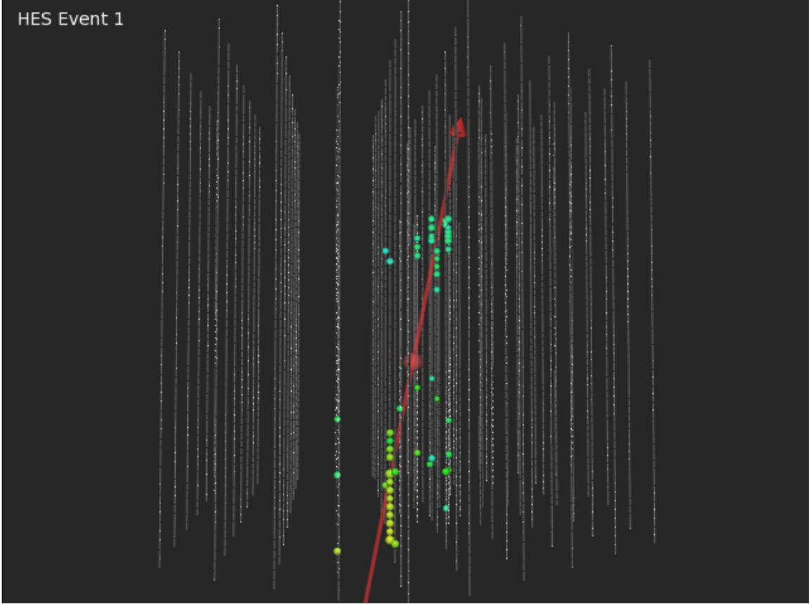
**Figure 33:** Event display for a final level neutrino track event with reconstructed track. This event is fairly energetic with respect to the usual events in the final sample. The red arrow shows the best fit from the 16-iteration SplineMPE reconstruction. The dust layer is clearly visible by the lack of DOMs registering light in the middle of the event track.
