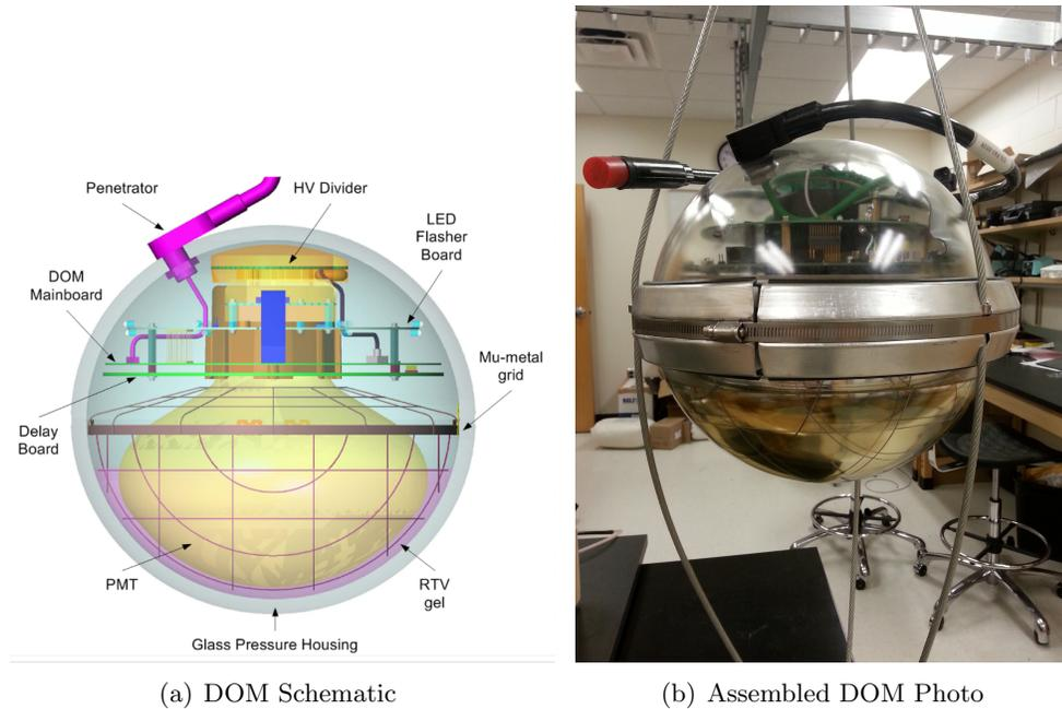
**Figure 22:** (a) Schematic detailing DOM structure [10]. (b) A fully assembled DOM supported by a cable harness.
