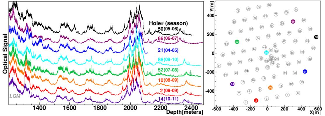
**Figure 18:** Borehole laser measurements of dust concentrations in the ice as a function of depth. Measurements for several IceCube strings are displayed. Higher values on the y-axis denote higher dust concentrations. The "dust layer" features quite prominently at a depth of 2100m [61].
