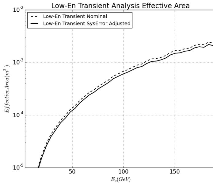
**Figure 42:** Effective area at final event level as a function of energy. The black line gives the analysis effective area after adjustment for systematic error while the nominal effective area is plotted as the dashed line.
