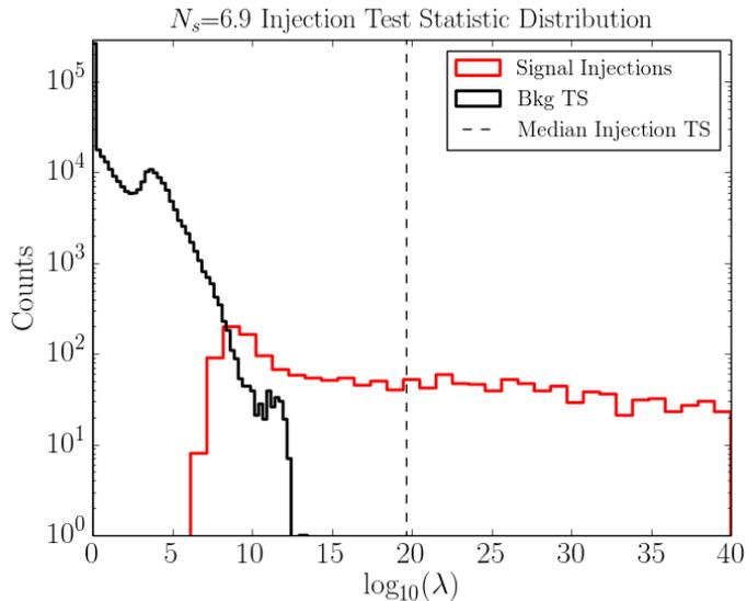
**Figure 54:** Test statistic distribution for signal injections (red) and background trials in the same declination band. The bi-modal shape of the background test statistic distribution arises from the inclusion of test statistic values returned by both the coarse and fine sky scans. The second background distribution does not begin at zero because the fine scan follow up is only performed for best fit flares that reach a certain test statistic threshold
