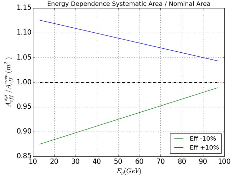
**Figure 41:** Ratio of systematic set effective areas to the nominal effective area. The plot above shows that the degree to which the analysis is affected by DOM efficiency is clearly energy dependent.
