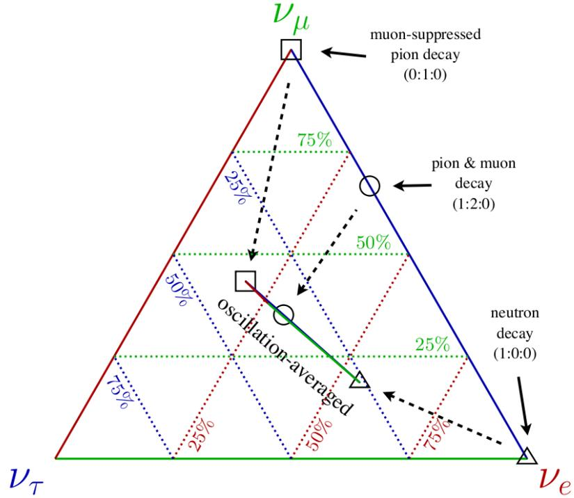
**Figure 6:** Neutrino flavor ratio space. Oscillation over astronomical baselines will result in a flavor ratio at Earth different than at source. If the flavor ratio for a given source can be measured it can help identify the process through which that source’s neutrinos were produced [65].
