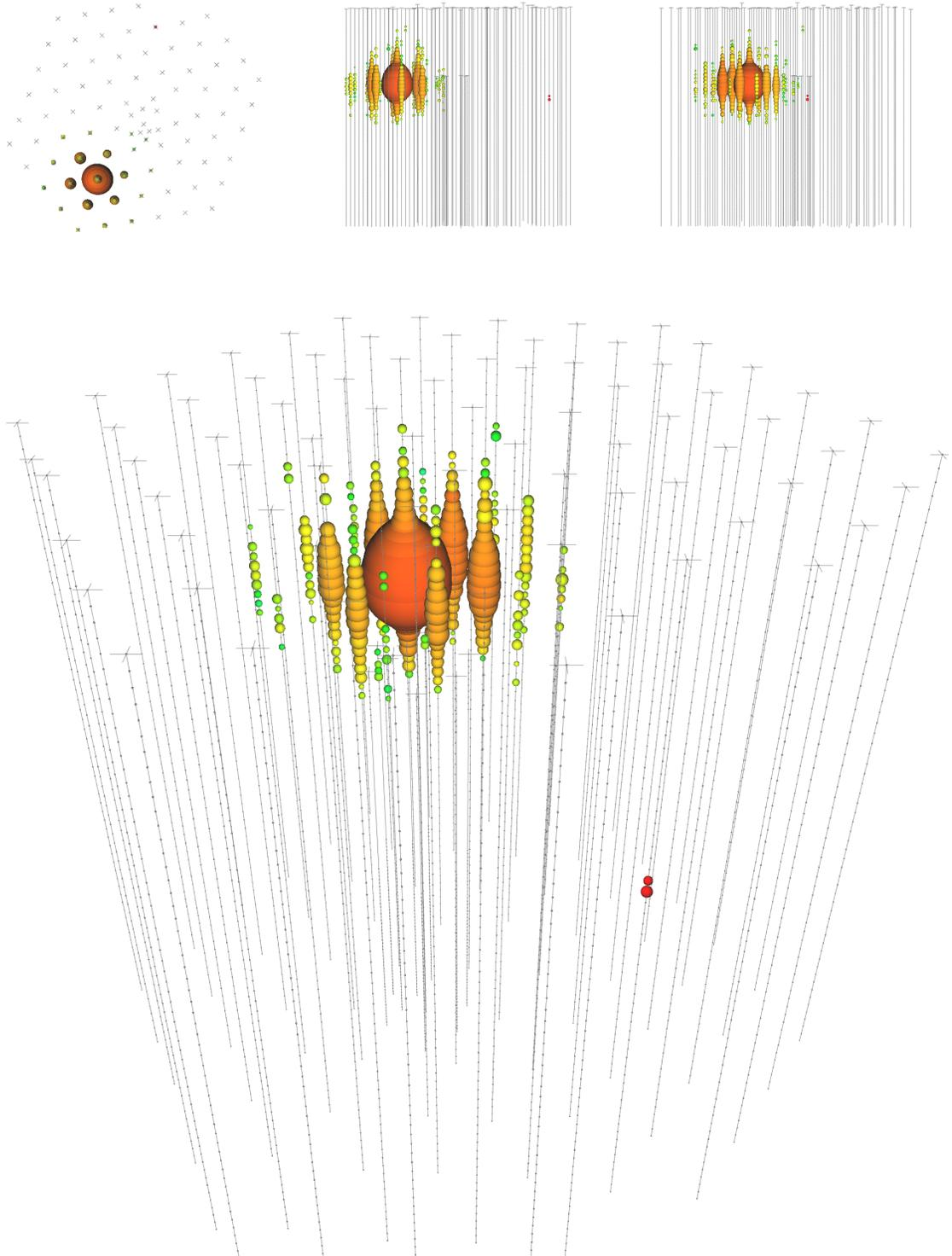
**Figure 20:** A high-energy cascade event in IceCube with deposited energy of  $210 \pm_{25.8}^{29.0}$  TeV [58]. The colored spheres represent DOMs that have registered light during the event. The size of the spheres are indicative of the total light received by the PMT on that DOM. The color denotes the timing of the hit with red corresponding to earlier times and blue corresponding to later times.
