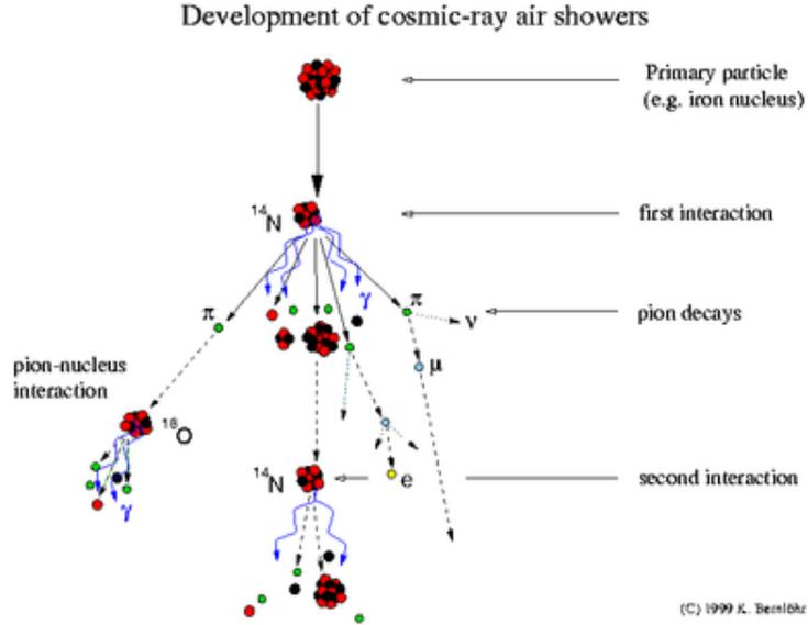
**Figure 8:** Schematic diagram of a iron nuclei cosmic ray interacting with a target nitrogen atom in the atmosphere. The development of the shower is demonstrated by the illustration of secondary interactions caused by daughter particles of the initial interaction [56].
