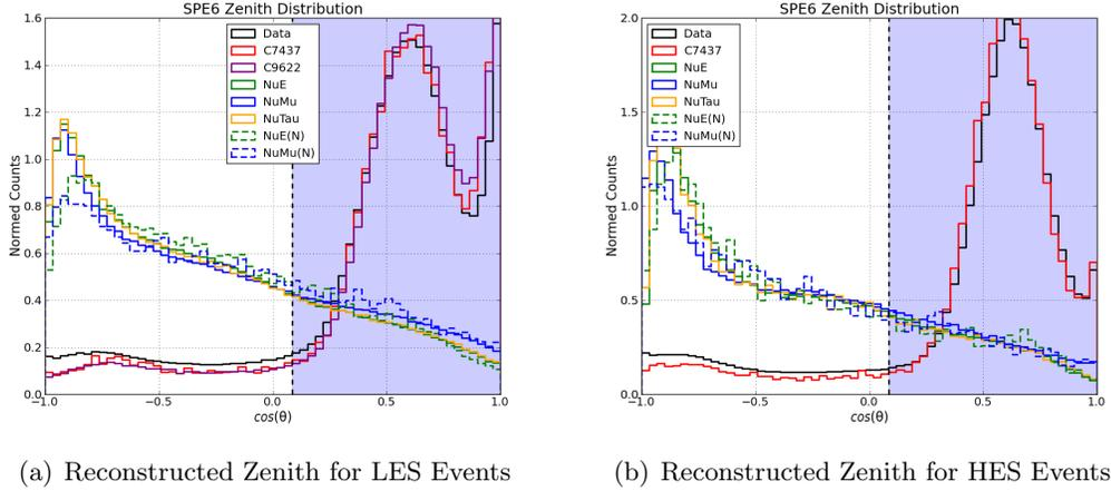
**Figure 27:** Normalized distributions of reconstructed zenith from an 6-iteration SPE fit to nominal DOM hit map. The distributions for LES (a) and HES (b) events show that the bulk of the data at this level consists of downgoing muons. The cut region is given by the shaded areas in the plots above.
