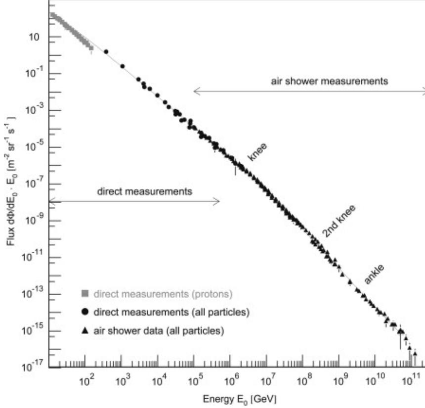
**Figure 7:** Cosmic ray energy spectrum at Earth as measured by several experiments [31]. The spectrum is relatively featureless over several orders of magnitude. There is an observed slight flattening of the spectrum at about  $10^{18}$  eV. This feature is dubbed the ‘ankle’ and is widely considered to signal a transition between a galactic and extra-galactic component of the cosmic ray spectrum [18].
