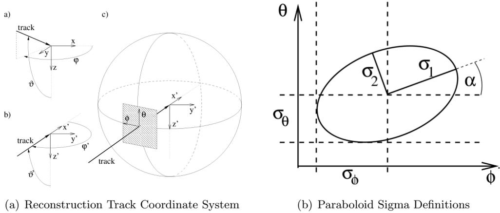
**Figure 34:** (a) The coordinate system for muon tracks in reconstruction algorithms. (b) Definition of the paraboloid sigmas derived from the reconstruction likelihood space. Width of the major and minor axes of the potential well are given by  $\sigma_{1,2}$  while  $\sigma_{\theta,\phi}$  give the width of the likelihood space in reconstruction directional coordinates [76].
