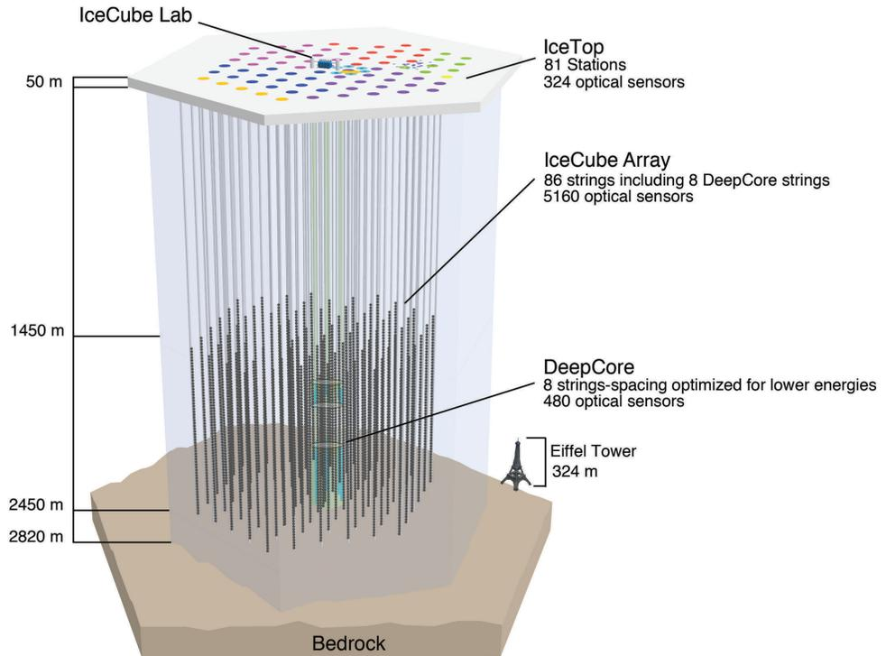
**Figure 17:** Diagram of the IceCube Neutrino Observatory (Courtesy of the IceCube Collaboration).
