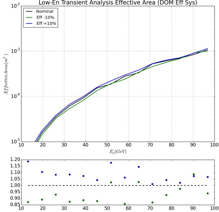
**Figure 40:** Effective area at final event level as a function of energy for different possible DOM efficiency settings. At lower energies, the change in effective area becomes approximately proportional to the relative change in DOM efficiency. The subplot below the effective area shows the bin-by-bin ratio of the systematic effective area to that of the nominal effective area.
