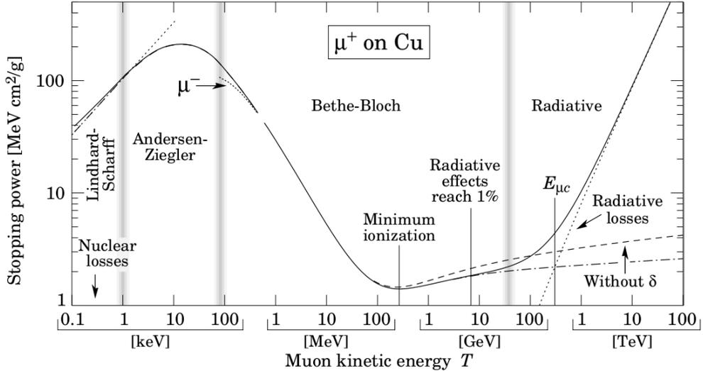
**Figure 4:** Total stopping power (solid line) of muons in copper as a function of kinetic energy. Contributions from individual processes are shown as well as the energy ranges in which these processes are most dominant. [48].
