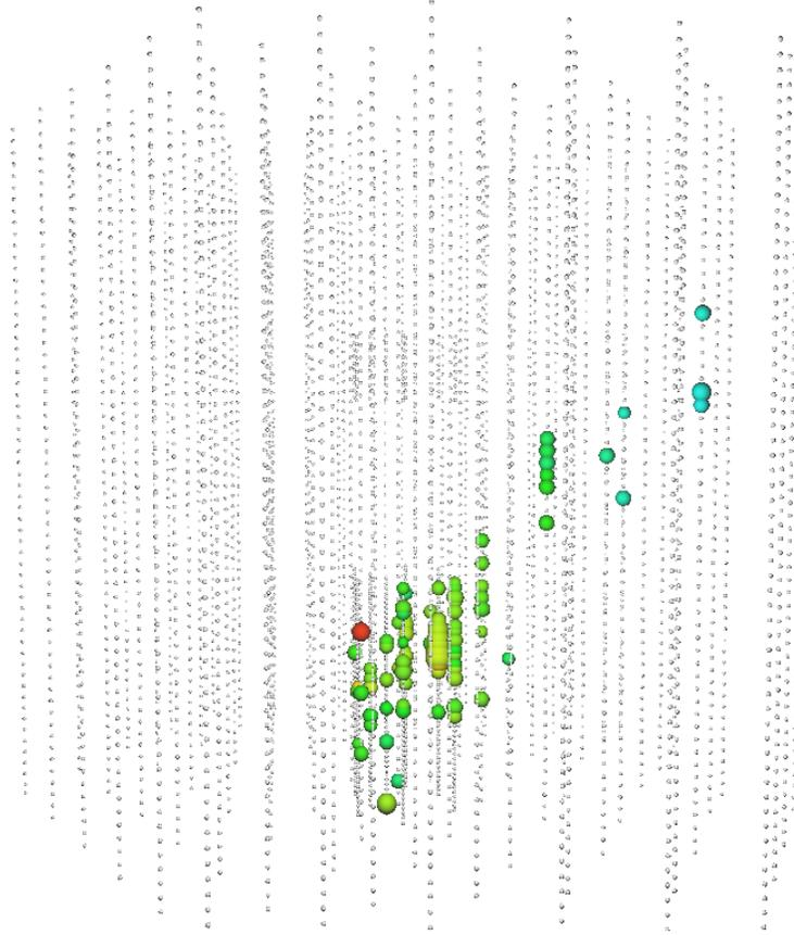
**Figure 38:** Event display for a final level neutrino track event originating in DeepCore. The colored spheres represent DOMs that have registered a hit during the event. The size of the spheres are indicative of the total light received by the PMT on that DOM. The color denotes the timing of the hit with red corresponding to earlier times and blue corresponding to later times.
