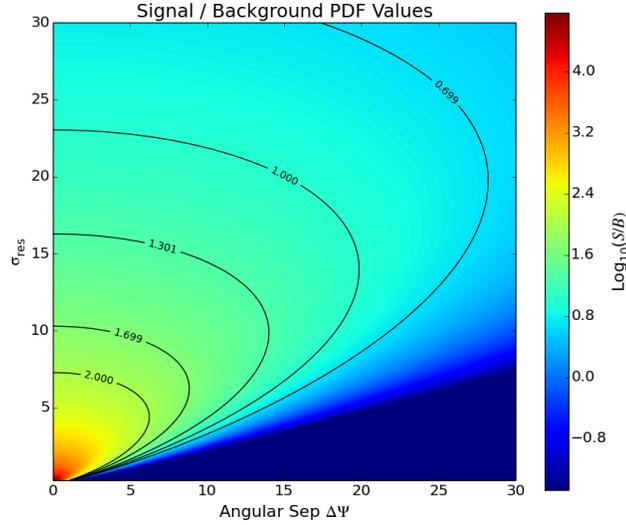
**Figure 30:** Contour plot showing the ratio of the signal and background p.d.f. values for different choices of event-source separation ( $\Delta\Psi$ ) and event resolution ( $\sigma_{res}$ ). Parameter choices that lie within the contours have a signal-to-background ratio large enough to be included in the analysis should that contour value of  $S/B$  be chosen as the threshold.
