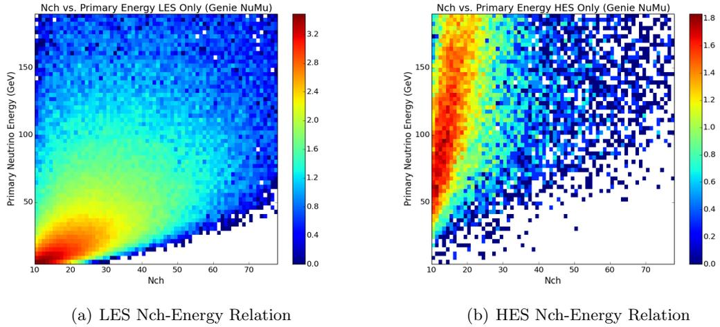
**Figure 63:** NCh-Energy relation for simulated  $\nu_\mu$  neutrino events at the final level. Nch is a shorthand term for the number of DOMs receiving light from an event. Subfigure (a) shows the correlation for events belonging to the Low-Energy Stream (LES) branch of the event selection while (b) shows the same for events belonging to the High-Energy Stream or HES branch.
