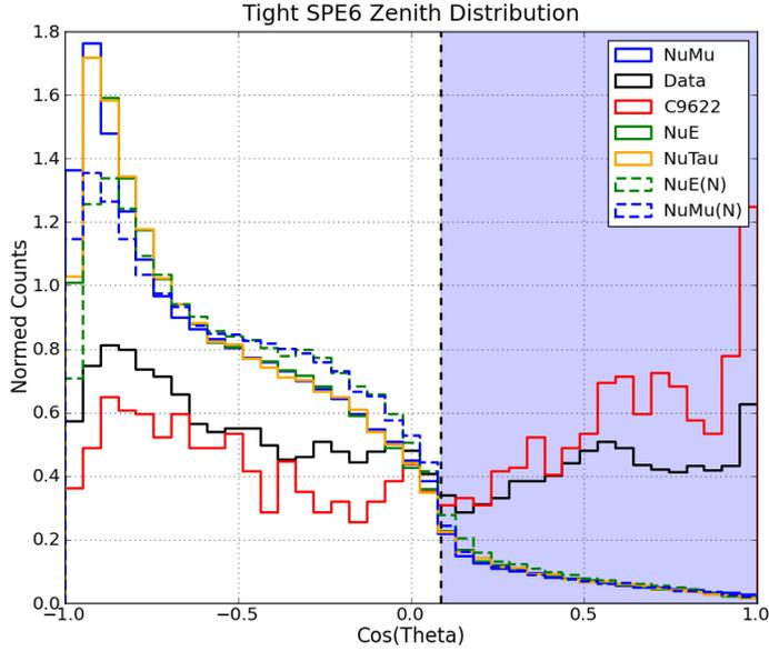
**Figure 60:** Distribution of reconstructed  $\text{Cos}(\Theta_{zen})$  for simulation and data. The Tight-SPE6 reconstruction is applied on the LES branch of the dataset. The SeededRT cleaning used to generate the hit map over which the reconstruction is applied has tighter settings for radius and time ( $R = 75$  m [150 m nominal],  $T = 625$  ns [1000 ns nominal]). The shaded area denotes the cut region.
