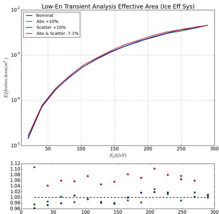
**Figure 39:** Effective area at final event level as a function of energy for different possible ice properties. Increased absorption and scattering lead to very little degradation of the neutrino effective area at even the lowest energies. The subplot below the effective area shows the bin-by-bin ratio of the systematic effective area to that of the nominal effective area.
