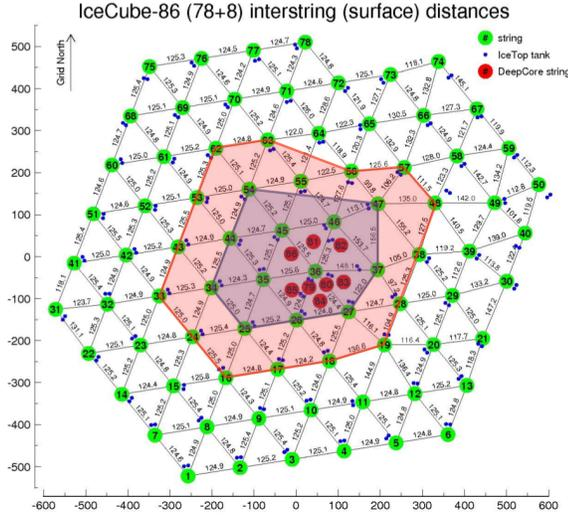
**Figure 25:** String location plot detailing the boundaries of the standard (blue shaded region) and expanded (orange shaded region) DeepCore volumes. DOMs belonging to strings inside the boundary and whose vertical position in the detector lies below the dust layer are considered to be inside the fiducial volume.
