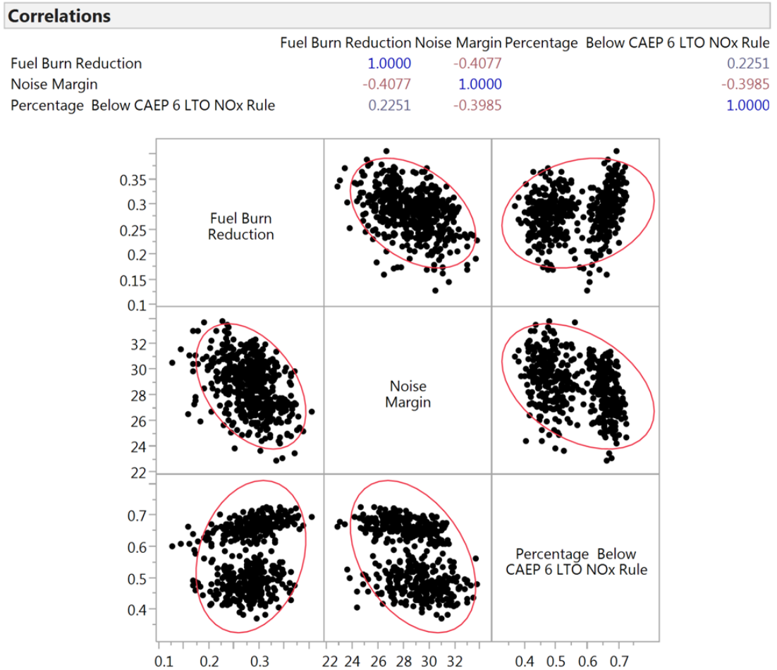
Figure 43: Analysis of correlation between fuel burn reduction, noise margin, and NOx emissions for LTA vehicle.
